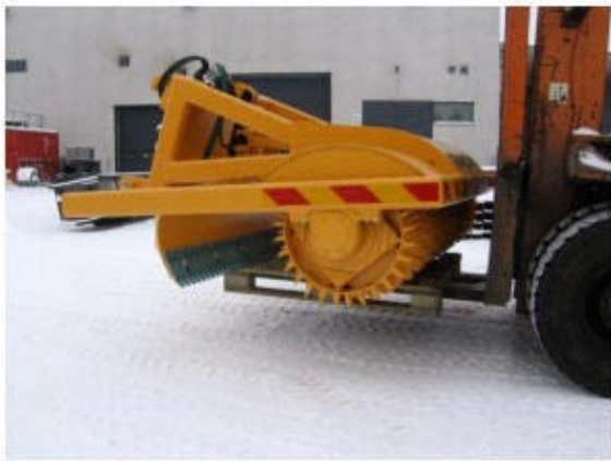
Fig 6. Raiko Wheel Loader Attachment with Plow
