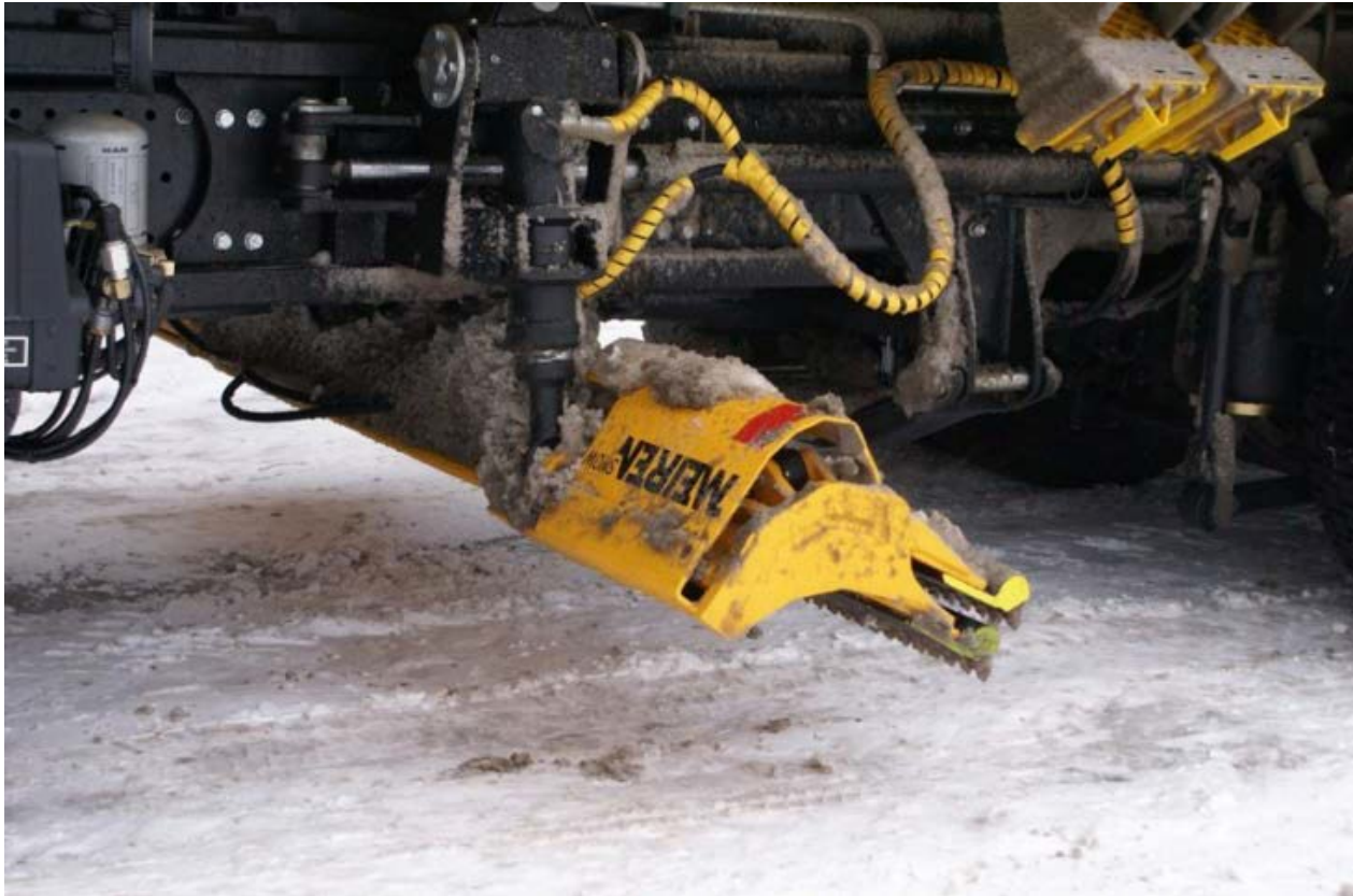
Fig 5. Underbody scraper (courtesy Meiren Engineering)
