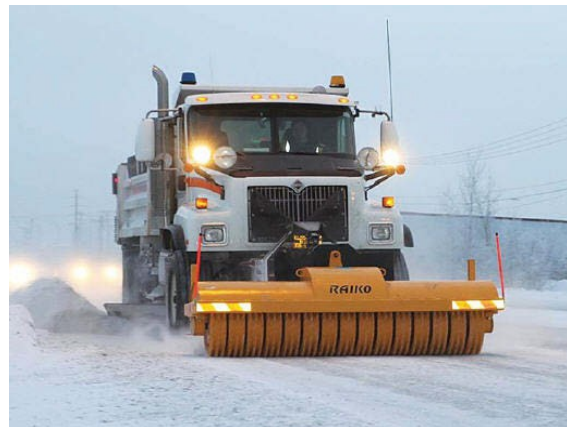
Fig 7. Underbody Plow Truck with a Raiko Attachment in Operation (Alaska DOT)
