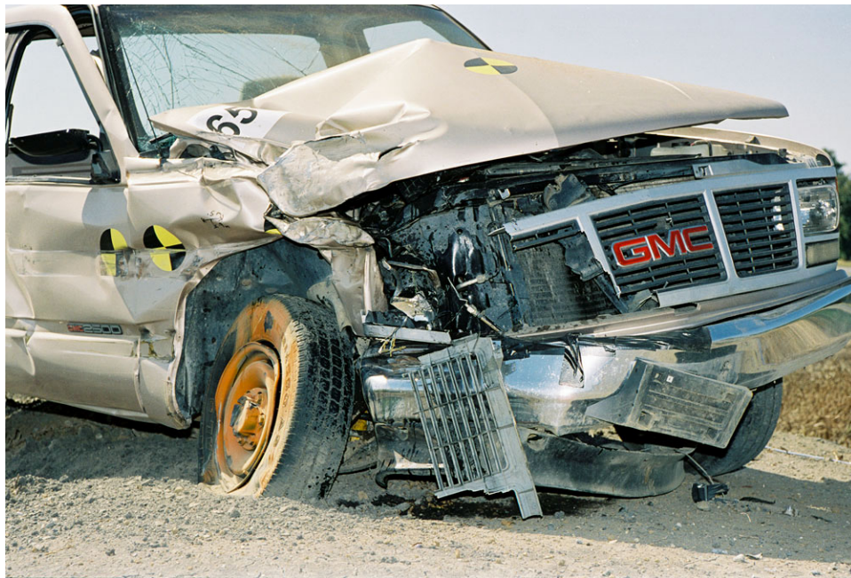
Figure 2-19 - Test 651 Vehicle Damage, Front Right Corner
