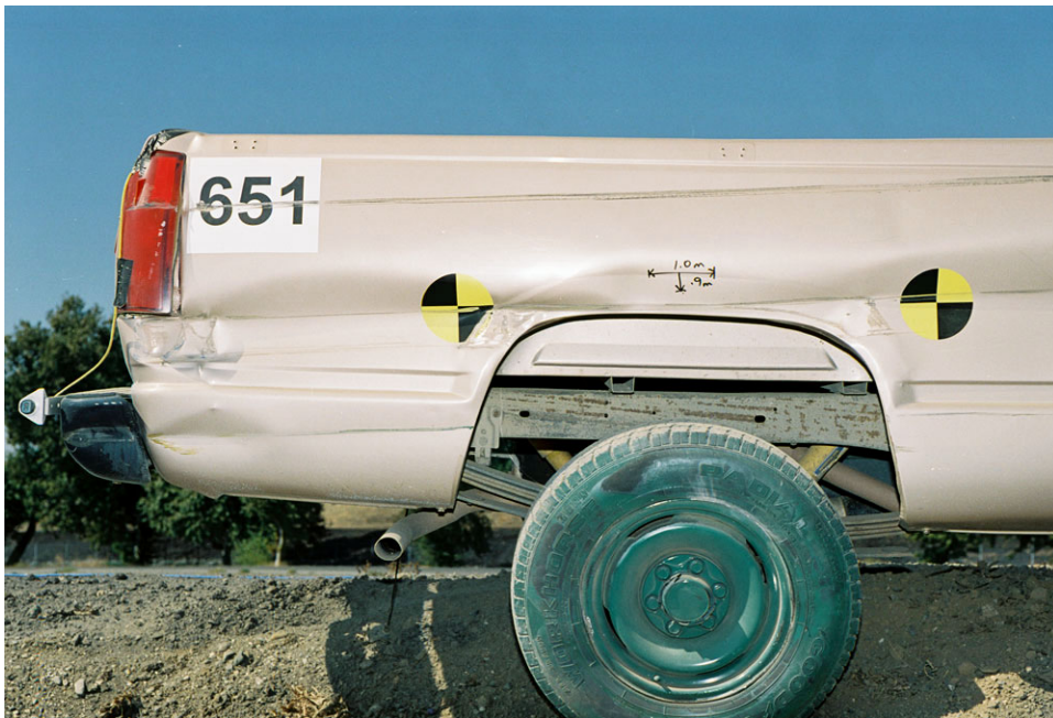
Figure 2-21 - Test 651 Vehicle Damage, Right Side of Truck Bed
