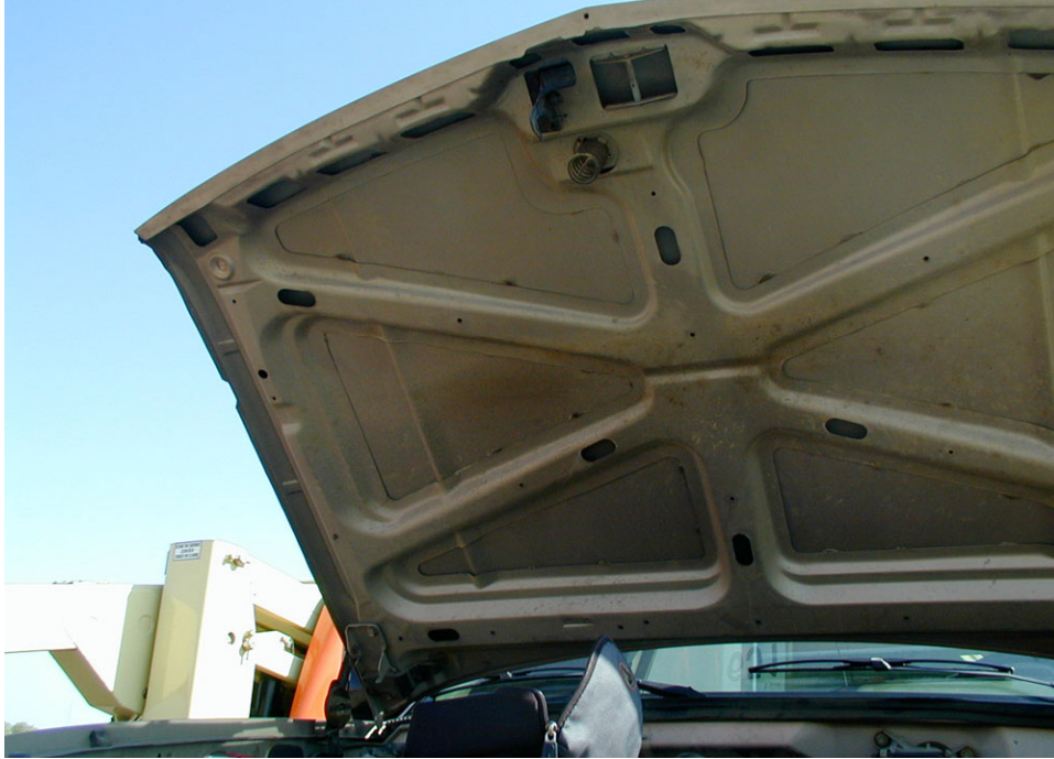
Figure 2-12 - Test Vehicle 651, Underside of the Hood
