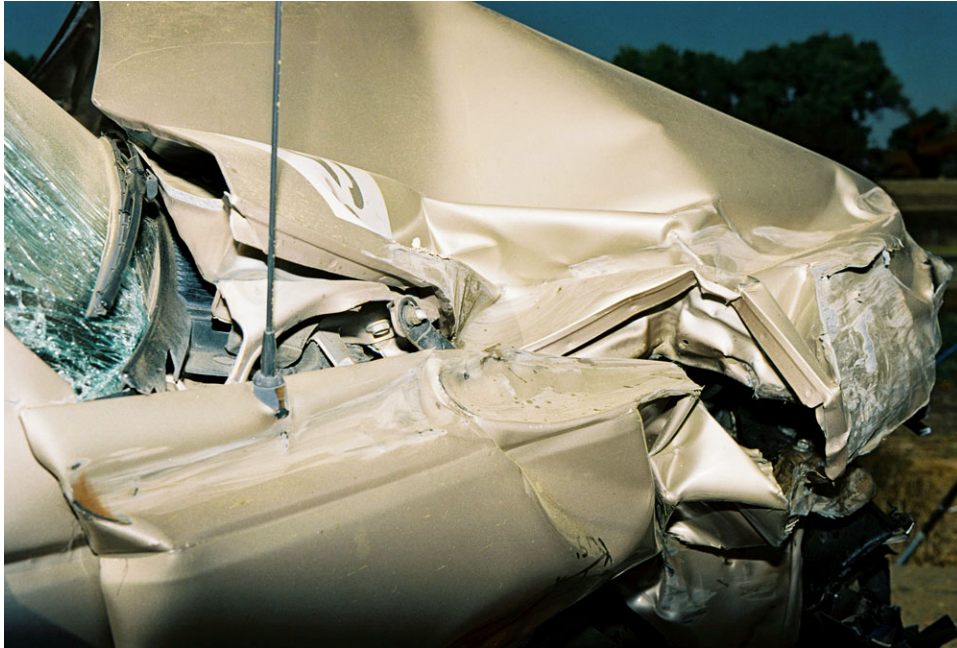
Figure 2-20 - Test 651 Vehicle Damage, Hood and Windshield
