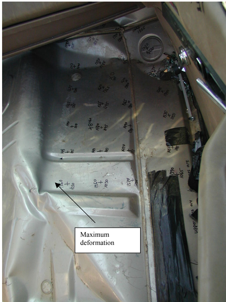
Figure 2-22 - Test 651 Vehicle Damage, Floor Deformation
