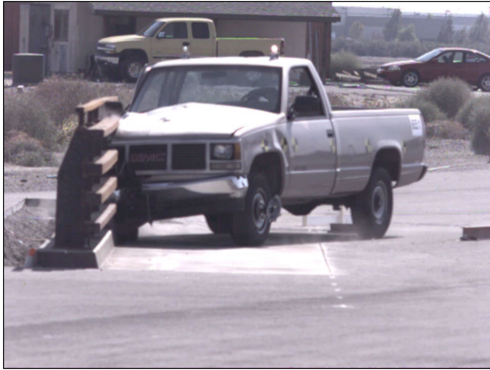
Figure 2-15 - Test 651 Hood Buckling, 66 ms After Impact
