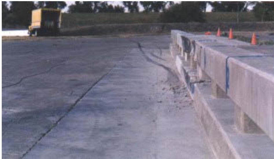
Figure 2-40 Barrier and Resting Point of Vehicle
