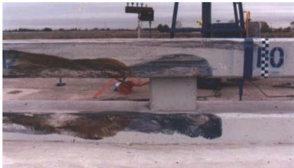
Figure 2-31 Test 545 Impact Area
