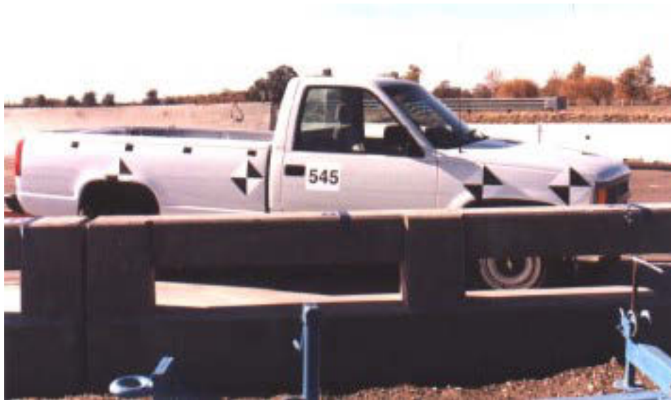
Figure 2-24 Vehicle and Bridge Rail before Test 545
