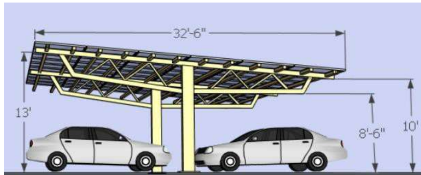
Figure F.1: A solar canopy design showing approximate dimensions of the structure (Structural Solar, 2013).
