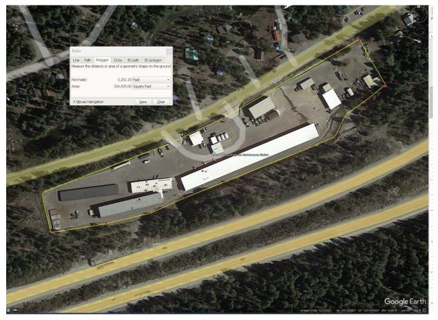
Figure 6.1: Kingvale yard outlined by a yellow line. The estimated perimeter is 3,251 feet. The estimated area is 324,435 square feet including buildings. Image courtesy of Google Earth.
