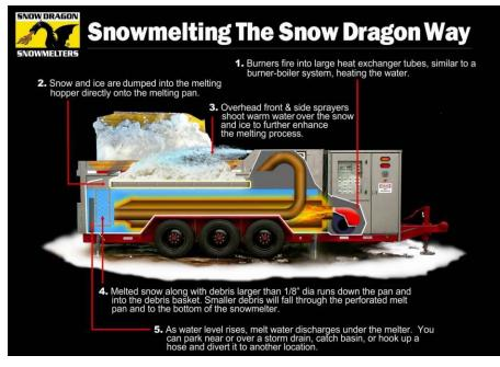
Figure 2.3: How the Snow Dragon works. Image courtesy of the Snow Dragon manufacturer.
