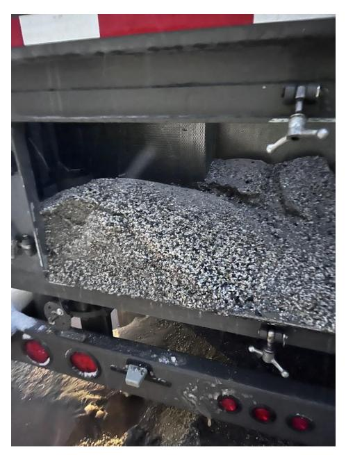
Figure 5.6: The bottom of the Snow Dragon and its condition after melting snow with less sand for 205 minutes
