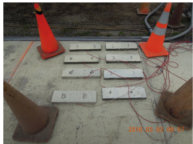
Prisms after demolding
