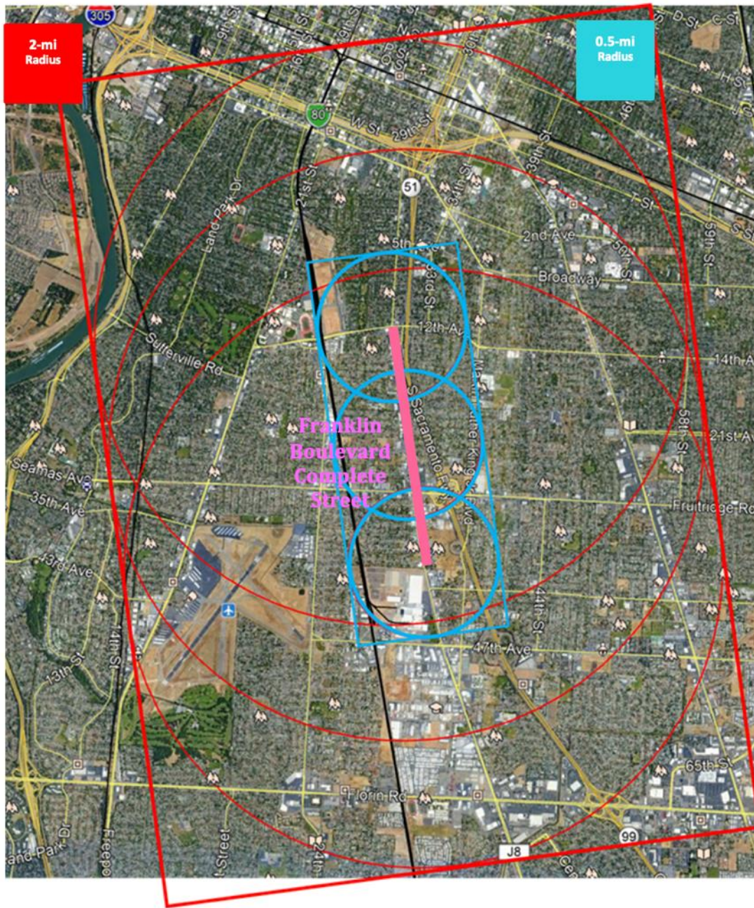
Figure 20. Access to Destination Buffer Area for Walking and Cycling Modes of Transportation, Franklin Boulevard Complete Street Project
