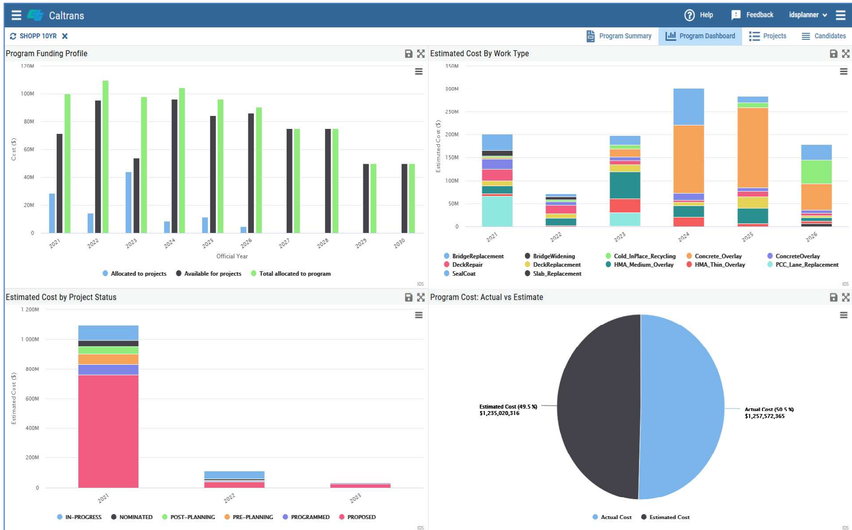
Figure 34: Example summary program status showing annual allocated funds, estimated costs, and actual expenditures.
