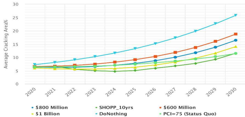
AVERAGE CRACKING AREA% UNDER DIFFERENT SCENARIOS
