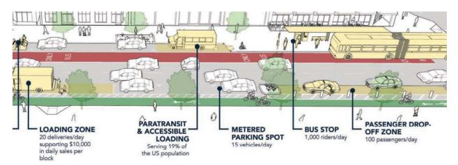
Figure 4. Examples of Various Flex Zone Uses (Roe and Toocheck, 2017)
