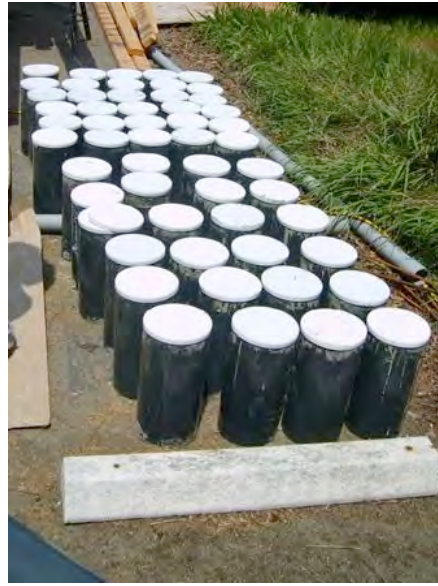
(b) After casting concrete cylinders
