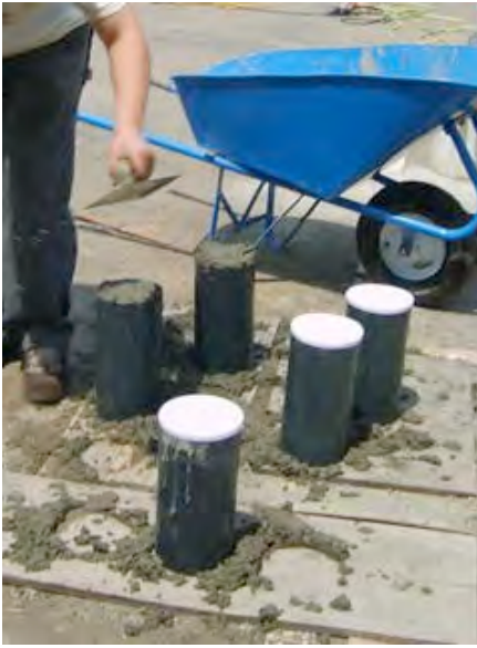
(a) Casting concrete cylinders
