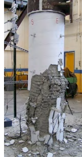
(b) Axial failure of the column
