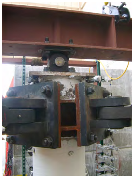
Fig. C.9 Attachment of actuators to column.
