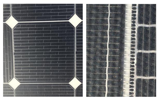
Figure 6.8. Photo of silicon cell with unusual grid pattern (left); enlarged image showing the interconnection of two cells (right).
