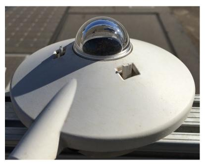
**Figure 2.1. Example of pyranometer.** The glass dome allows light to strike the black thermopile from any angle.
