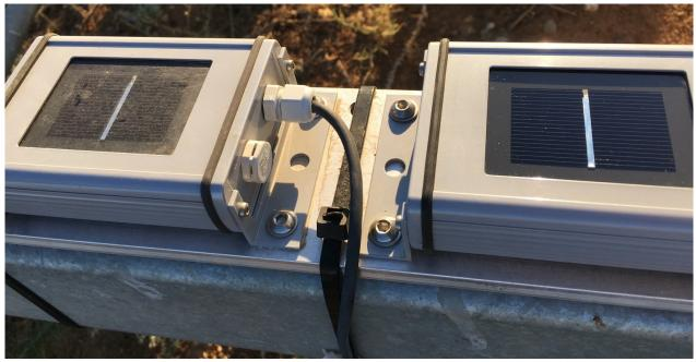
Figure 2.16. Sensors used to measure soiling.
