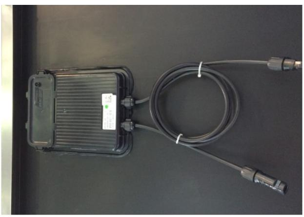
Figure 6.25. Example of "smart" module with electronics in junction box.
