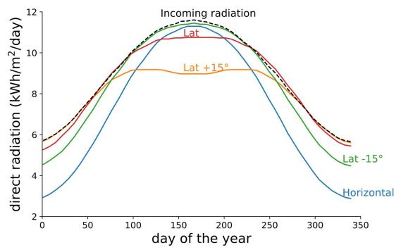
**Figure 6.16. Simulation of daily insolation.** Simulation of the daily insolation over a whole year for surfaces tilted toward the south by the latitude (37 degrees), latitude plus 15 degrees (aimed more to the south to better catch the winter sun), and latitude minus 15 degrees (closer to horizontal to better catch the summer sun).
