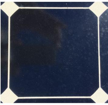
Figure 6.9. Image of cell in SunPower Module with no front grid pattern.
