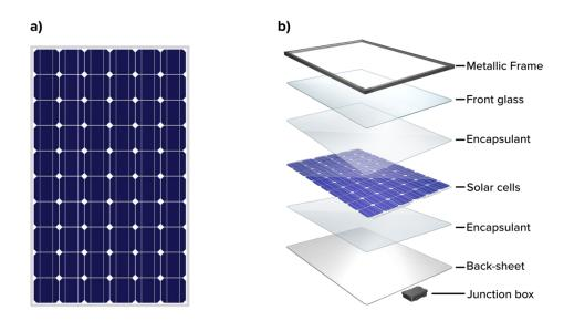
Figure 6.4. Silicon solar module structure: (a) silicon solar module, and (b) schematic diagram of the components of the solar module. Figure source: https://www.dupont.com/products/what-makes-up-a-solar-panel.html.
