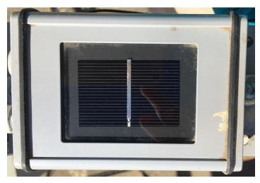
Figure 2.2. Silicon reference cell.
