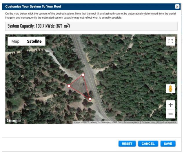
Figure 7.8. Estimation of siting of 130-kW system for Case 1.
