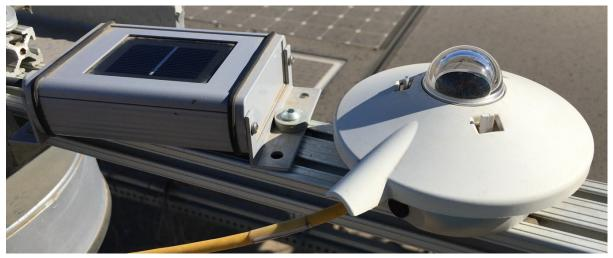
Figure 2.15. Example of reference cell and pyranometer mounted in same plane.
