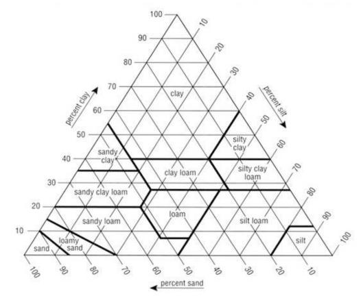
Fig. 3.3 Soil triangle used to classify soil texture
