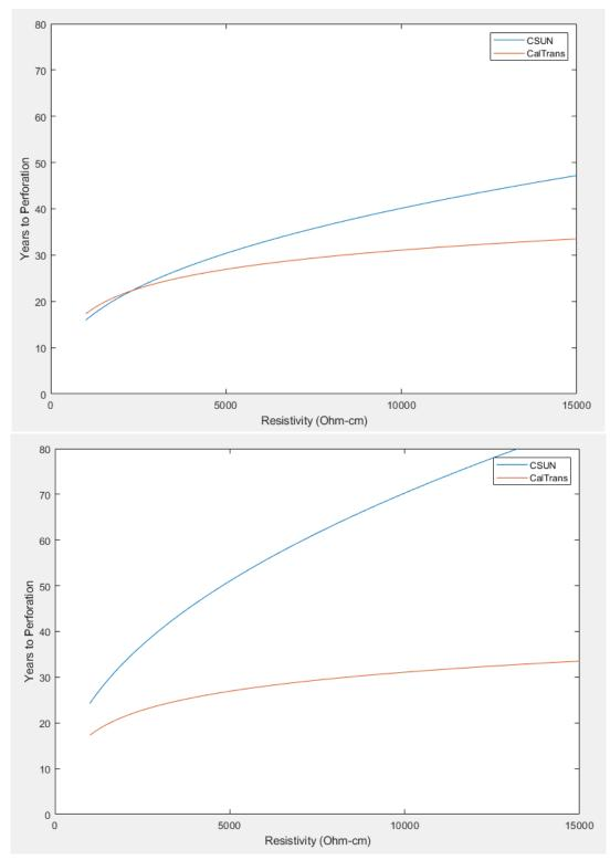
Fig. 6.9 Years vs. resistivity with a constant pH of 7 at 15% failure criteria (top) and 25% failure criteria (bottom)\*
