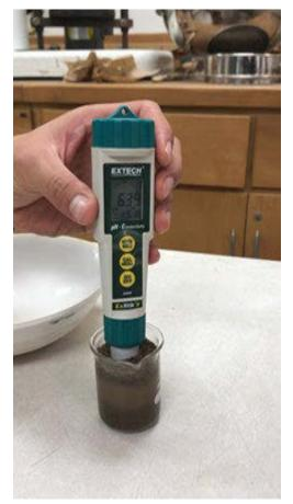
Fig. 4.2 ExStik II reading soil data
