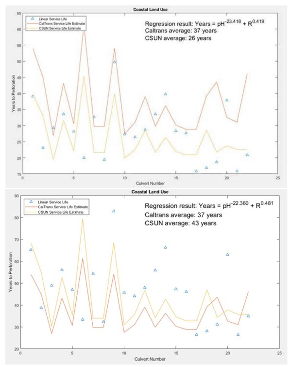
Fig. 6.4 Comparison of Caltrans and CSUN service life equations for Coastal regions at 15% failure criteria (top) and 25% failure criteria (bottom) \*
