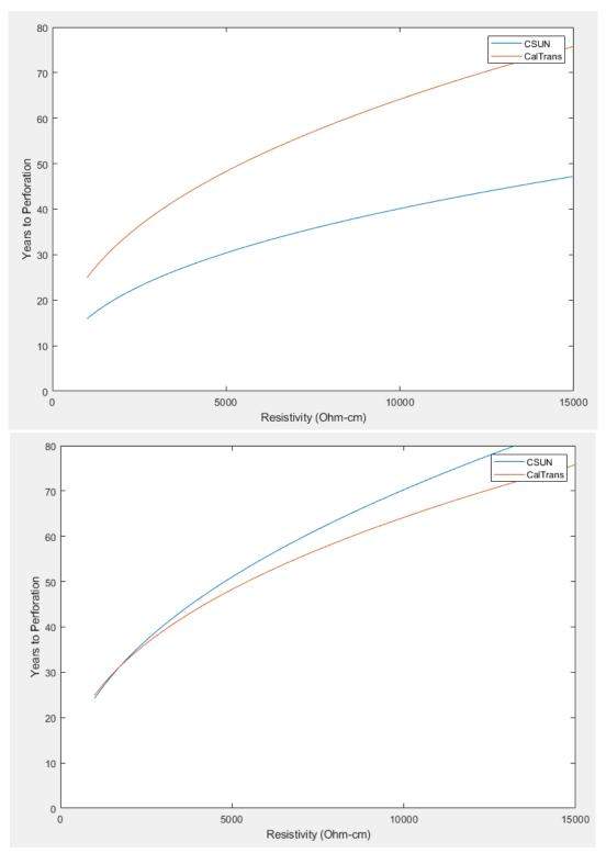
Fig. 6.8 Years vs. Resistivity with a constant pH of 7.5 at 15% failure criteria (top) and 25% failure criteria (bottom) \*
