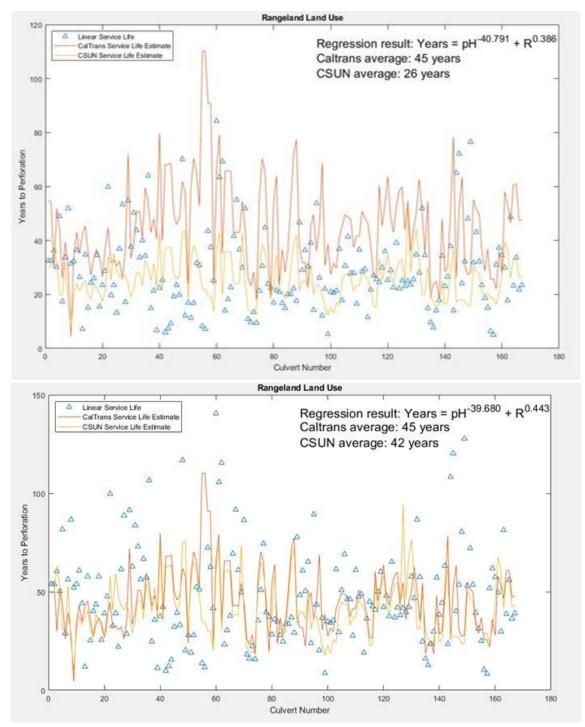
Fig. 6.6 Comparison of Caltrans and CSUN service life equations for Rangeland regions at 15% failure criteria (top) and 25% failure criteria (bottom) \*
