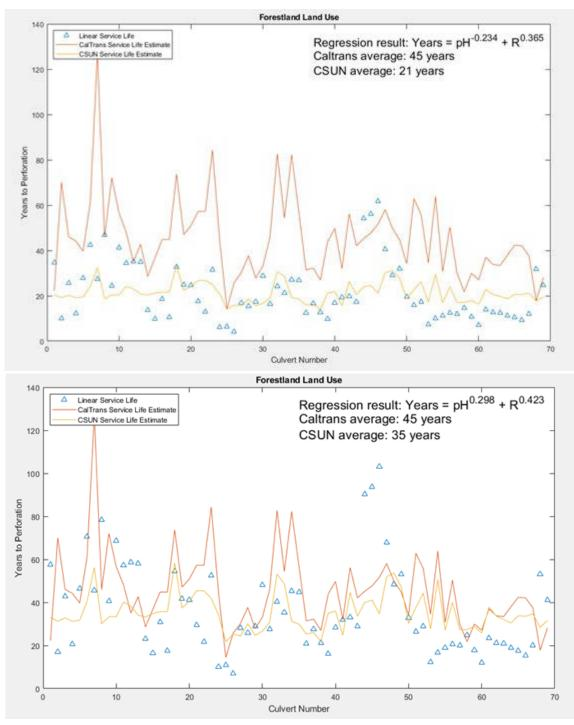
Fig. 6.5 Comparison of Caltrans and CSUN service life equations for Forestland regions at 15% failure criteria (top) and 25% failure criteria (bottom) \*
