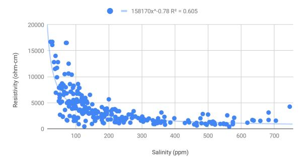
Fig. 4.5 Plot of salinity vs. resistivity
