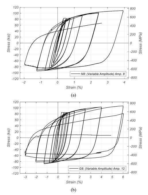
Figure 5.14. Hysteretic Response of: (a) Normal; (b) Smoothed-Rib-Radii Test Bars to Loading Protocol SH1
