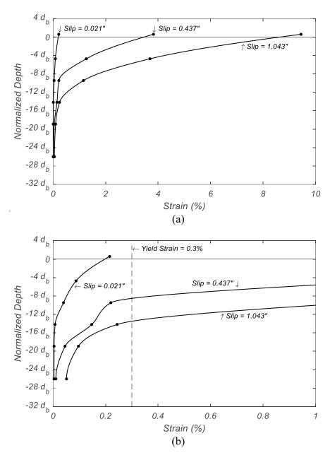
Figure 2.19. Strain Profile of Test Bar in Specimen #2: (a) Overall; (b) Closeup View Displaying Yield Penetration
