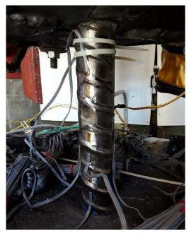
Figure 5.12. Electrical-Foil Strain Gages Applied to Test Bar
