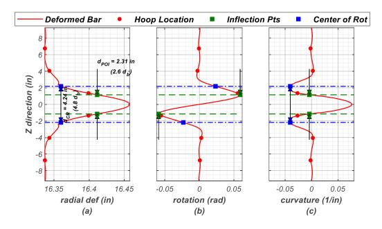
Figure 5.27. Deformed Shape of Buckled Reinforcement, Case 28: (a) Lateral Deformation; (b) Node Rotations; (c) Curvature Distribution
