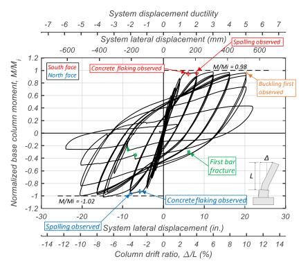
Figure 3.17. Normalized Base Column Moment-Displacement Response of Test Specimen Identifying Key Points During Testing
