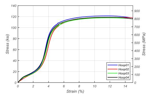
Figure 4.9. Butt-Welded Column Hoop Validation Tensile Tests
