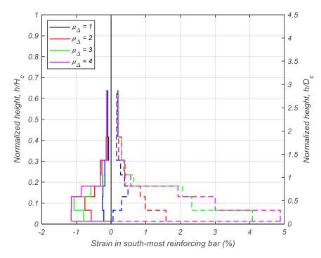
Figure 3.27. Smeared Strain Profile of Southern-Most Column Reinforcing Bar
