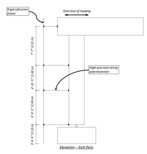
Figure 4.16. High-Precision String Potentiometers to Monitor Lateral Displacements
