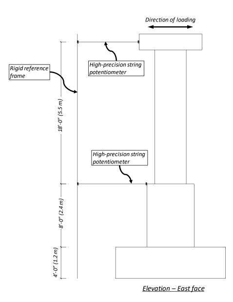
Figure 3.15. String Potentiometers Monitoring Lateral Displacements
