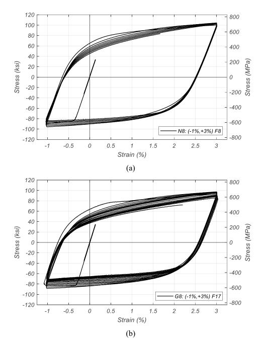
Figure 5.16. Hysteretic Response of: (a) Normal; (b) Smoothed-Rib-Radii Test Bars to Loading Protocol SH3
