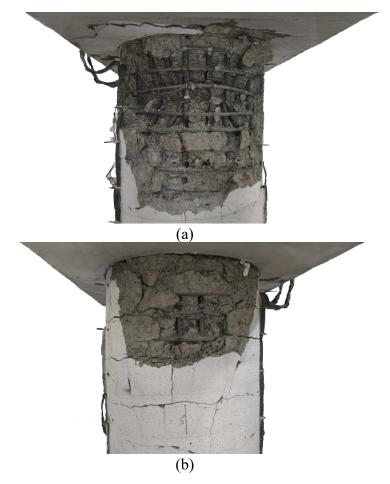
Figure 4.22. 360° Detailed 3D Point Cloud Model Showing Extent of Damage in Column Plastic Hinge Region Post-Test; (a) Interior Face of Column; (b) Exterior Face of Column
