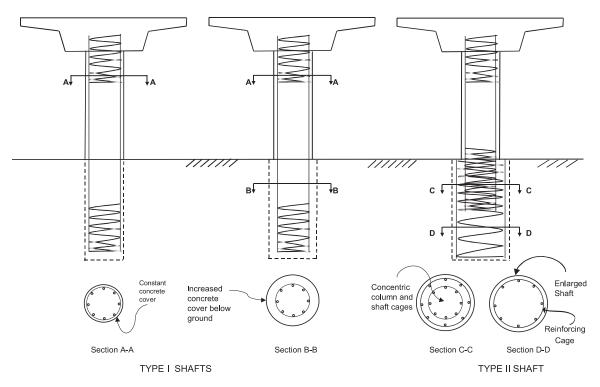
Figure 3.1. Columns Extending into Type I and Type II Pile Shafts (Caltrans SDC 2.0)
