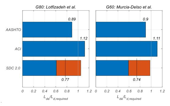
Figure 3.9. Comparison of Column Longitudinal Bar Embedment Length
