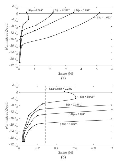
Figure 2.15. Strain Profile of Test Bar in Specimen #1: (a) Overall; (b) Closeup View Displaying Yield Penetration
