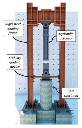
Figure 2.5. 3D Rendering of Test Setup
