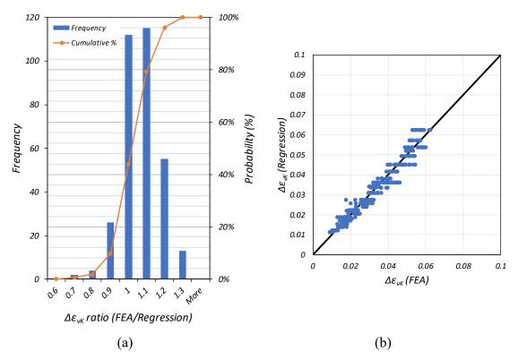
Figure 5.32. Regression Results for  $\Delta \varepsilon_{\nu K}$ : (a) Fragility Curve for Ratio Between Regression and FE Model Results; (b) Regression vs FE Model Results
