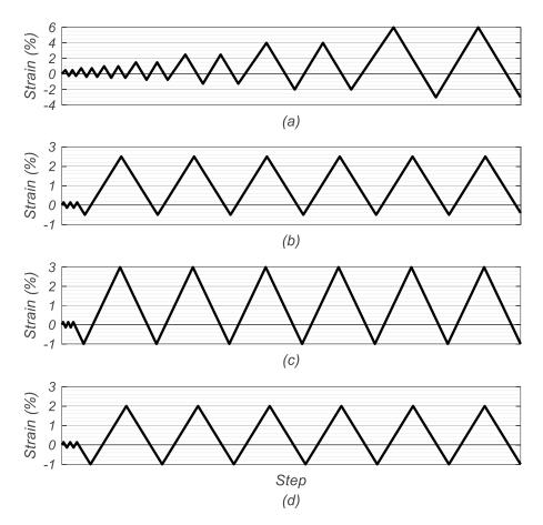
Figure 5.7. Loading Protocol Strain Histories: (a) SH1: Variable Amplitude; (b) SH2: (3%, -0.5%); (c) SH3: (4%, -1%); (d) SH4: (3%, -1%)
