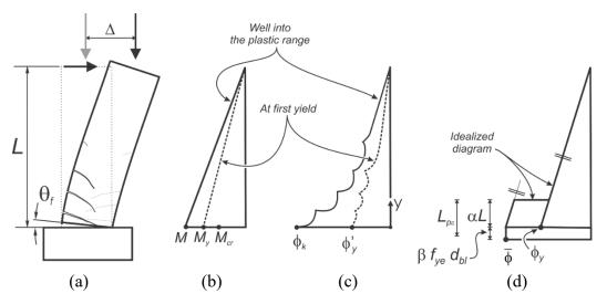
Figure 3.37. Smeared-Strain Compatible Method for Equivalent Plastic Hinge Length: (a) Deformed Column; (b) Bending Moment Diagram; (c) Curvature Diagram; (d) Idealized Curvature Diagram (Duck et al., 2018)
