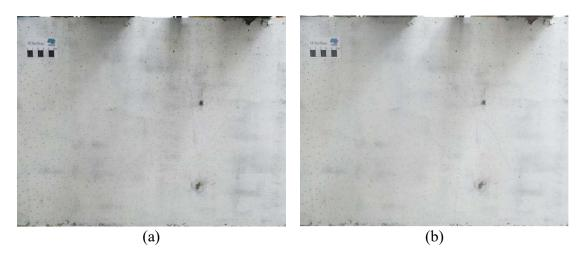
Figure 4.21. Minor Shear Cracking Observed in West Face of Bent Cap Joint at: (a) Peak of Displacement Ductility +4; (b) Peak of Displacement Ductility -4
