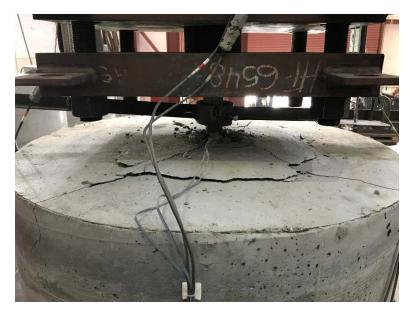
Figure 2.25. Damage Surface at Top of Column in Specimen #4
