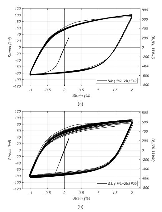
Figure 5.17. Hysteretic Response of: (a) Normal; (b) Smoothed-Rib-Radii Test Bars to Loading Protocol SH4
