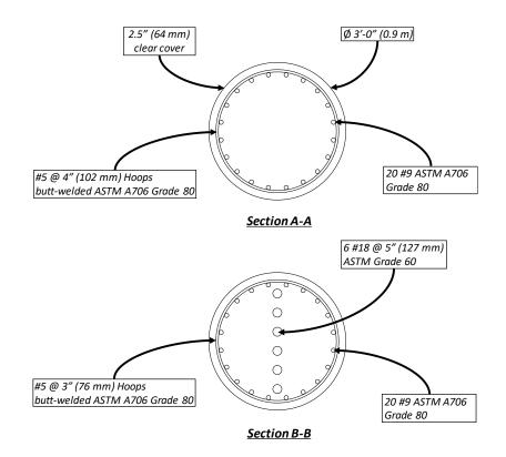
Figure 4.5. Reinforcement Configuration of Column
