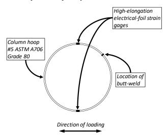
**Figure 4.13. Representative Column Hoop Instrumentation**
