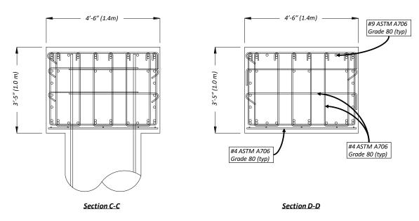
Figure 4.6. Reinforcement Configuration of Cap Beam
