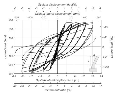
Figure 3.16. Global Lateral Load-Displacement Response of Test Specimen
