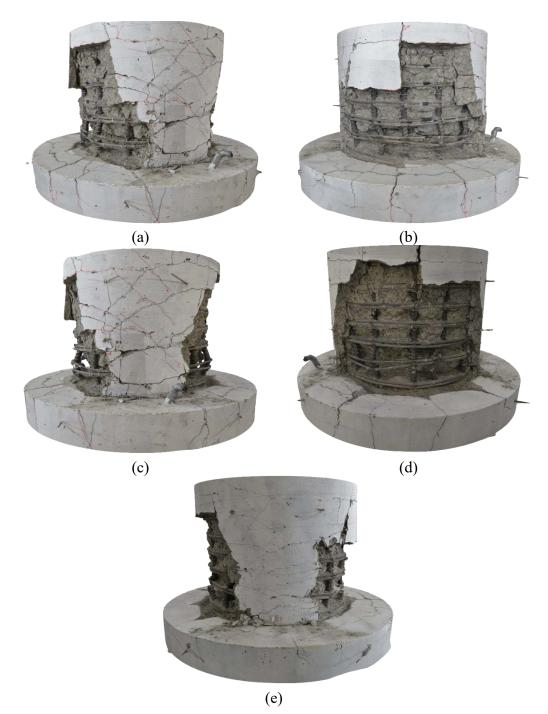
Figure 3.22. 360° Detailed 3D Point Cloud Model Showing Extent of Damage in Column Plastic Hinge Region Post-Test
