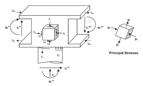
Figure 4.7. Joint Shear Stresses in T-Joints (Caltrans SDC 2.0 Figure C7.4.2-1)
