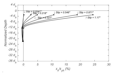
Figure 2.28. Transverse Hoop Strain Profile in Specimen #4
