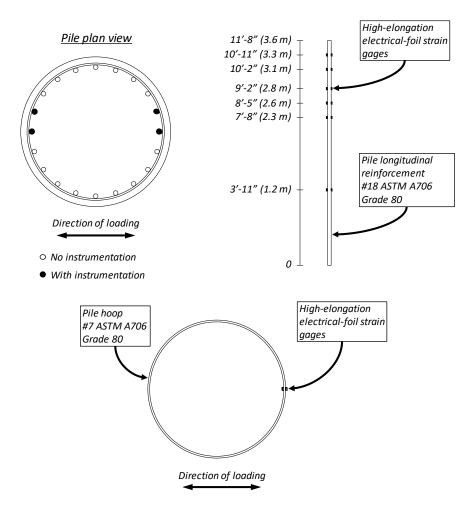
Figure 3.13. Representative Pile Longitudinal and Transverse Reinforcement Instrumentation
