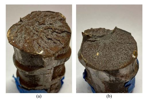
Figure 5.20. Fracture Surface of (a) Spec06 (SH3); (b) Spec08 (SH3)
