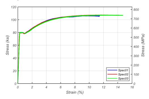
Figure 5.9. Smoothed-Rib-Radii #14 ASTM A706 Grade 80 Tensile Test Data
