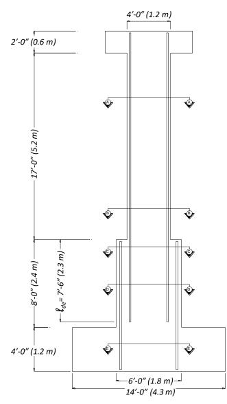
Figure 3.3. General Dimensions of Test Specimen (Elevation View)
