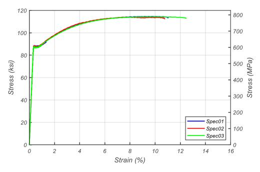
Figure 5.8. Normal #14 ASTM A706 Grade 80 Tensile Test Data
