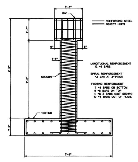
Figure 5.37. Typical Test Specimen Dimensions and Reinforcement Layout (Moyer & Kowalsky, 2003)
