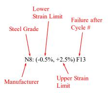
Figure 5.13. Coding System for Identifying Test Bars
