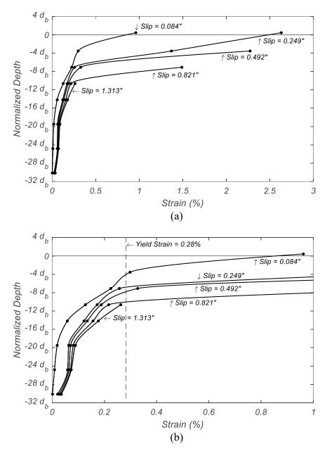
Figure 2.23. Strain Profile of Test Bar in Specimen #3: (a) Overall; (b) Closeup View Displaying Yield Penetration
