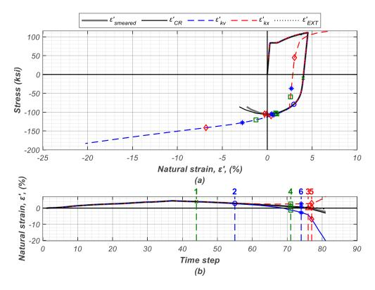
Figure 5.29. Local vs Smeared Response in Buckled Reinforcement, Case 28: (a) Natural Strain vs Stress; (b) Natural Strain Time-History
