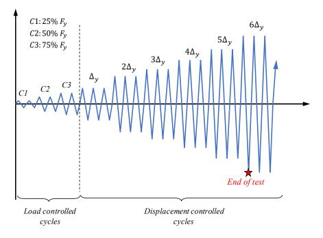
Figure 4.12. Test Specimen Loading Protocol
