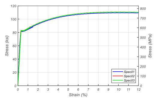
Figure 2.2. Monotonic Stress-Strain Response of ASTM A706 Grade 80 #18 Bars
