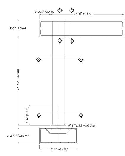
Figure 4.4. General Dimensions of Test Specimen (Elevation View)
