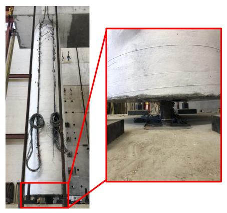
Figure 4.3. Proprietary Hinge at Column Base
