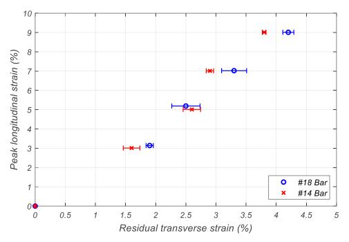
Figure 2.9. Relationship Between Measured Residual Transverse and Peak Longitudinal Strains
