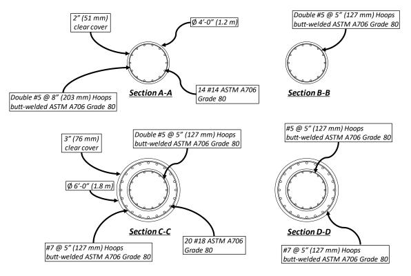
Figure 3.4. Reinforcement Configuration of Test Specimen
