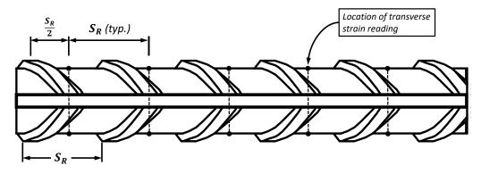
Figure 2.7. Consistent Measurement Location Between Deformations on Bar
