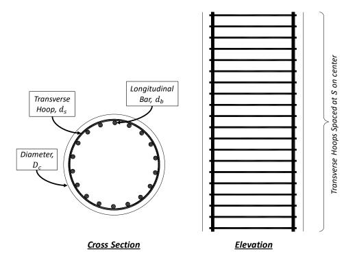
Figure 5.24. Column Reinforcement Cage Configuration
