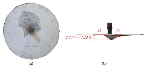
Figure 2.14. 3D Point Cloud Model of Fracture Surface of Test Specimen #1: (a) Plan View; (b) Cone Shaped Fracture
