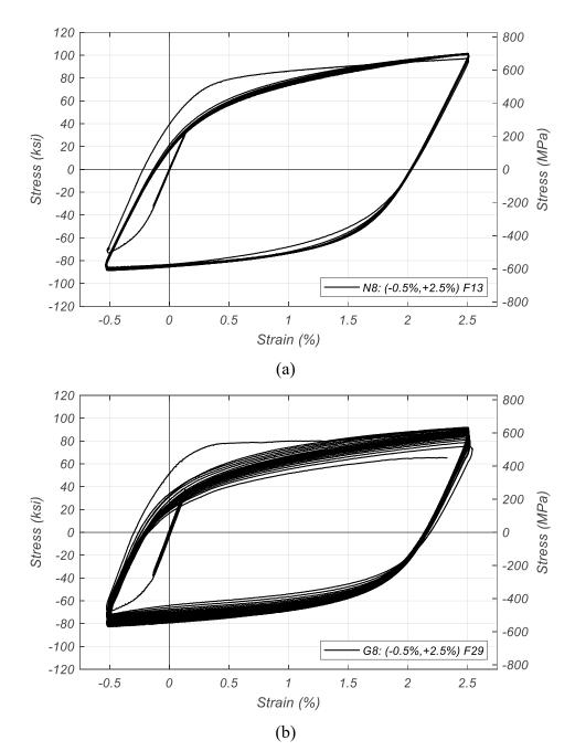
Figure 5.15. Hysteretic Response of: (a) Normal; (b) Smoothed-Rib-Radii Test Bars to Loading Protocol SH2
