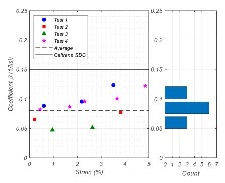
Figure 3.55. Comparison of Coefficient  $\beta$  in Yield Penetration Test Columns
