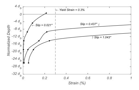
Figure 2.20. Transverse Hoop Strain Profile in Specimen #2
