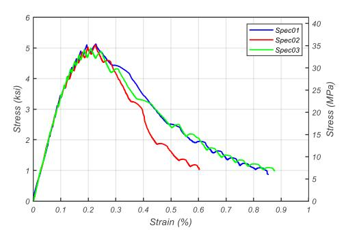
Figure 3.7. Monotonic Stress-Strain Response of Column Elsewhere Concrete at DOT
