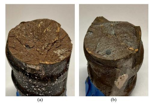
Figure 5.18. Fracture Surface of (a) Spec01 (SH1); (b) Spec10 (SH1)
