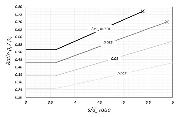
Figure 5.34. Confinement Ratio vs Hoop Spacing for Various von Karman Strain Amplitudes
