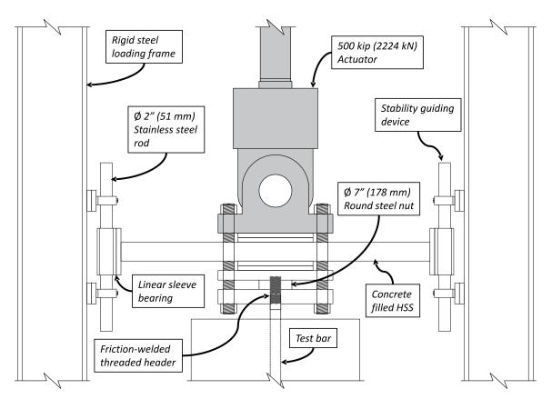
Figure 2.6. Actuator-Test Bar Connection with Stability Guiding Device
