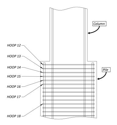
Figure 3.35. Pile Hoops Instrumented with High-Elongation Electrical Foil Strain Gages
