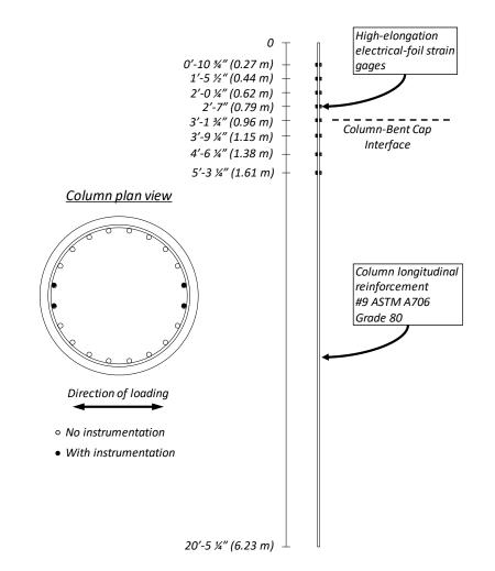
Figure 4.14. Representative Column Longitudinal Reinforcement Instrumentation
