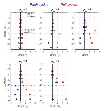
Figure 4.28. Measured Strains of Northern-Most Column Longitudinal Bars (from Strain Gages) at Peak Displacements of Various Cycles
