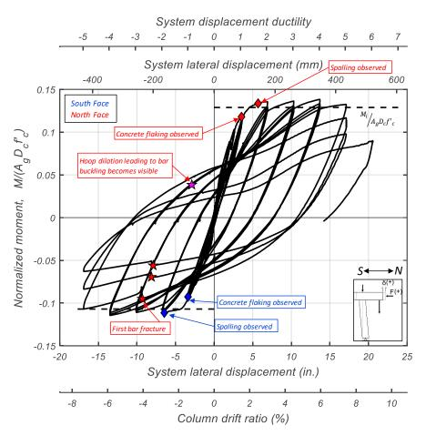
Figure 4.18. Normalized Column Moment-Displacement Response of Test Specimen
