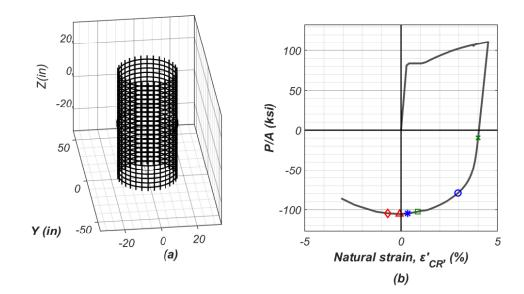
Figure 5.26. Global Response of FE Model, Case 28: (a) 3D Representation of Buckled Shape; (b) Smeared Natural Strain vs Stress in a Single Longitudinal Bar Identifying Key Analysis Steps
