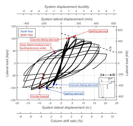
Figure 4.17. Global Lateral Load-Displacement Response of Test Specimen
