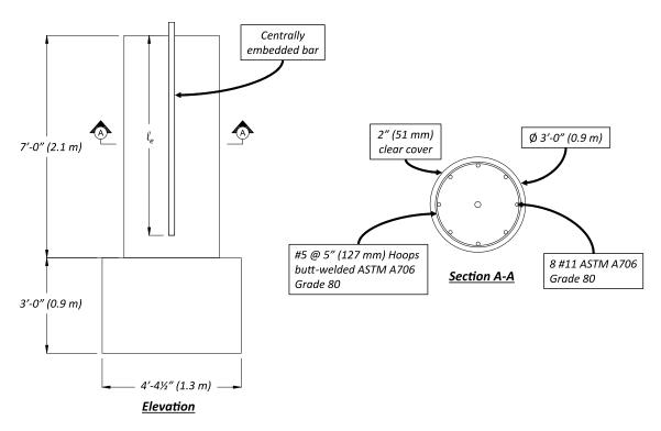
Figure 2.1: Test Specimen Design, Elevation and Plan View
