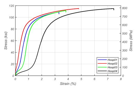
Figure 3.5. Butt-Welded Column Hoop Validation Tensile Tests
