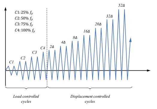
Figure 2.11. General Loading Protocol for All Test Specimens
