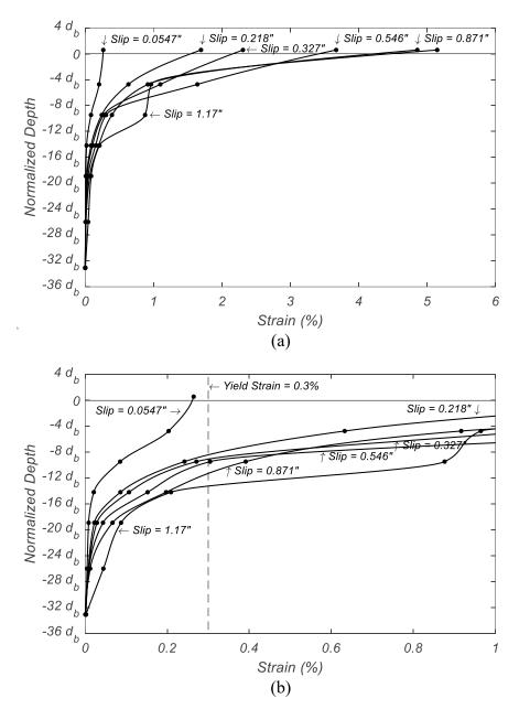
Figure 2.27. Strain Profile of Test Bar in Specimen #4: (a) Overall; (b) Closeup View Displaying Yield Penetration
