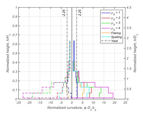
Figure 3.23. Curvature Profile of Column Obtained from Linear Potentiometers
