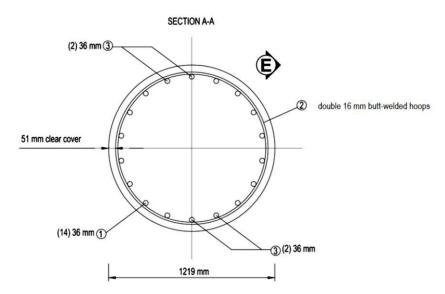
Figure 3.48. Large Bridge Column (L.B.C.) Test Specimen from Schoettler et al., Column Cross-Section
