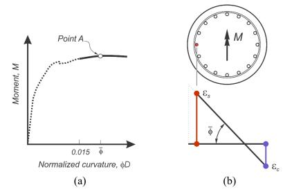
Figure 3.38. Smeared-Strain Compatible Method for Equivalent Plastic Hinge Length: (a) Domain Used in the Theoretical Moment-Curvature Response; (b) Section Strain Profile at Point "A" (Duck et al., 2018)
