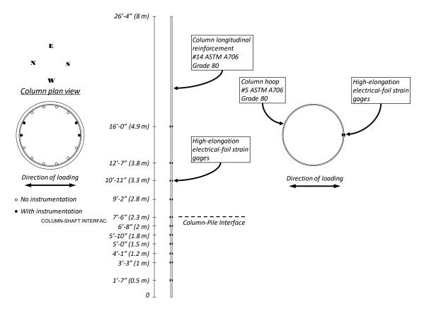
Figure 3.12. Representative Column Longitudinal and Transverse Reinforcement Instrumentation
