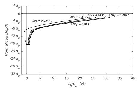
Figure 2.24. Transverse Hoop Strain Profile in Specimen #3
