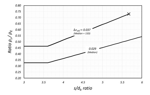
Figure 5.36. Confinement Ratio vs Hoop Spacing for Median and Median+1SD von Karman Strain Amplitudes
