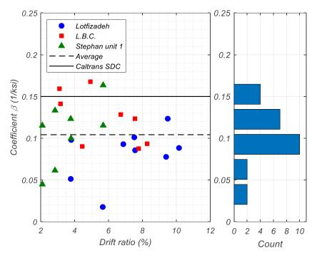
Figure 3.54. Comparison of Coefficient  $\beta$  in Column Tests
