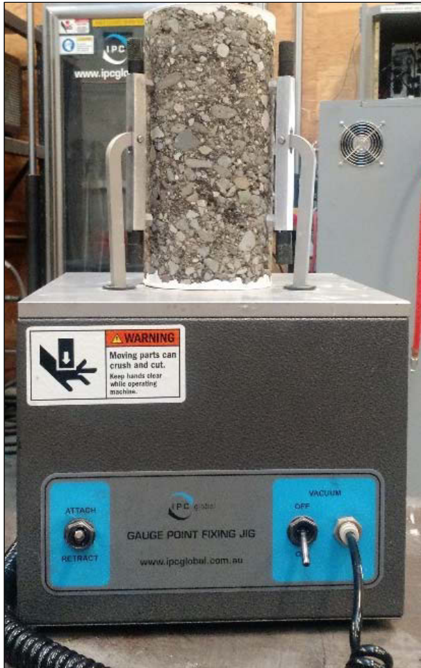
Figure 6.16: Modified jig for mounting LVDTs on 200 mm × 100 mm specimens.
