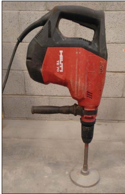
Figure 6.4: Vibrating compaction hammer with 148 mm compaction attachment.
