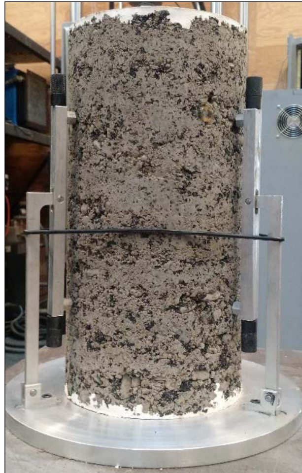
Figure 6.17: Fabricated jig for mounting LVDTs on 300 mm × 150 mm specimens.
