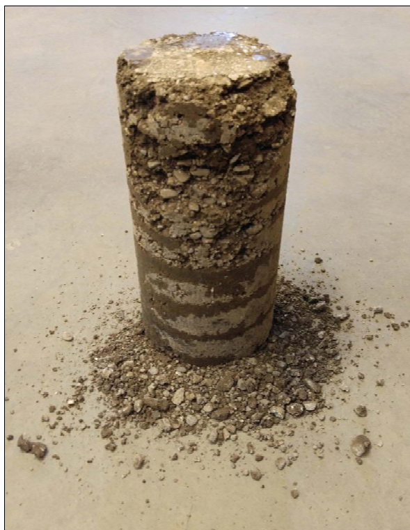
Figure 5.2: Result of microcracking effort with vibrating hammer.
