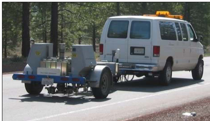
Figure 2.11: Falling weight deflectometer.
