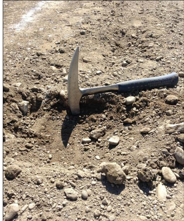
Figure 3.14: CR99: Depth of delaminated material (50 mm [2 in.]).
