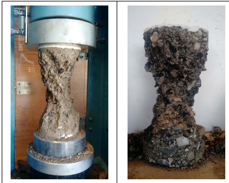
Figure 2.18: Shear failure of FDR-PC and FDR-FA specimens after UCS testing.
