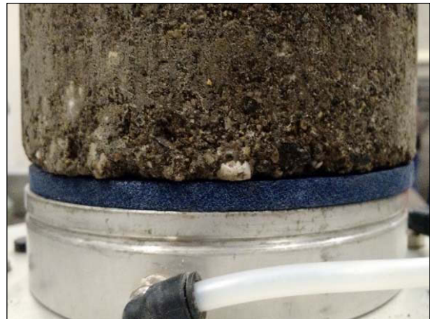
Figure 6.15: Irregular specimen ends leading to poor contact.
