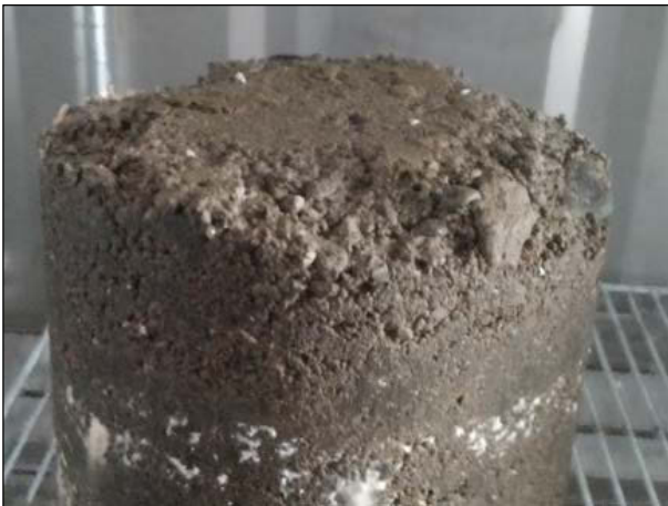
Figure 6.14: Broken edges caused by brittle nature of stabilized material.
