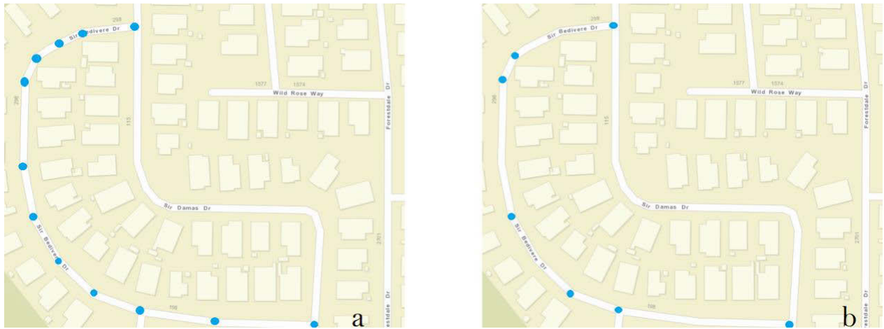
a. a curved link is split into 11 straight links
