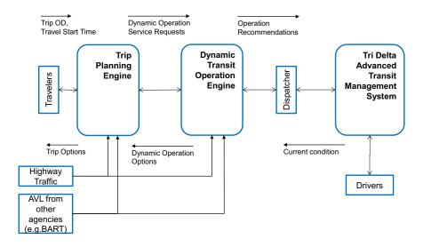
Figure 3. IDTO Conceptual Architecture
