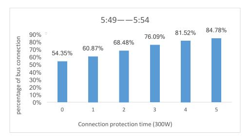
Figure 29. Connection success rate of T-CONNECT of 380W to 300W (trip 1090) at Hillcrest P & R
