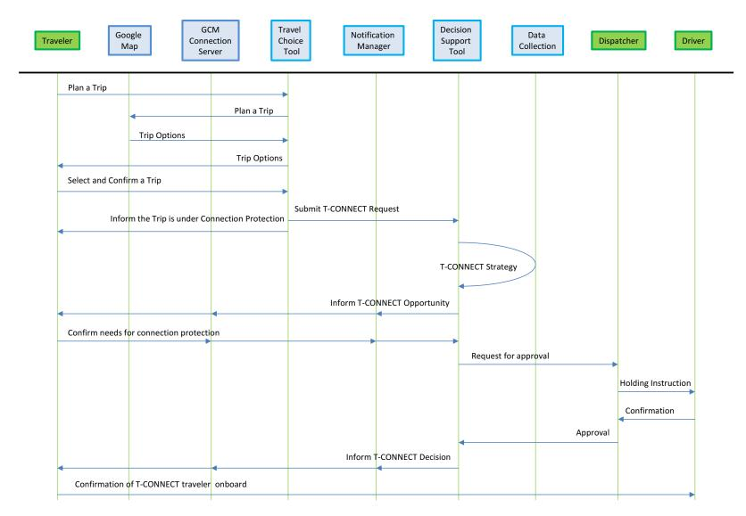
Figure 6. Sequence Diagram of Scenario 1: T-CONNECT
