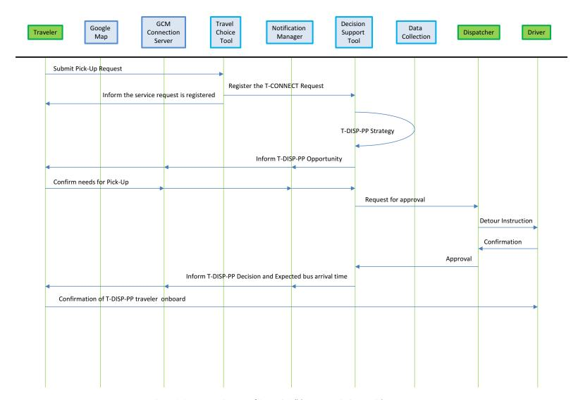
Figure 8. Sequence Diagram of Scenario 2(b) Route Deviation to Pick Up Passenger
