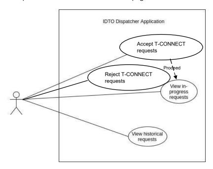
Figure 13. Interactions on the Dispatcher Interface
