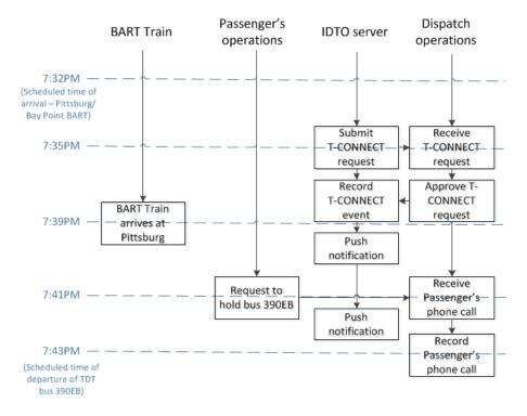
Figure 39. Parallel testing flow of T-CONNECT
