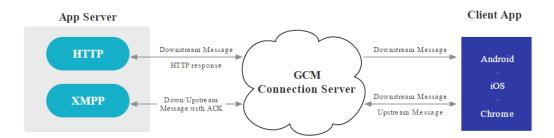
Figure 11. GCM mechanism
