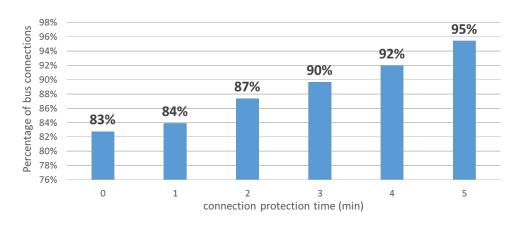
Figure 31. Connection success rate of T-CONNECT of 388W to 300W (trip 1087) at Hillcrest P& R
