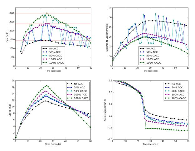
Figure 2.22: Case with red light downstream: comparison of point measurements of flow, distance to leader, speed and acceleration at the detector location for different portions of ACC/CACC traffic.
