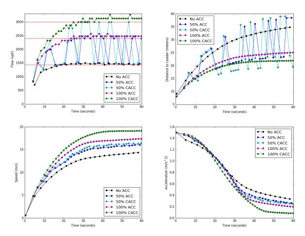
Figure 2.21: Single intersection case: comparison of point measurements of flow, distance to leader, speed and acceleration at the detector location for different portions of ACC/CACC traffic.
