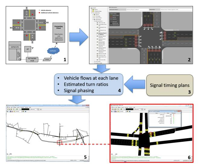
Figure 2.2: Process of data collection, analysis and building the simulation model.
