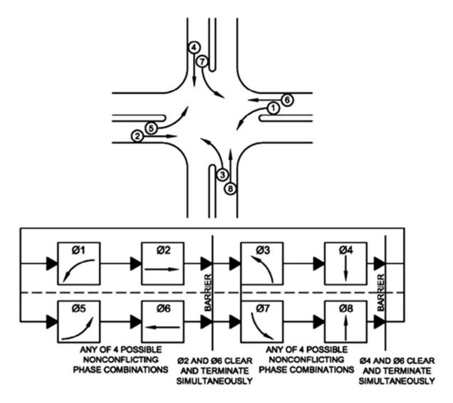
Figure 1.2: An intersection with four approaches, each with a through and left-turn movement (top), and a ring-and-barrier diagram to organize the movements (bottom). Source: [15].
