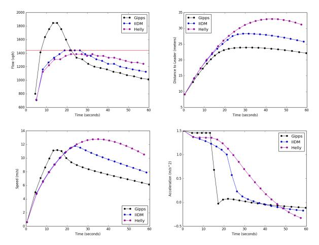
Figure 2.18: Experiment with a red light ahead: comparison of point measurements of flow, distance to leader, speed and acceleration at the detector location between the three car following models.
