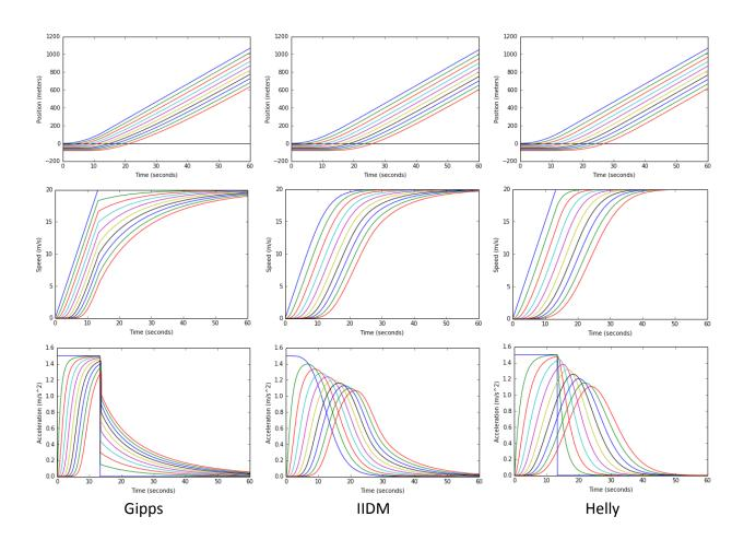
Figure 2.14: Experiment with a free road ahead: comparison of vehicle trajectories, speeds and accelerations between the three car following models.
