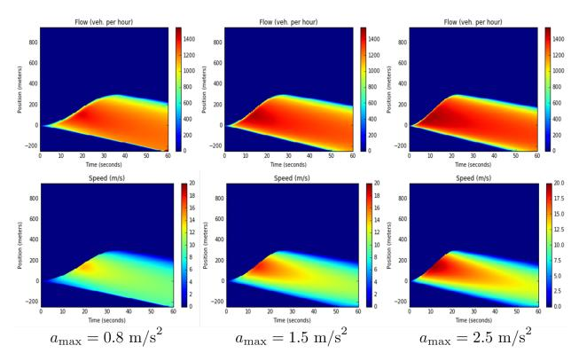
Figure 2.20: Flow (top) and speed (bottom) contours generated by the IIDM-induced macroscopic model in the experiment with the red light downstream for  $a_{\text{max}} = 0.8$ , 1.5 and 2.5 m/s<sup>2</sup>.
