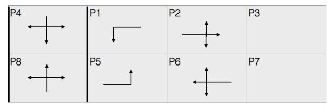
Figure 2.4: The dual-ring diagram; phases  $p_3$  and  $p_7$  have zero duration. The thicker vertical lines are the two barriers.
