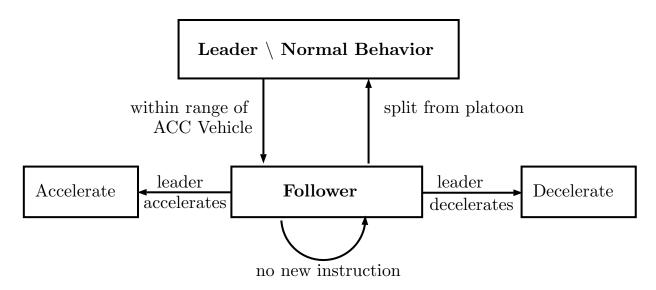
Figure 2.24: State machine describing platoon behavior.
