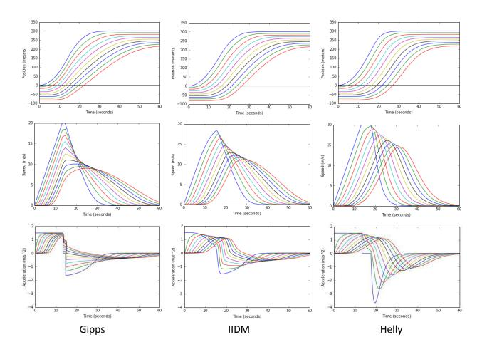
Figure 2.17: Experiment with a red light ahead: comparison of vehicle trajectories, speeds and accelerations between the three car following models.
