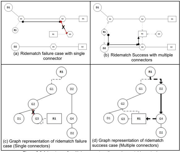
Figure 3.3 Advantage of multiple connectors (improving matching rates)
