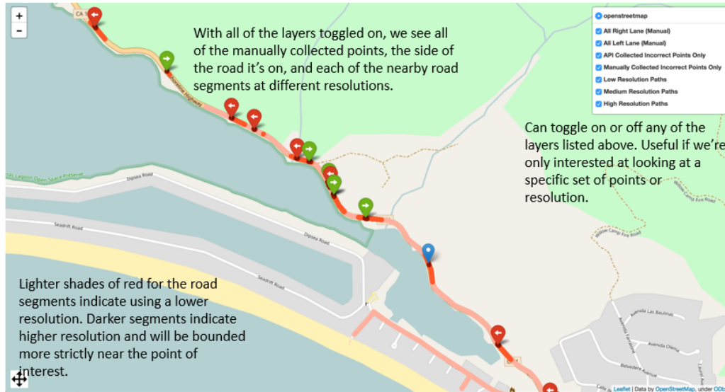
Figure 5.6. Path-based reconstruction of speed profiles along a route using varying spatial resolutions of the query
