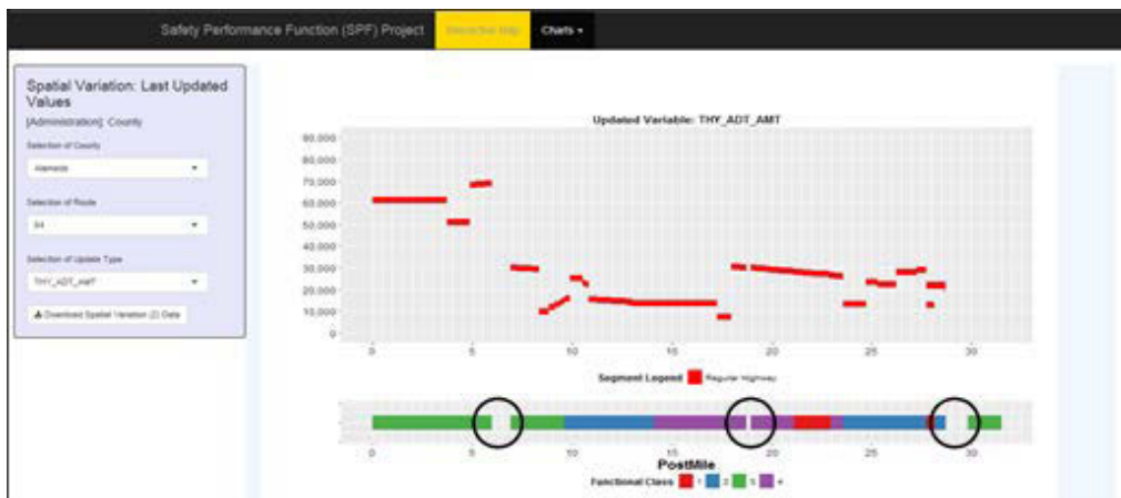
Figure 4.3. Last updated values of AADT across different functional classes of HWY84, Alameda
