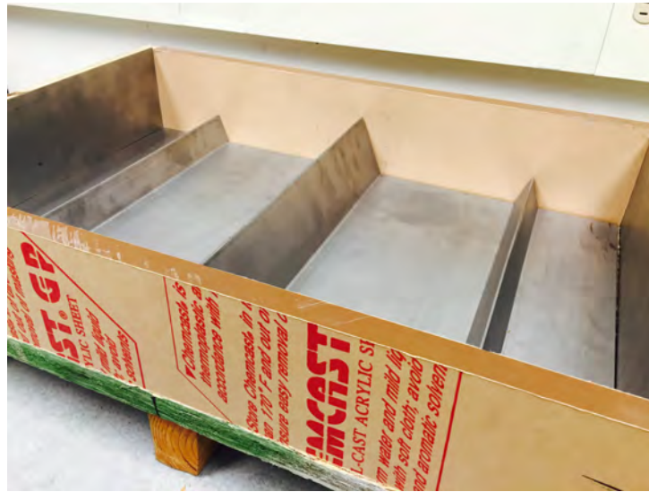
Figure D.11: Formwork for plastic shrinkage test
