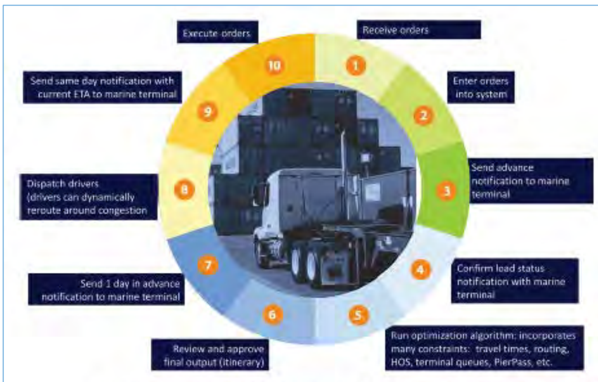
Figure 2 Overview of FRATIS system 10-step process for uses in the LA-Gateway FRATIS Demonstration (Jensen, Fayez and DeSantis, 2015)
