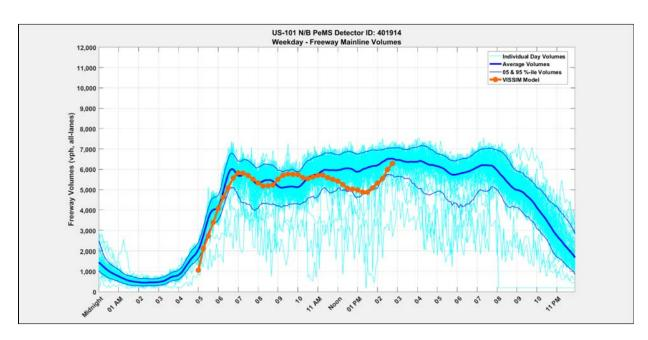
Figure 4.06: PeMS VDS 401914, At Hillsdale Blvd, P.M. 11.20 US-101 Northbound Traffic Volumes (Caltrans PeMS & VISSIM Simulation Model)
