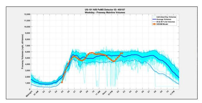
Figure 4.07: PeMS VDS 400107, Opposite EB 92 RM-S-Diag, P.M. 11.72 US-101 Northbound Traffic Volumes (Caltrans PeMS & VISSIM Simulation Model)
