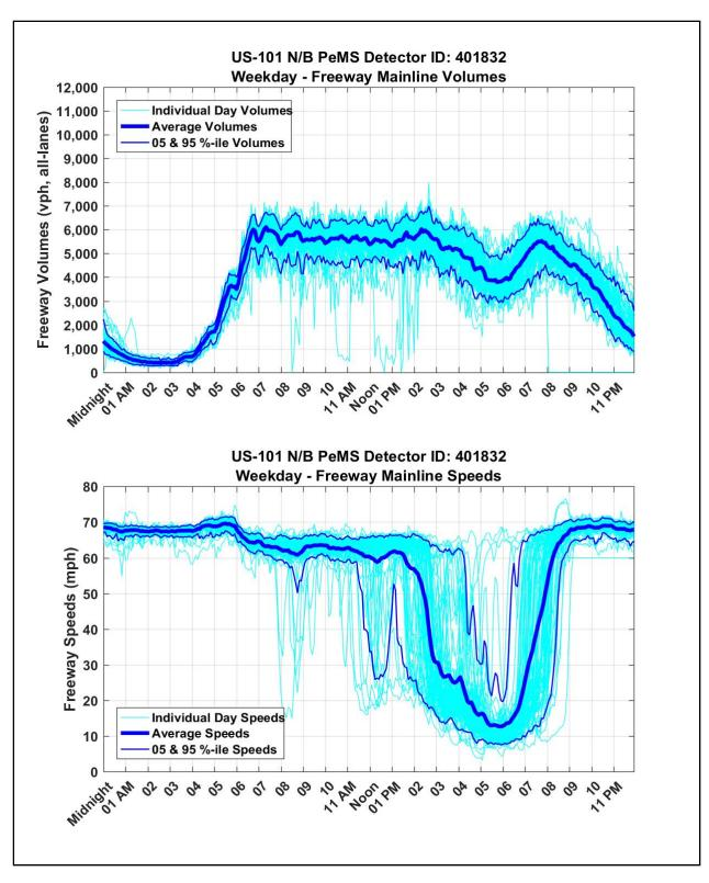
Figure 3.03: Mainline Hourly Traffic Volumes and Speeds (Average Weekday) PeMS Detector Station: 401832, "At Holly Street Diagonal On-Ramp"
