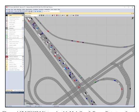
Figure 4.02 VISSIM Network with Mainline & Ramp Detectors (loops)
