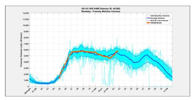
Figure 4.05: PeMS VDS 401882, At Holly Street On-Ramp, P.M. 8.34 US-101 Northbound Traffic Volumes (Caltrans PeMS & VISSIM Simulation Model)
