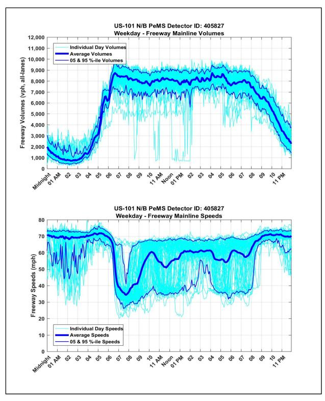
Figure 3.01: Mainline Hourly Traffic Volumes and Speeds (Average Weekday) PeMS Detector Station: 405827, "At Kehoe Ave Off-Ramp"
