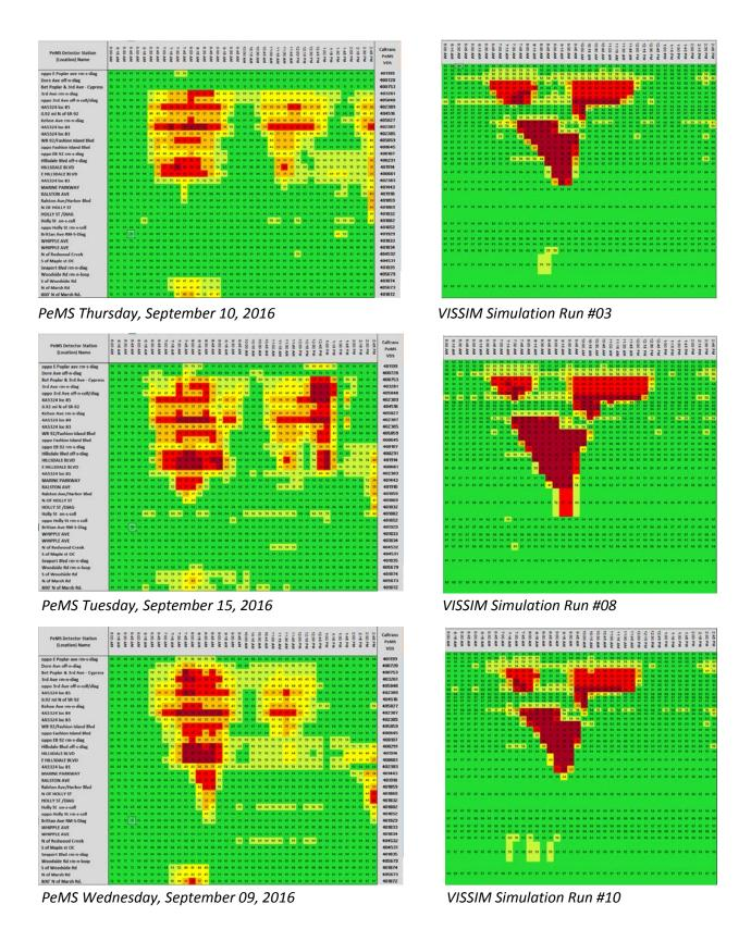
Figure 4.03: US-101 Northbound Congestion Scans (Caltrans PeMS & VISSIM Simulation Model)
