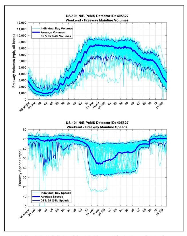
Figure 3.04: Mainline Hourly Traffic Volumes and Speeds (Average Weekend) PeMS Detector Station: 405827, "At Kehoe Ave Off-Ramp"
