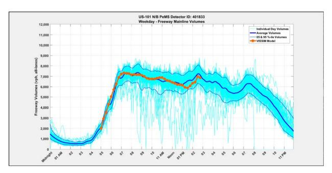
Figure 4.04: PeMS VDS 401833, At Whipple Avenue, P.M. 6.63 US-101 Northbound Traffic Volumes (Caltrans PeMS & VISSIM Simulation Model)
