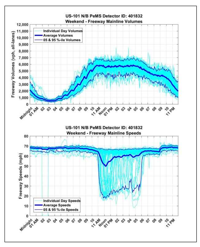
Figure 3.06: Mainline Hourly Traffic Volumes and Speeds (Average Weekend) PeMS Detector Station: 401832, "At Holly Street Diagonal On-Ramp"
