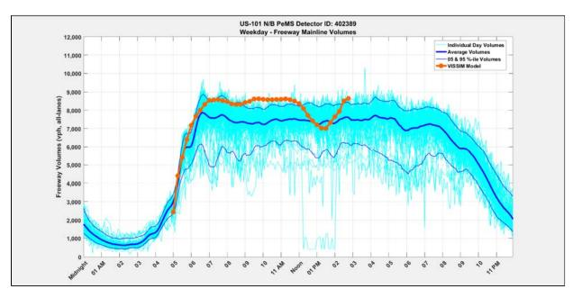
Figure 4.08: PeMS VDS 402389, South of the 3rd Avenue Interchange, P.M. 13.00 US-101 Northbound Traffic Volumes (Caltrans PeMS & VISSIM Simulation Model)
