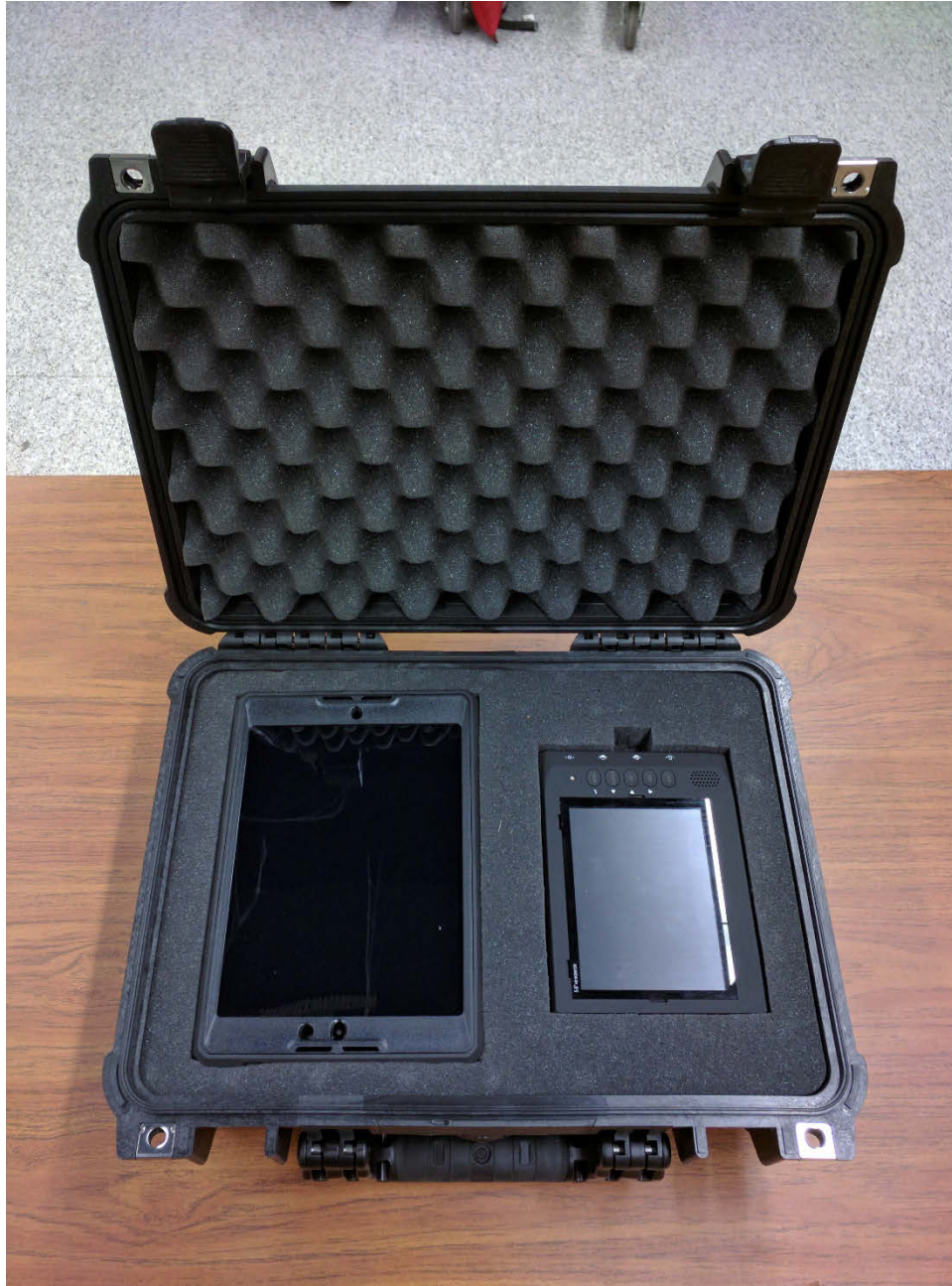
Figure 6.2: HHT primary kit internals, i.e. the tablet and the LCD video monitor
