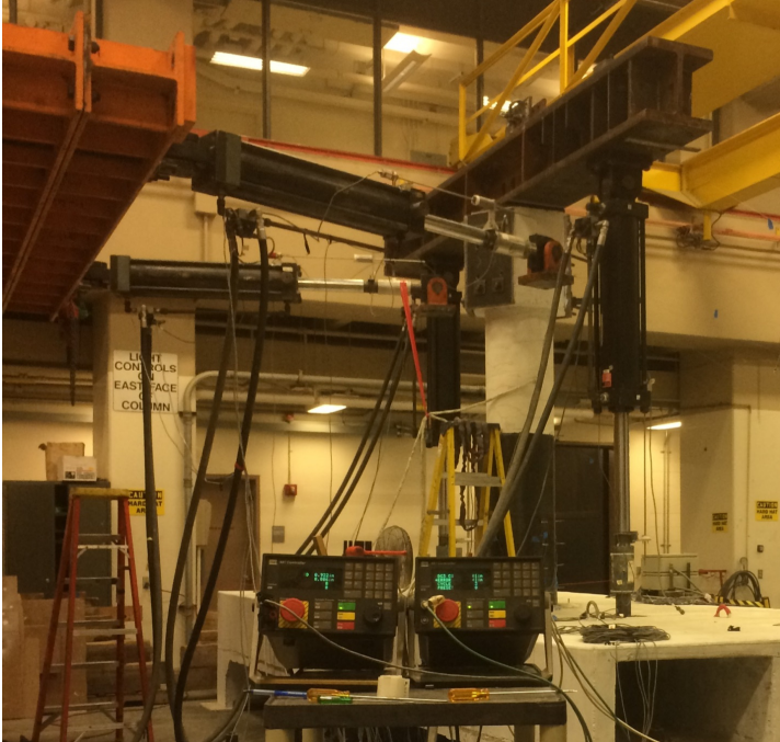
Figure 2.14 Actuators detached from the specimen for conducting trial HS tests.
