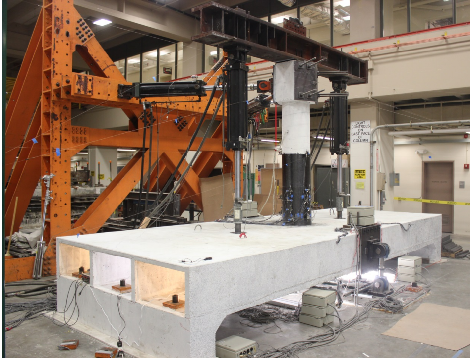
Figure 2.32 Test set-up used for conducting HS trial tests for the repaired Specimen No. 1.
