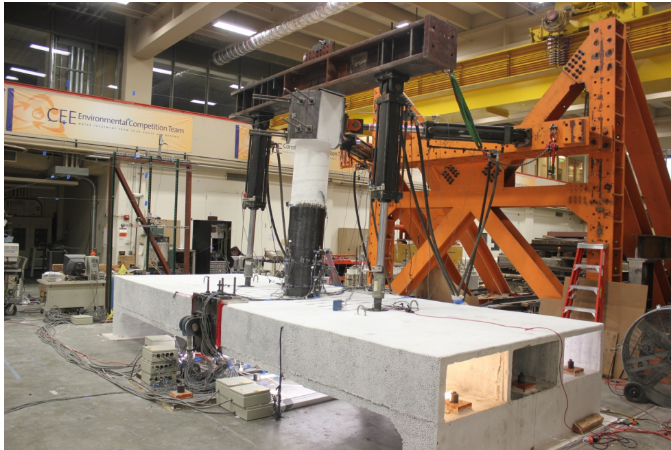
Figure 3.6 Retrofitted Specimen No. 2 HS test set-up during a bi-directional run.
