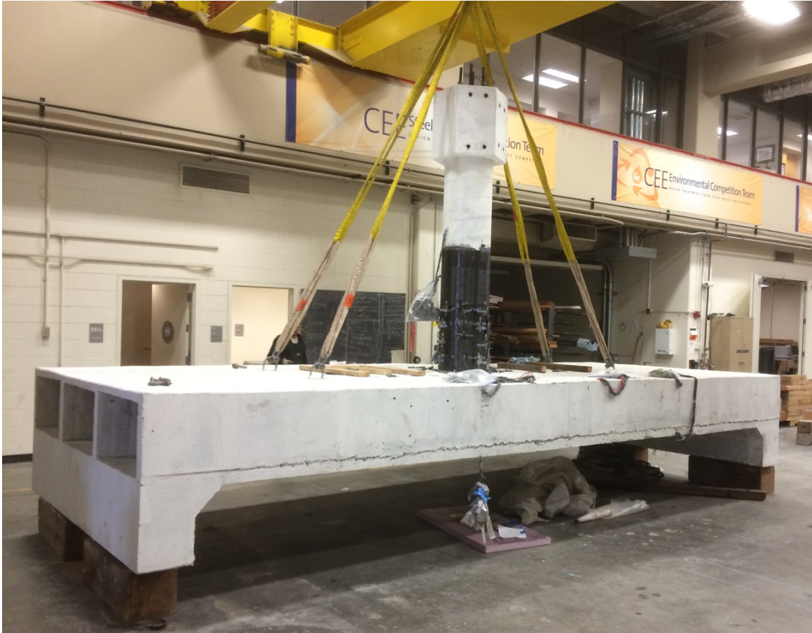
Figure 2.4 Physical experimental substructure (retrofitted Specimen No. 2) used in the HS tests.
