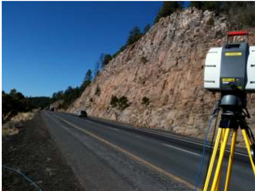
Figure 7. The Arizona site, showing the Leica scanner used to conduct scans.
