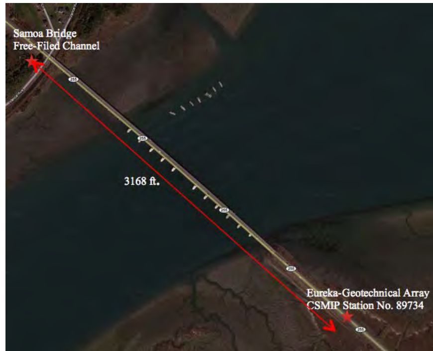
Figure 2-19: Positions of the two free-field stations near the Eureka-Samoa Channel Bridge.
