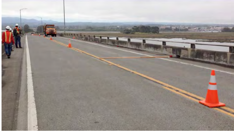
Figure 3-5: Truck test #1 (the 2-by-4 lumber piece is visible on the far lane).
