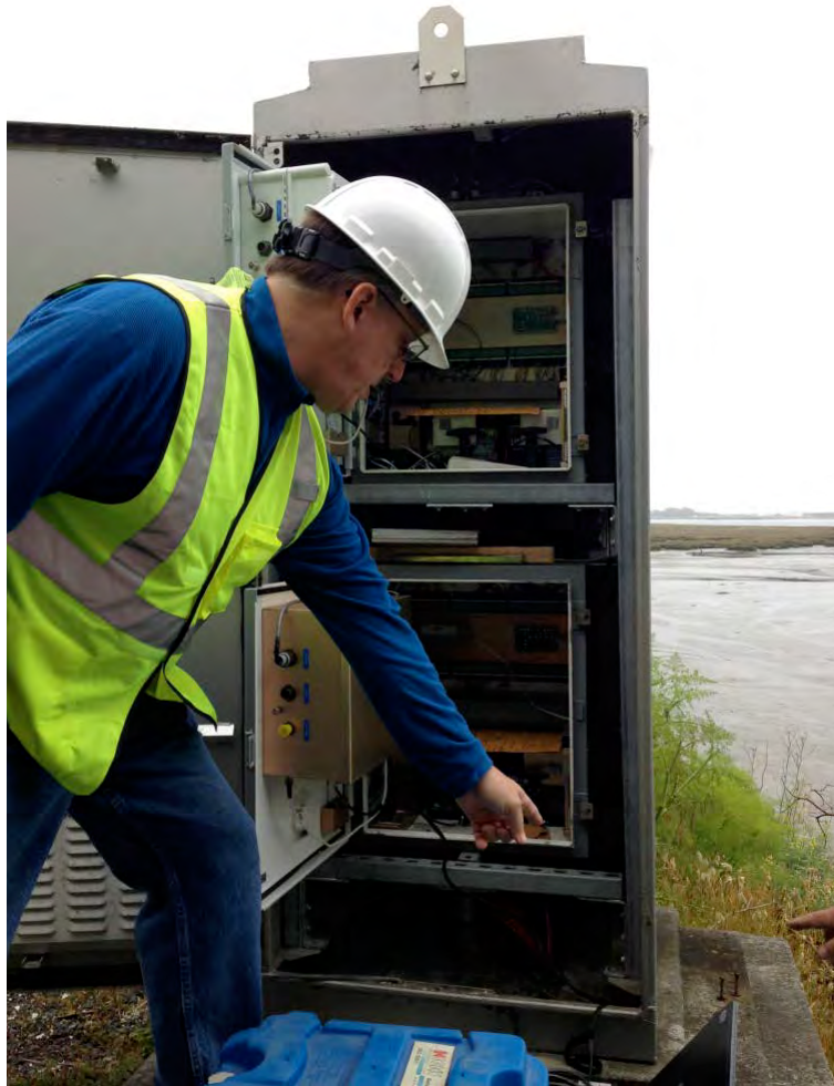
Figure 1-9: Two existing data acquisition (DAQ) units installed and operated by the California Geological Survey (CGS) (Co-PI, Robert Nigbor pictured).
