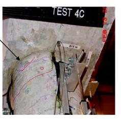
Damage State 2 (after test 4C)
