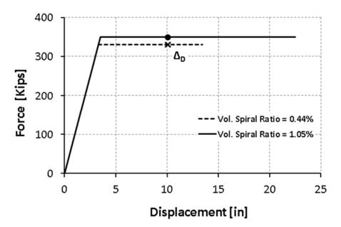
Figure 5-1. Displacement demand for different spiral ratios
