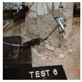
Damage State 3 (after test 6)
