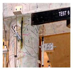
Damage State 4 (after test 6)
