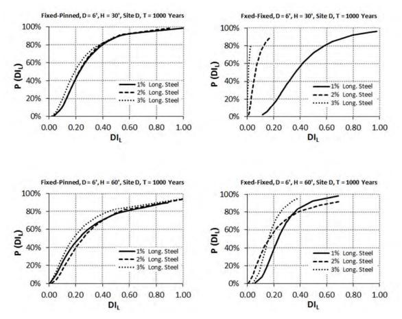
Figure 4-29. Fragility curves for TCBs with six foot diameter columns for Site D
