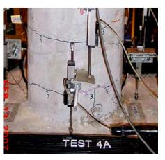
Damage State 2 (after test 4A)
