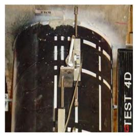
Damage State 2 (after test 4D)
