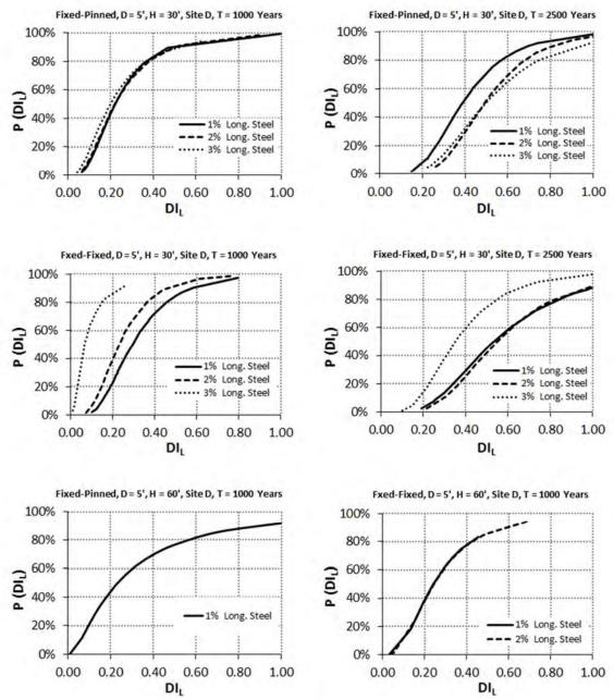
Figure 4-27. Fragility curves for TCBs with five foot diameter columns for Site D
