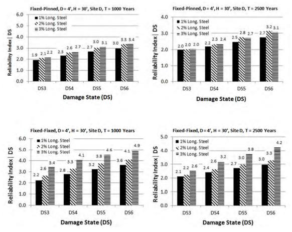
Figure 4-32. Reliability indices for FCBs with four foot diameter columns for Site D
