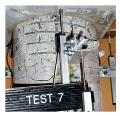
Damage State 5 (after test 7)
