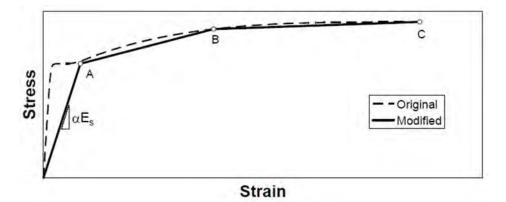
Figure 6-4. Original and modified stress-strain relationship for steel (Vosooghi and Saiidi 2010)
