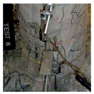
Damage State 5 (after test 6)
