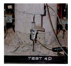
Damage State 3 (after test 4D)
