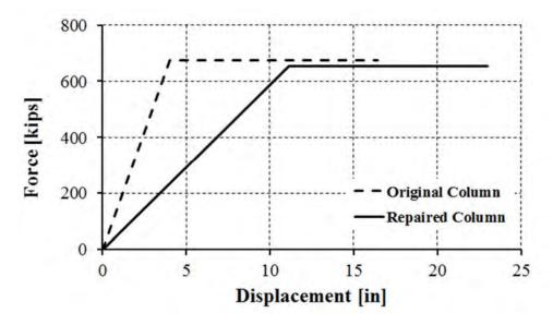
Figure 6-7. Idealized force-Displacement curves for the original and repaired columns
