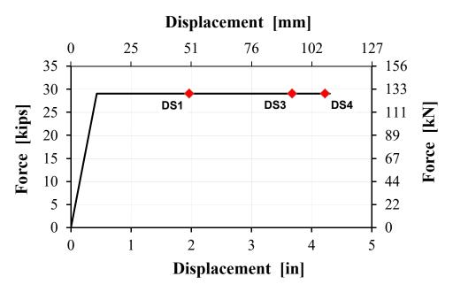
Figure 3-23. Idealized pushover curve and damage states for bent 2 East column
