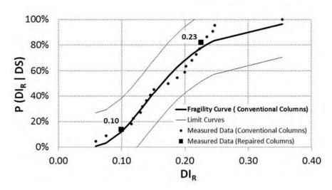
Figure 6-2. Resistance fragility curve for DS2 in conventional columns
