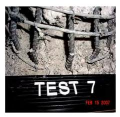
Damage State 6 (after test 7)
