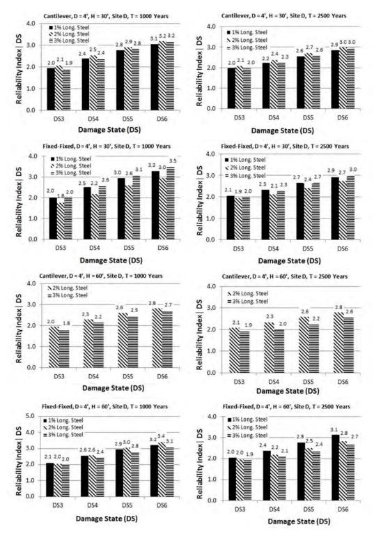
Figure 4-18. Reliability indices for SCBs with four foot diameter columns for Site D
