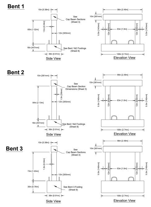
Figure 3-2. Bents configuration (Saiidi et al. 2013)
