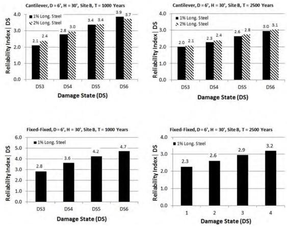
Figure 4-20. Reliability indices for SCBs with six foot diameter columns for Site B/C
