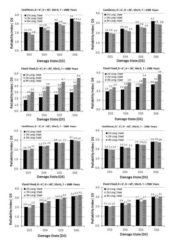
Figure 4-22. Reliability indices for SCBs with six foot diameter columns for Site D
