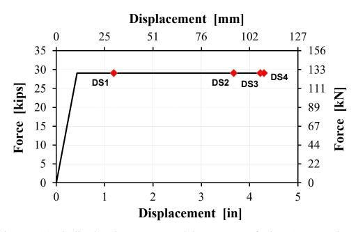
Figure 3-24. Idealized pushover curve and damage states for bent 2 West column
