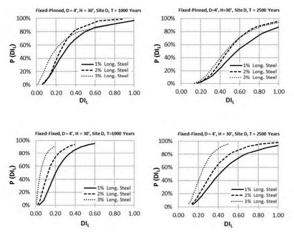
Figure 4-31. Fragility curves for FCBs with four foot diameter columns for Site D
