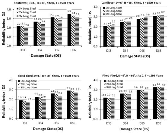
Figure 4-25. Reliability indices for SCBs with six foot diameter columns for Site D
