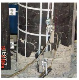
Damage State 3 (after test 5)Damage State 4 (after test 7)Figure 3-11. Apparent damage states for bent 3 East column bottom plastic hinge
