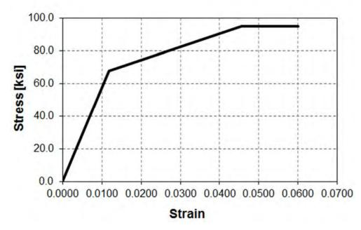
Figure 6-5. Modified stress-strain relationship for steel used for cantilever SCB
