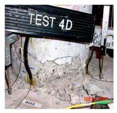
Damage State 3 (after test 4D)
