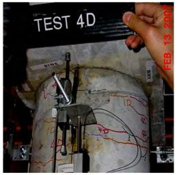
Damage State 2 (after test 4D)
