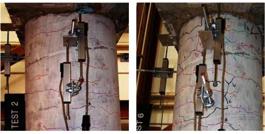
Damage State 1 (after test 2)
