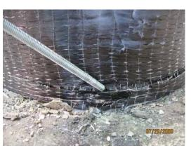
NHS2-R (DS3) NHS2-R (DS6) Figure 6-1. Damage states for repaired columns
