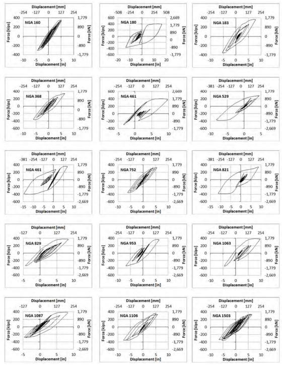
Figure 4-16. Force-displacement hysteresis curves for near-field GMs
