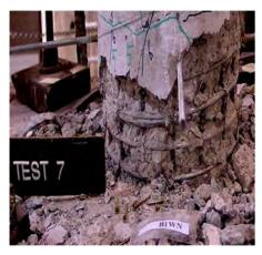
Damage State 5 (after test 7)
