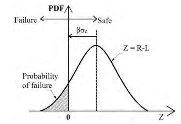
Figure 2-5. Graphical representation of reliability index and probability of failure (Cornell 1969)
