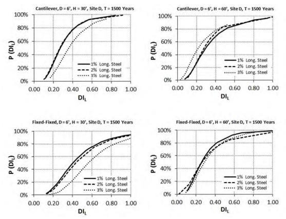
Figure 4-23. Fragility curves for SCBs with six foot diameter columns for Site D analyzed under 1500-year earthquake
