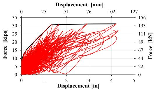
Figure 3-17. Bent 2 measured force-displacement hysteresis curves and envelope
