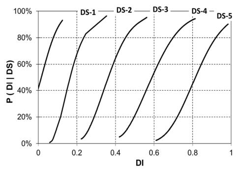
Figure 2-2. Correlation between damage states and damage indices
