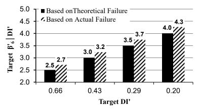
Figure 5-5. The target  $\beta'_6$  for a given design DI' for FCBs
