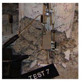
Damage State 4 (after test 7) Figure 3-9. Apparent damage states for bent 2 West column bottom plastic hinge
