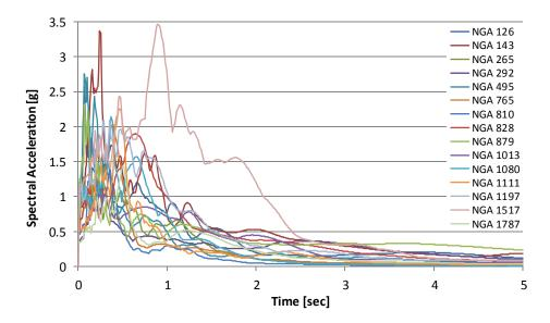
Figure 4-2. Near-field ground motions response spectrum of site class B/C
