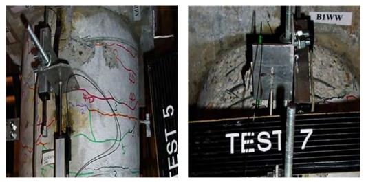
Damage State 3 (after test 5)
