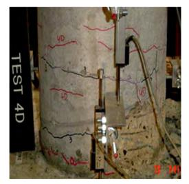
Damage State 4 (after test 4D)
