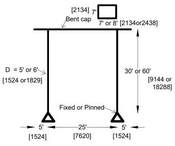
Figure 4-13. Typical two column bents configuration
