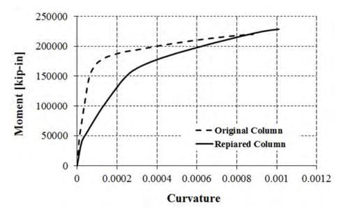
Figure 6-6. Moment curvature curves for the original and repaired columns
