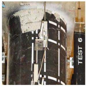
Damage State 4 (after test 6)
