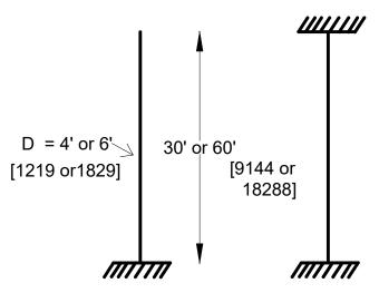
Figure 4-12. Typical single column bents configuration
