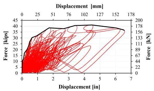
Figure 3-19. Bent 3 measured force-displacement hysteresis curves and envelope
