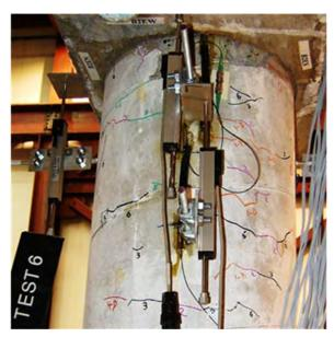
Damage State 3 (after test 6)
