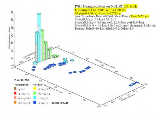
GMT 2014 Feb 7 18:46:12 Distance (R), magnitude (M), epsilon (E0.E) deaggregation for a site on rock with average vs\* 760. mis top 30 m. USGS CGHT PSHA2008 UPDATE Bins with it 0.05% contrib. omitted Figure 4-5. USGS Interactive Deaggregation Tool (Beta)
