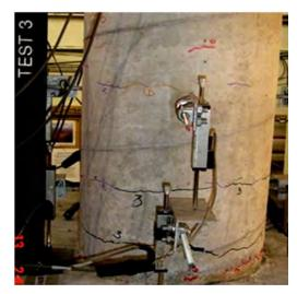
Damage State 1 (after test 3)
