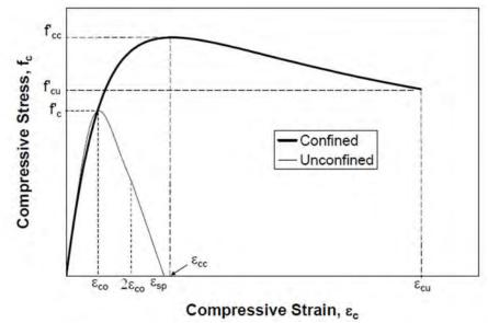
Figure 4-9. Mander's confined and unconfined concrete model
