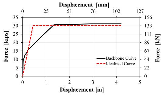
Figure 3-18. Bent 2 measured envelope and idealized force-displacement curve
