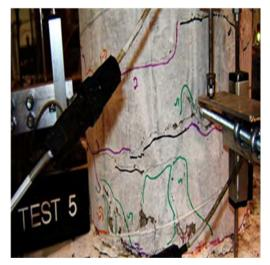
Damage State 2 (after test 5)
