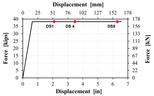
Figure 3-26. Idealized pushover curve and damage states for bent 3 West column
