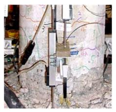
Damage State 4 (after test 5)
