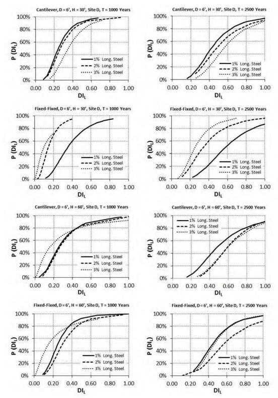
Figure 4-21. Fragility curves for SCBs with six foot diameter columns for Site D
