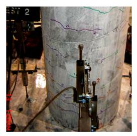
Damage State 1 (after test 2)
