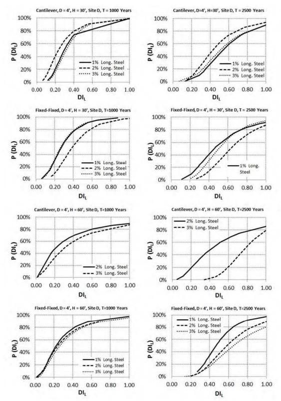
Figure 4-17. Fragility curves for SCBs with four foot diameter columns for Site D
