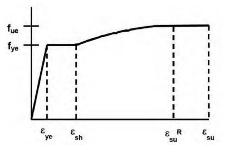
Figure 4-10. Steel stress strain model
