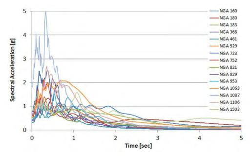
Figure 4-4. Near-field ground motions response spectrum of site class D
