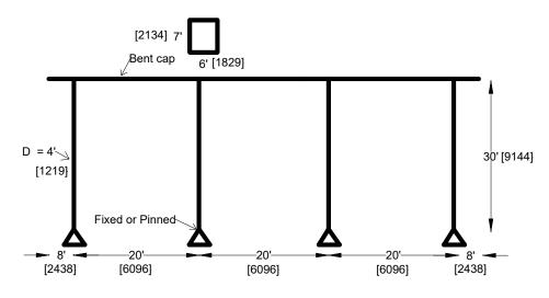
Figure 4-14. Typical four Column Bents configuration
