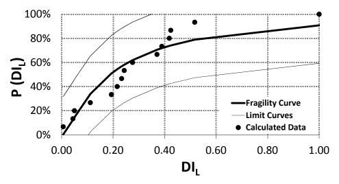
Figure 6-8. Fragility curve for DI<sub>L</sub> for the repaired column
