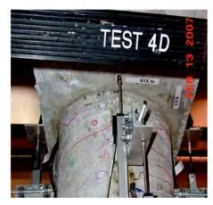
Damage State 3 (after test 4D)
