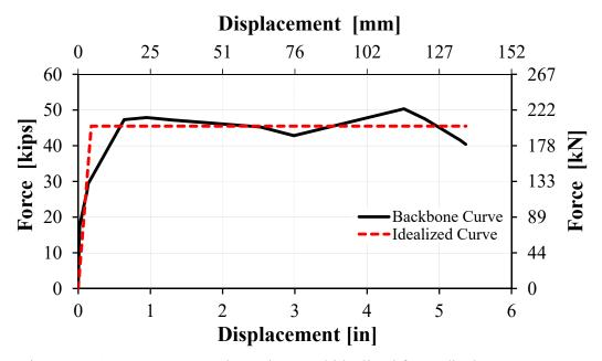
Figure 3-16. Bent 1 measured envelope and idealized force-displacement curve
