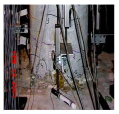
Damage State 2 (after test 3)
