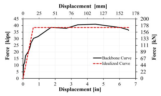
Figure 3-20. Bent 3 measured envelope and idealized force-displacement curve
