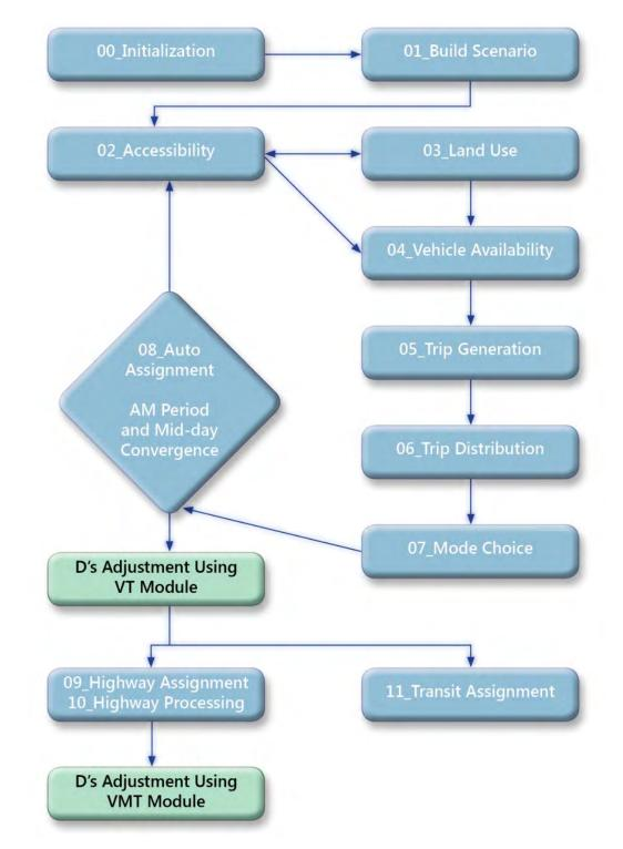
Figure 13. Trips-Based TDF Model Flowchart
