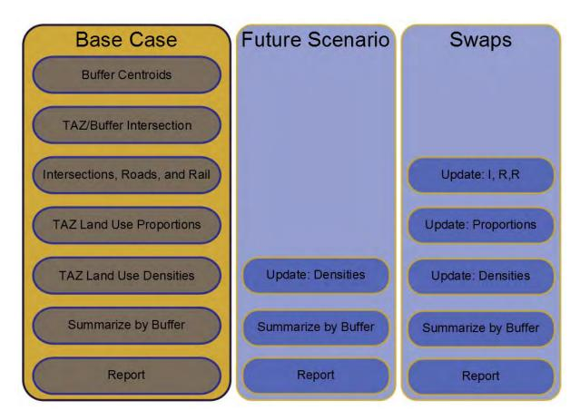
Figure 4. Process diagram for buffering. Showing the steps for the base case, and the additional steps needed to generate the future and swap scenarios.
