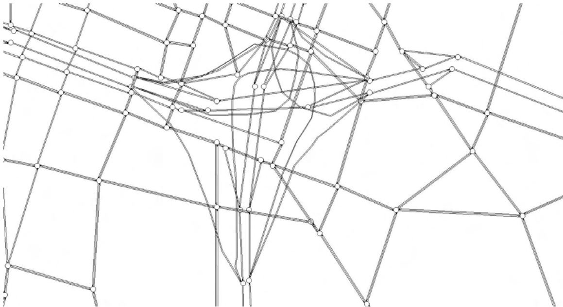
Figure 5.6: The interchange of I-80 and US-50 in Downtown Sacramento displayed in the new NetZone
