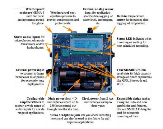
**Figure 6.** Wildlife Acoustics Song Meter SM2 recorder. The SM2 can be programmed to record on simple time-of-day schedules or more complex monitoring protocols such as recording relative to local sunrise, sunset and twilight.
