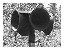
**Figure 1**. Acoustic horn configuration used for field recording of bird vocalizations.
