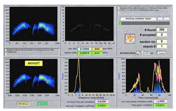
Signal search progress panel shown recognizing a willow flycatcher call found within a multi-hour recording. The upper left sonogram displays the exemplar search term used to seek matches in the recording.
