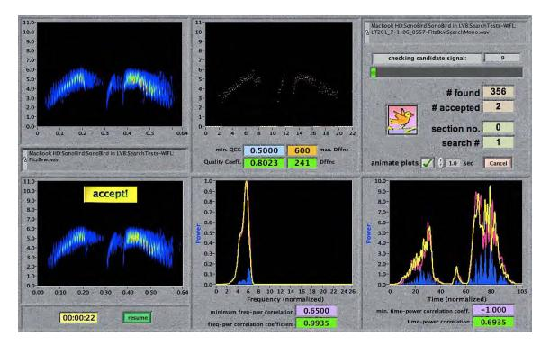
**Figure 8.** SonoBird search panel. SonoBird seeks for signals similar to a known species search term (upper left sonogram) by first running a coarse search to select file segments having basic similarity, then performs a more discriminating comparison with the candidate signal (lower left sonogram) using user-defined criteria. SonoBird saves search criteria in the search term file to facilitate repeated searches. See Appendix C for a full description and guide for use.
