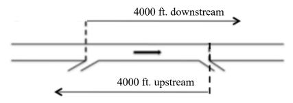
Figure 1. Location of collision data if the weaving section is shorter than 4000 ft
