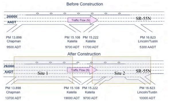
Figure 3. Geometric configuration of study sites 1 and 2
