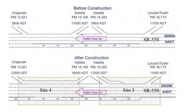
Figure 5. Geometric configuration of study sites 3 and 4
