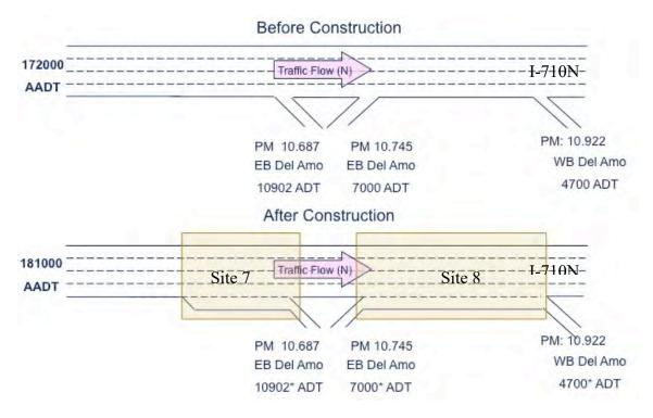
Figure 12. Geometric configuration of study sites 7 and 8
