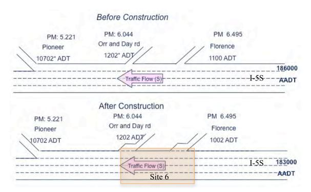
Figure 10. Geometric configuration of study site 6
