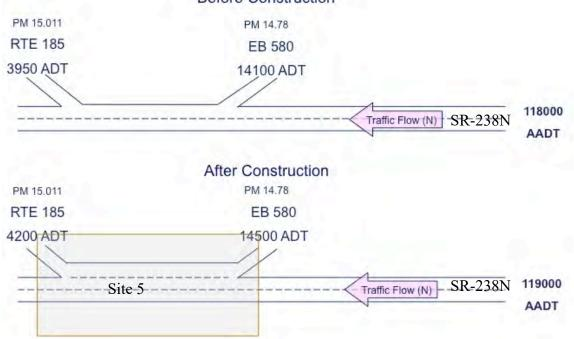
Figure 5. Geometric configuration of study site 5
