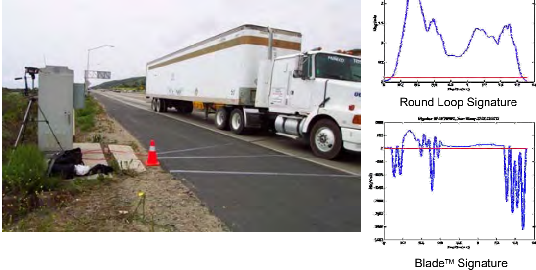
Figure 6.1 Example of Round and Blade™ inductive loop sensor signatures of a tractor trailer
