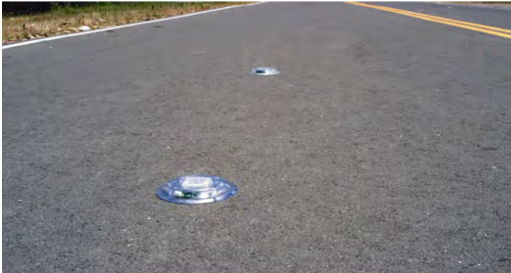
Figure 9. Sensys VDS240 Sensors on PATH Testbed
