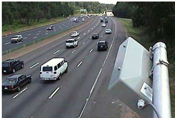
Figure 6 - Multi-lane highway monitoring using SAS-1
