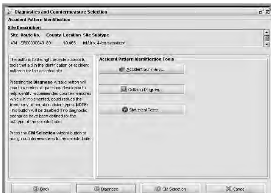
Figure 13. Module 2—Input Screen to Select Diagnostic Tools for Identifying Accident Patterns of Interest
