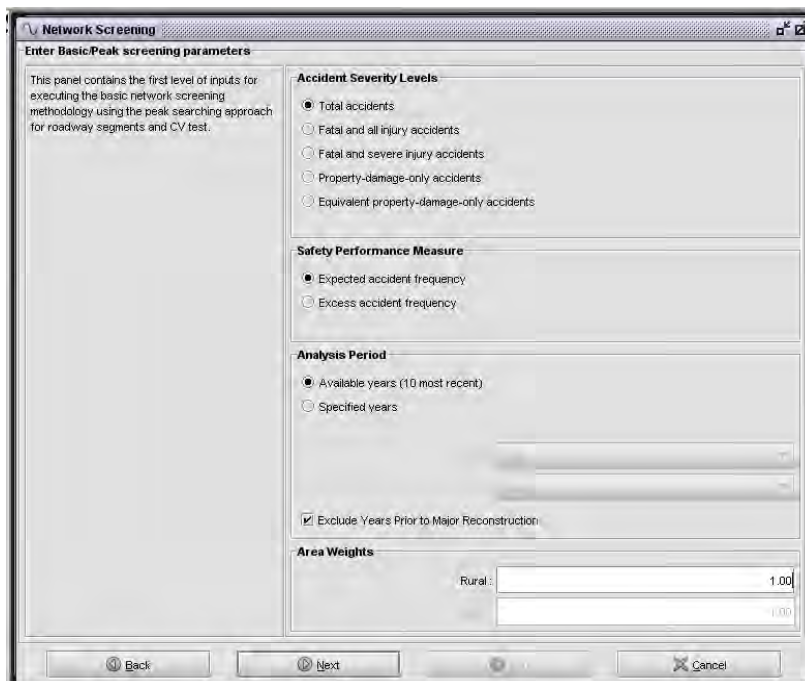
Figure 1. Module 1—Typical Input Screen With Several Common Input Parameters for Network Screening
