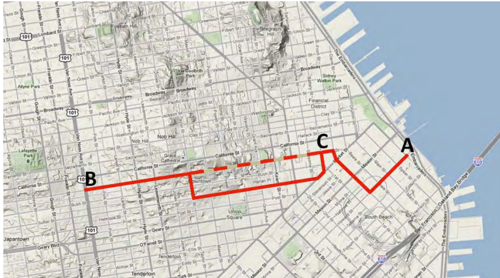
Figure 5.7. Commute from point A to point B: two drivers depart from point A at 8:50 pm on February 1 st with a budget of 20 minutes to reach point B. They are routed by the SOTA module. Because their realized travel times differ, their recommended routes differ. The first driver is suggested to turn left at point C, whereas the second driver is suggested to drive straight.
