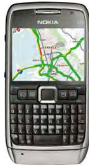
Figure 2.6. The Mobile Millennium phone client running on a Nokia E71. The phone client displays a color map of current traffic conditions around the driver’s location while simultaneously providing VTL data to a central server.
