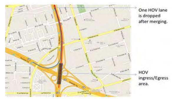
Figure 73. The HOV direct connector and HOV lane stripping at SR-57/SR-91 interchange Caltrans proposed the following re-stripe guideline, which is graphically explained in Figure 75:
