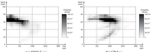
(a) HOV Lane (b) GP lane Figure D9. Probability density of speed-flow: (a) HOV lane, and (b) GP lane (State Route
