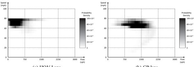
(a) HOV Lane (b) GP lane Figure D6. Probability density of speed-flow: (a) HOV lane, and (b) GP lane (State Route
