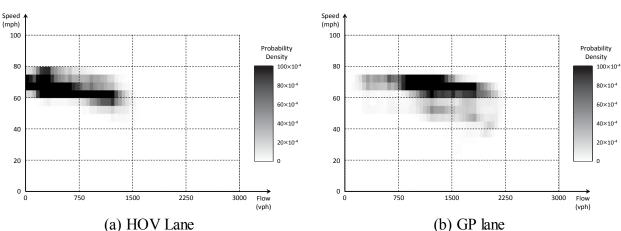
Figure D7. Probability density of speed-flow: (a) HOV lane, and (b) GP lane (State Route
