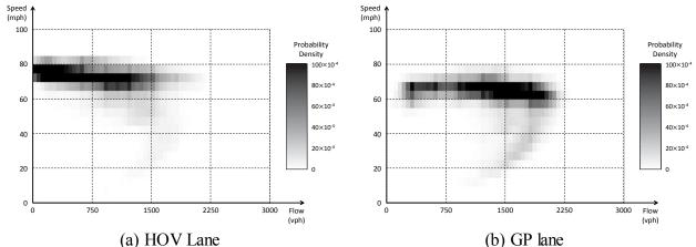
Figure B3. Probability density of speed-flow: (a) HOV lane, and (b) GP lane (Interstate 680
