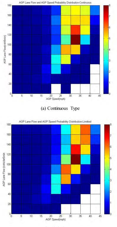
Figure H6. AGP Lane Flow Matrix (a) Continuous, and (b) Limited
