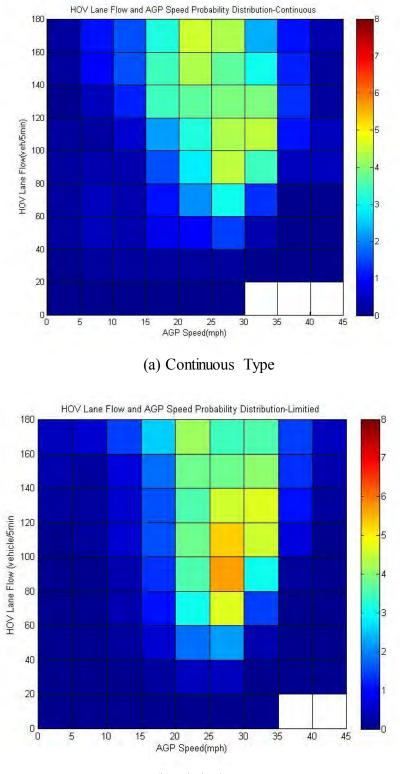
Figure H5. HOV Lane Flow Matrix (a) Continuous, and (b) Limited
