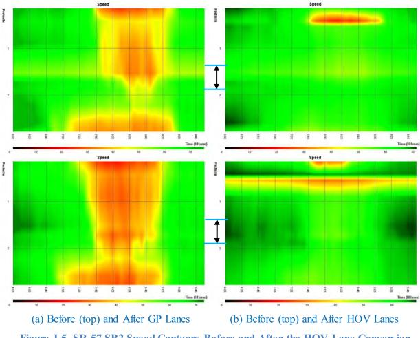
Figure I-5. SR-57 SB2 Speed Contours Before and After the HOV Lane Conversion
