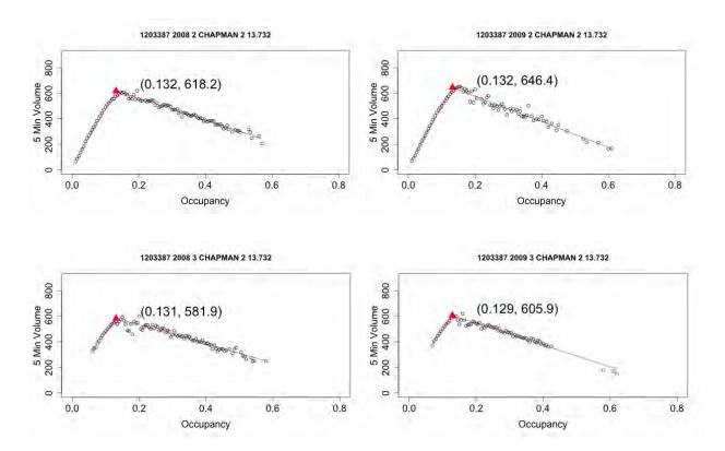
Figure 59. SR-55 SB1: Estimated Traffic Flow Diagram Parameters using Data in Formulation Phase (Top) and Dissipation Phase (Bottom) at Postmile 13.732
