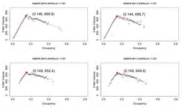
Figure I-8. SR-57 SB2: Estimated Traffic Flow Diagram Parameters using Data in Formulation Phase (Top) and Dissipation Phase (Bottom) at Postmile 1.751
