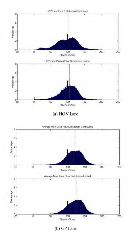
Figure 45. Flow Distribution (a) HOV lane, and (b) GP lane (by Access Type)
