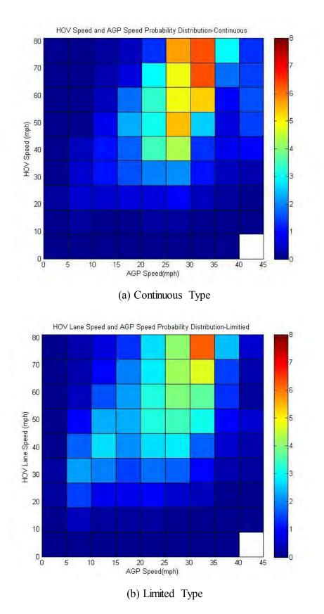
Figure H4. HOV Speed Matrix (a) Continuous, and (b) Limited
