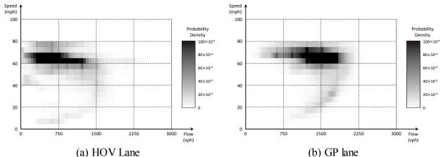
Figure D3. Probability density of speed-flow: (a) HOV lane, and (b) GP lane (Interstate 405
