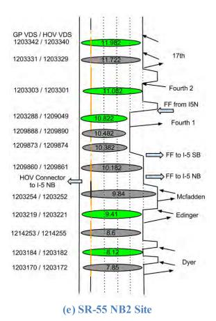
Figure 55. Geometry and Detectors along the Study Sites (Green: Good Detector Data; Grey: Incomplete or Bad Detector Data)
