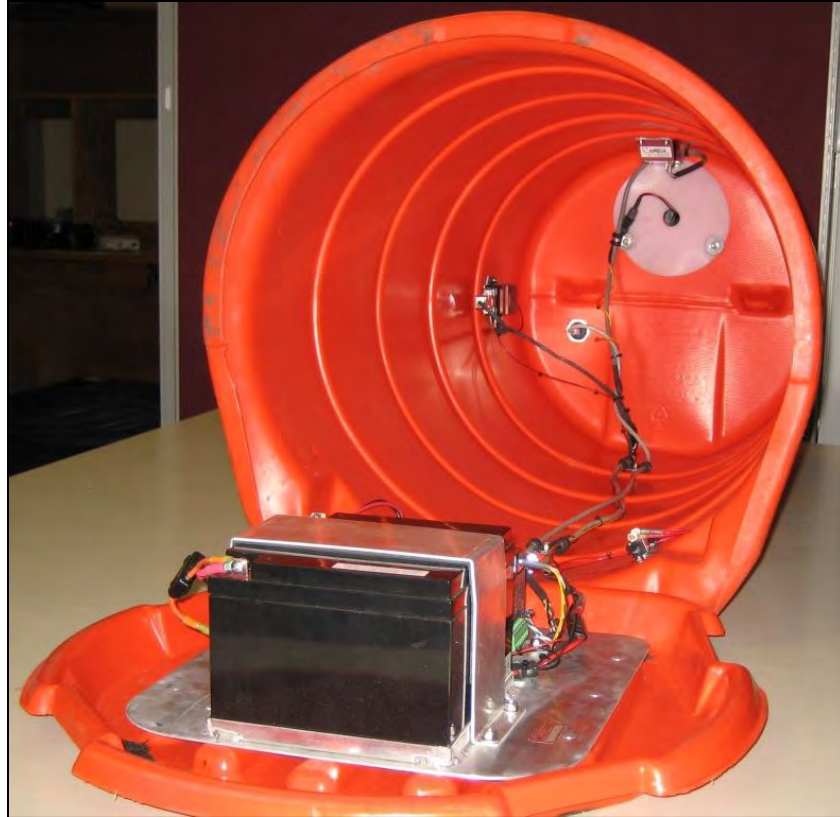
Figure 46: Assembled Master sDrum – WTI Photo
