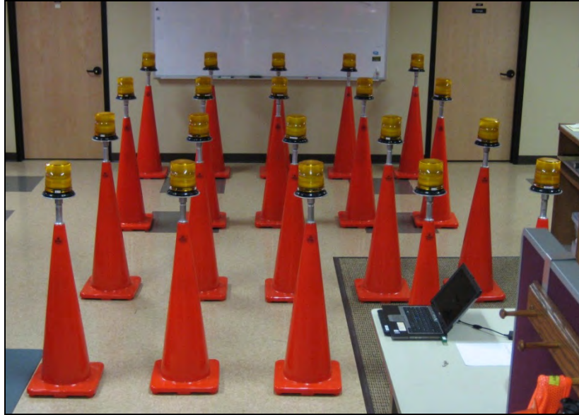
Figure 70: Laboratory Light Pattern Testing - WTI Photo
