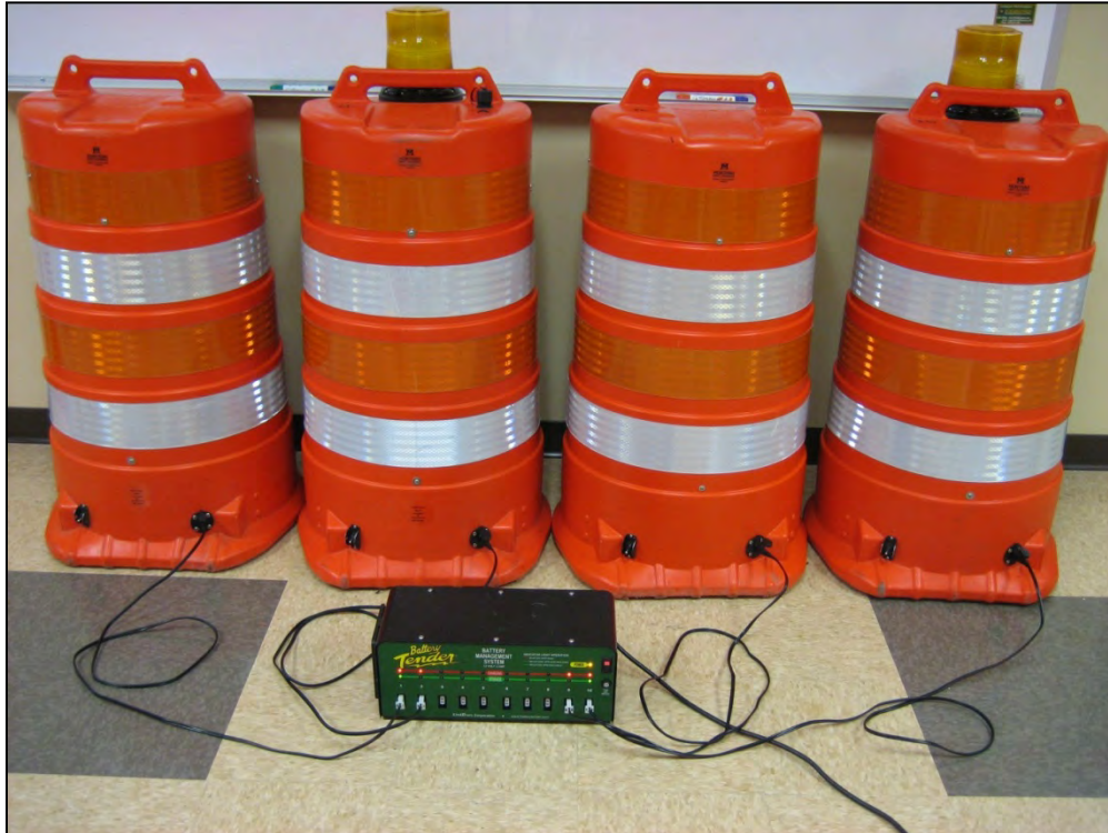
Figure 38: sDrum Charging – WTI Photo
