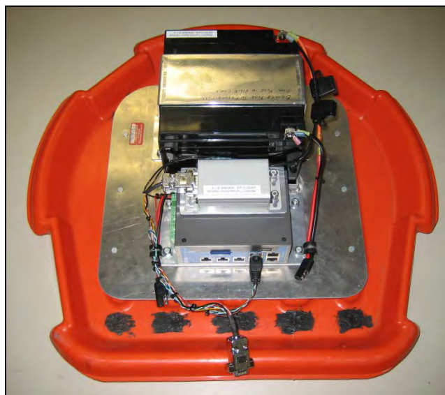
Figure 44: Master/Logger sDrum Base Assembly – WTI Photo
