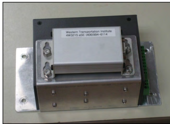
Figure 42: Controller and Light Switch attached to Mounting Bracket – WTI Photo
