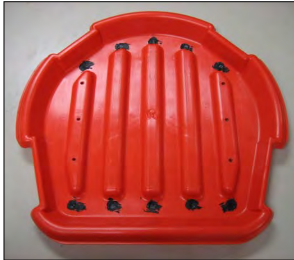
Figure 34: Traffix Standard Drum Base with Tabs Removed - WTI Photo
