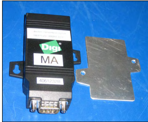
Figure 39: Digi Radio with Mounting Plate – WTI Photo
