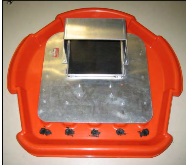
Figure 43: Battery Tray and Strap – WTI Photo
