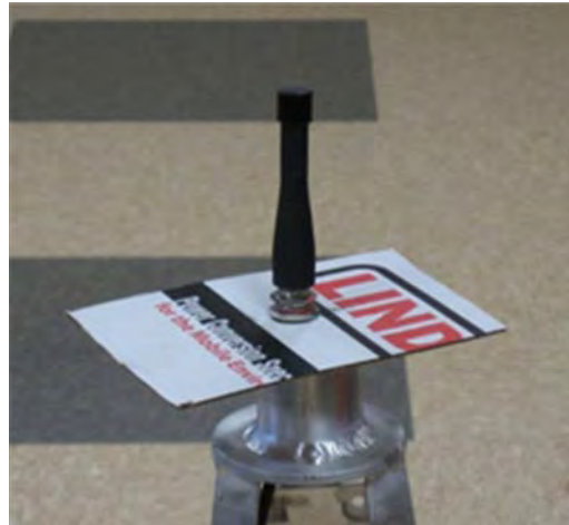
Figure 14: No Ground Plane – WTI Image
