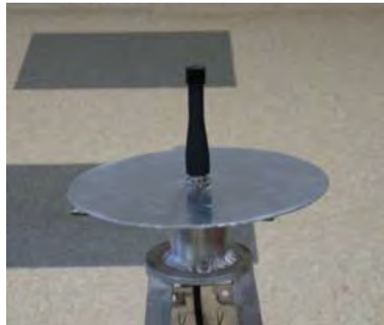
Figure 15: Small Ground Plane – WTI Image
