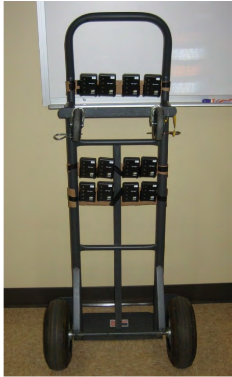
Figure 13: Pager Range Test Fixture - WTI Photo
