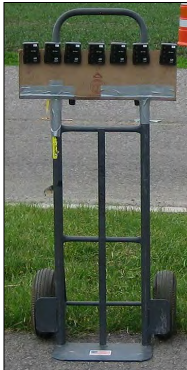
Figure 17: Tuned Pager Range Test Fixture – WTI Image
