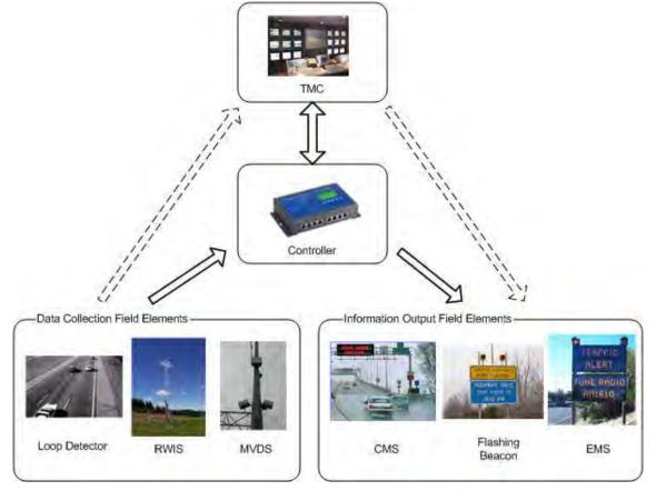
Figure 1: Controller Interaction with TMC and Field Elements
