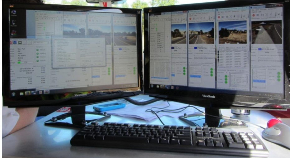
Figure A.3. MX8 user interface (dual monitors, keyboard, and trackball) mounted next to the driver
