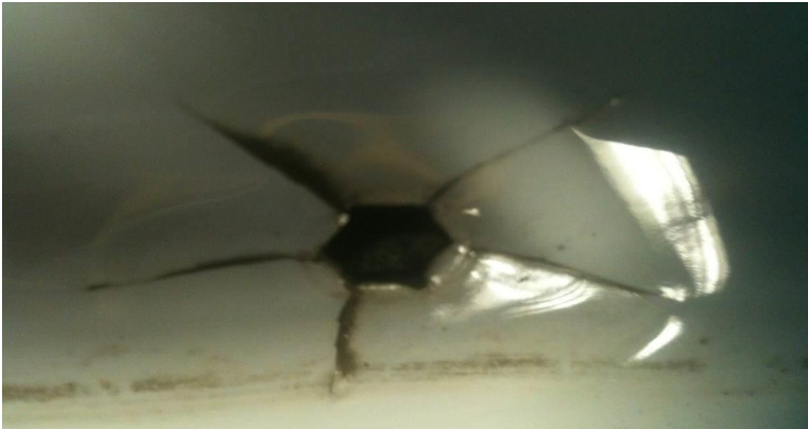
Figure 2.7. Cracks developed at the front roof rack mounts
