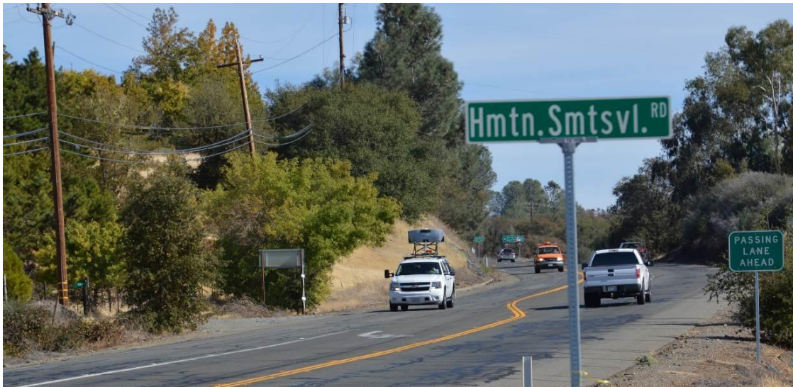
Figure 5.6. MTLS scanning supported by a chase vehicle
