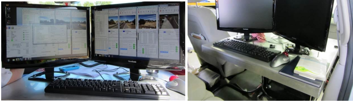
Figure 2.3. MX8 user interface (dual monitors, keyboard, and trackball) mounted next to the driver
