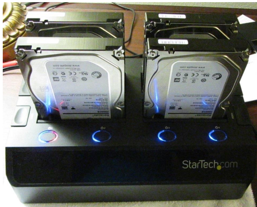
Figure A.38. Data transfer using USB3 4 bay drive dock.
