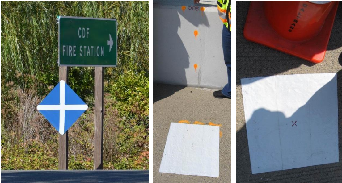
Figure 5.9. “Cross” target on the left and reflective temporary striping tape square target on the right
