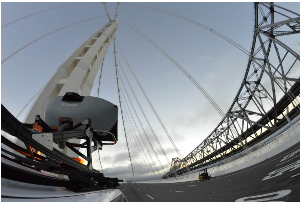
Figure 4.6. Caltrans MTLs system vehicle scanning on the new San Francisco-Oakland Bay Bridge before the bridge opening
