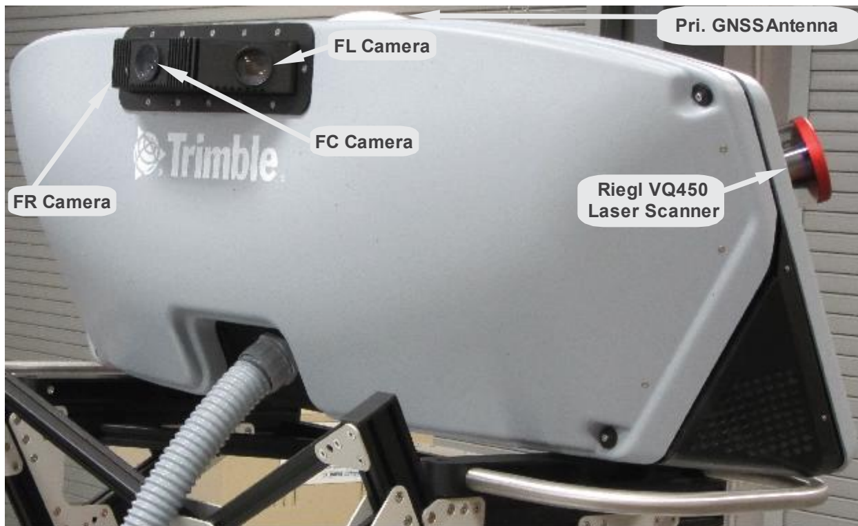
Figure A.2. Caltrans Trimble MX8 MTLs system sensor pod (front view)
