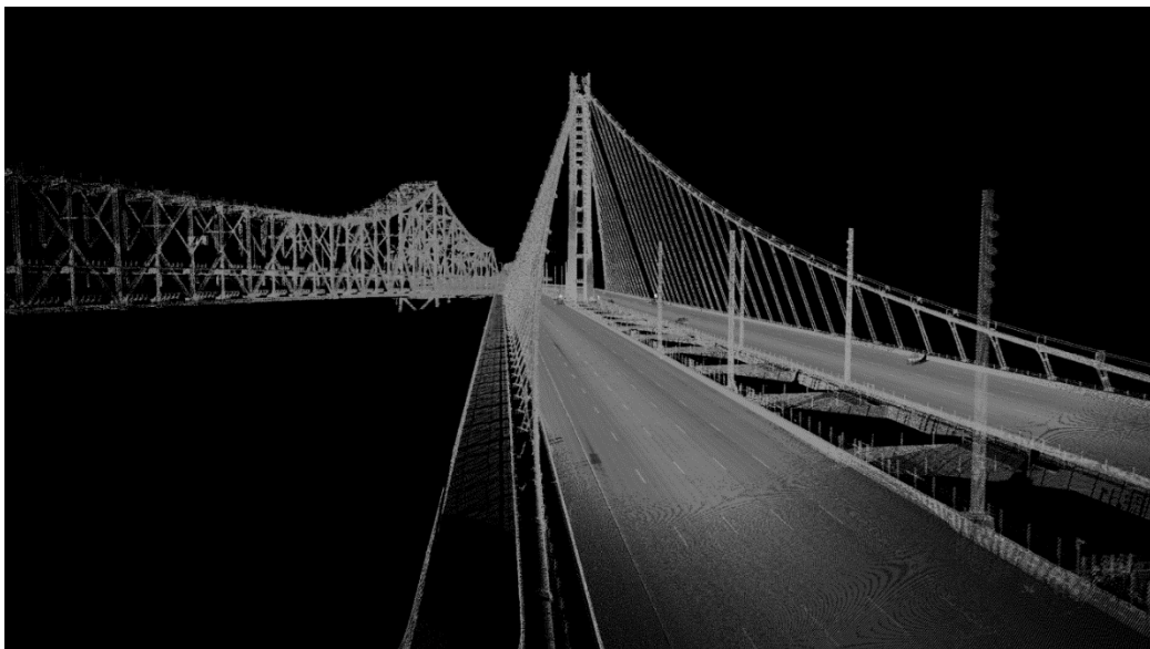
Figure 4.9. Point cloud of the new San Francisco-Oakland Bay Bridge MTLS project
