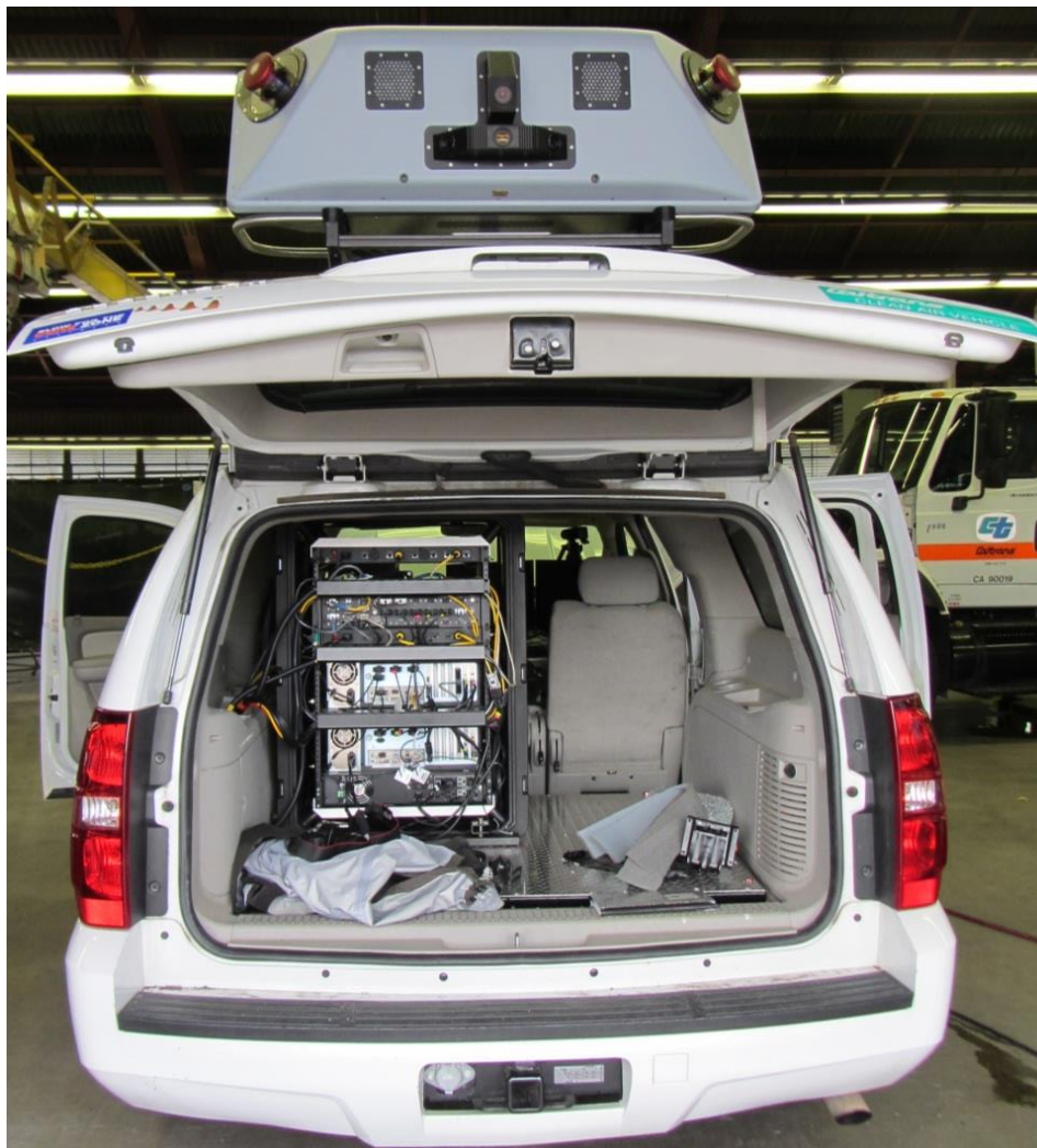
Figure 2.4. MX8 computer rack mounted at the vehicle rear
