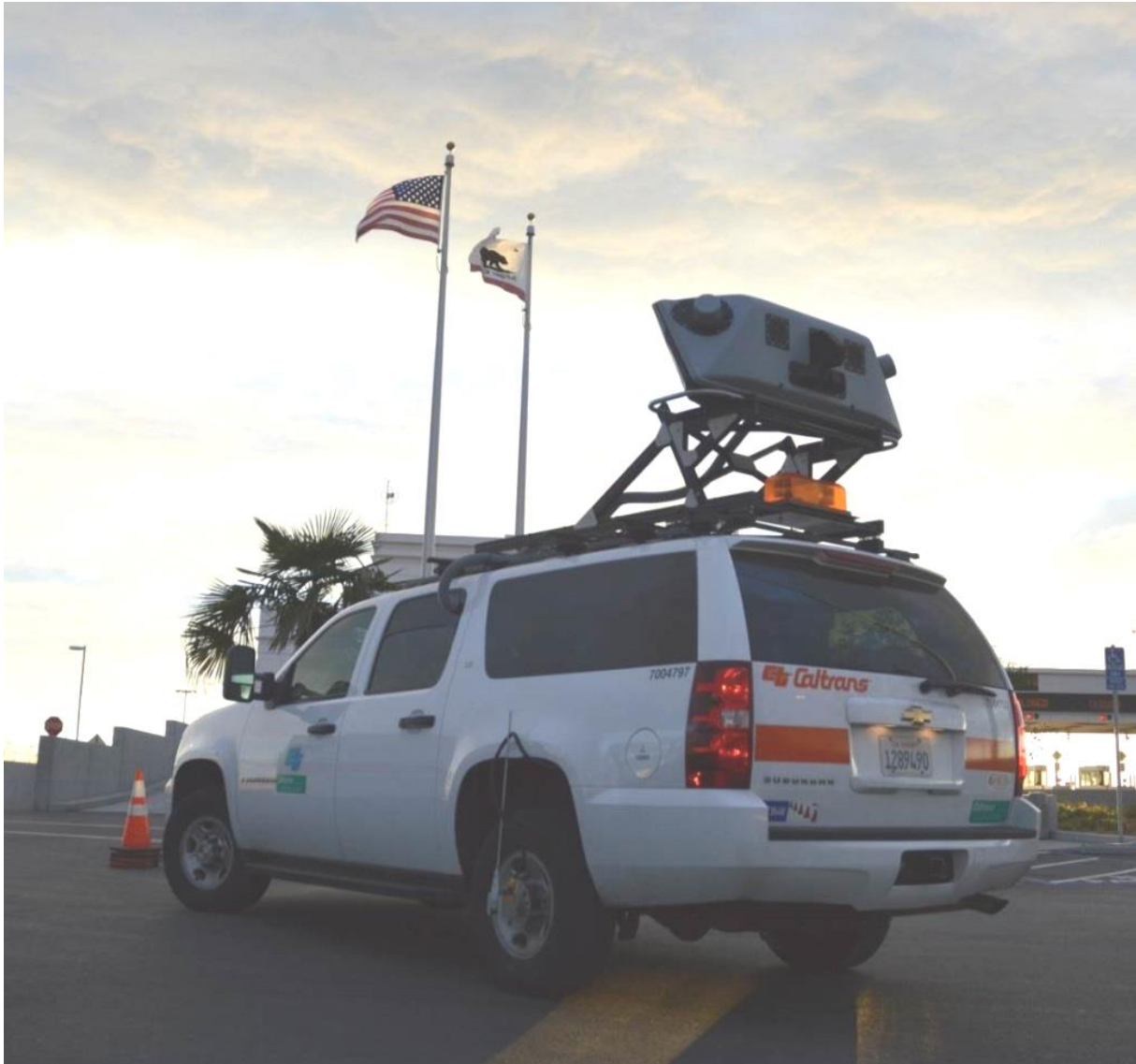
Figure 1.1. Caltrans Trimble MX8 MTLs vehicle at San Francisco-Oakland Bay Bridge Toll Plaza.
