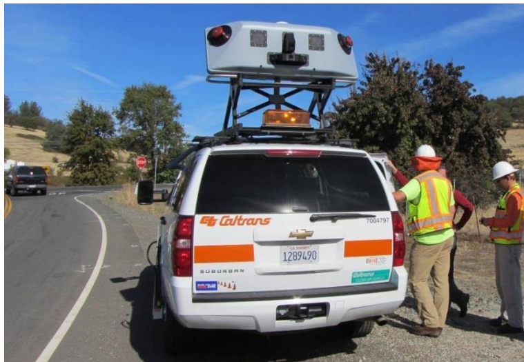
Figure 3.1. MTLS field data collection training at HWY20 Yuba County, CA. (Performing 5-minute static GNSS/IMU data collection at the end of the project data collection)
