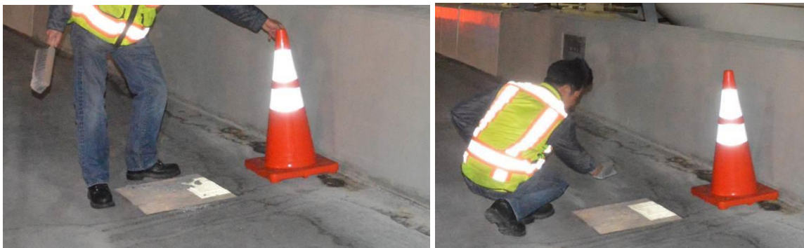
Figure 5.12. Dust and dirt accumulate on the square reflective tape target (on the left) and sweeping off dirt off target (on the right) before scanning
