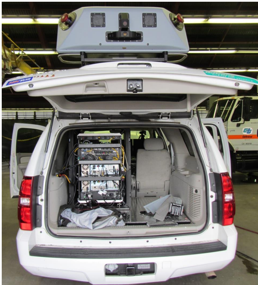
Figure A.4. MX8 computer rack mounted in the vehicle rear
