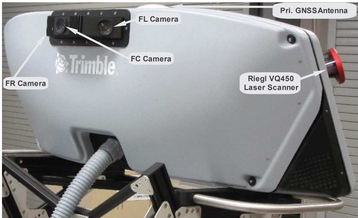
Figure 2.2. Caltrans Trimble MX8 MTLS system sensor pod (front view)
