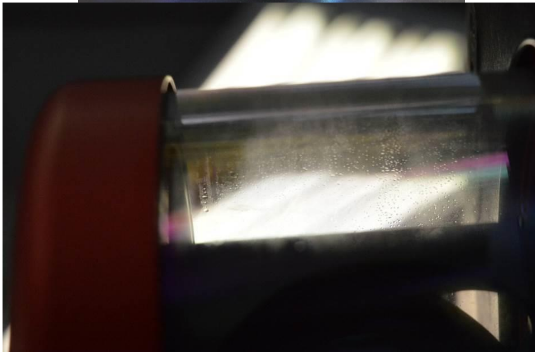
Figure 2.9. Liquid droplet found inside the laser scanner head
