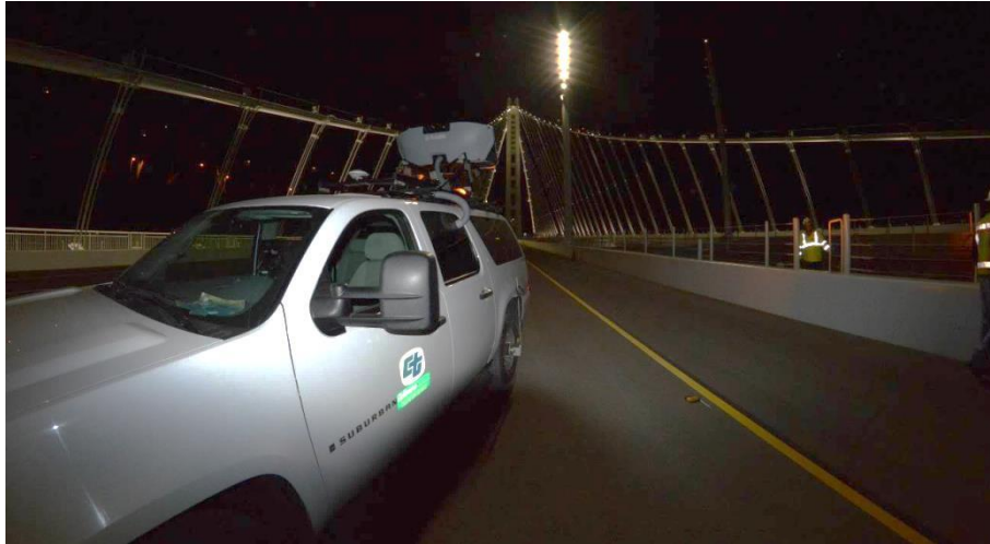
Figure 4.7. Caltrans MTLS system vehicle on the new San Francisco-Oakland Bay Bridge during night time scanning before the bridge opening
