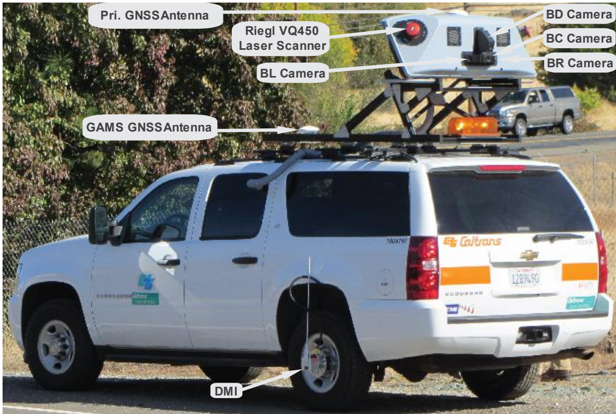
Figure 2.1. Caltrans Trimble MX8 MTLS system sensor pod and DMI
