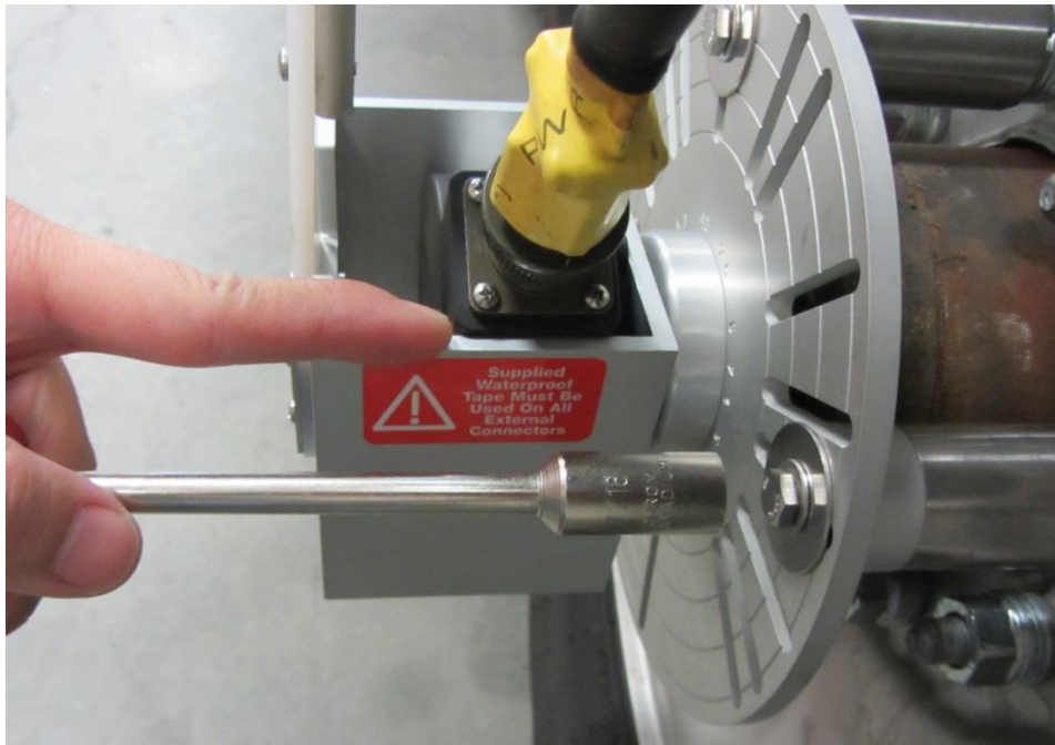
Figure A.40. Removing Applanix DMI adapter plate mounting bolts
