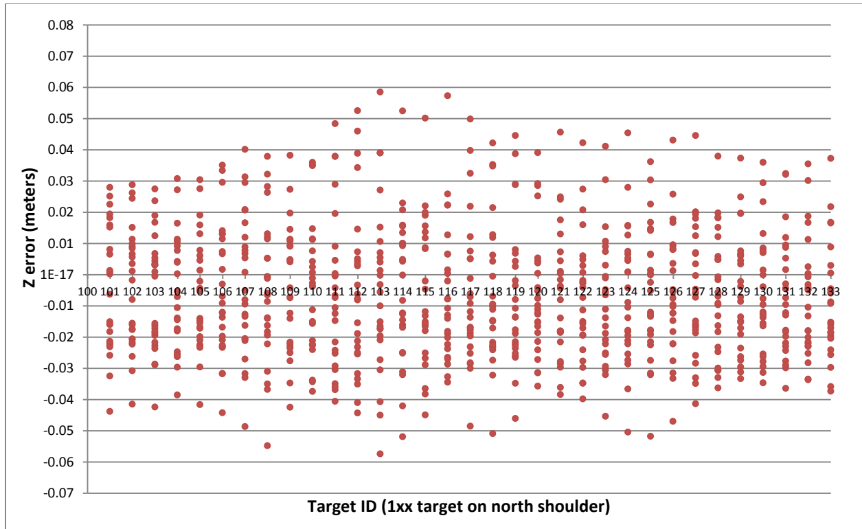
Figure 14. Delta Z error for target ID 1xx on the north shoulder.
