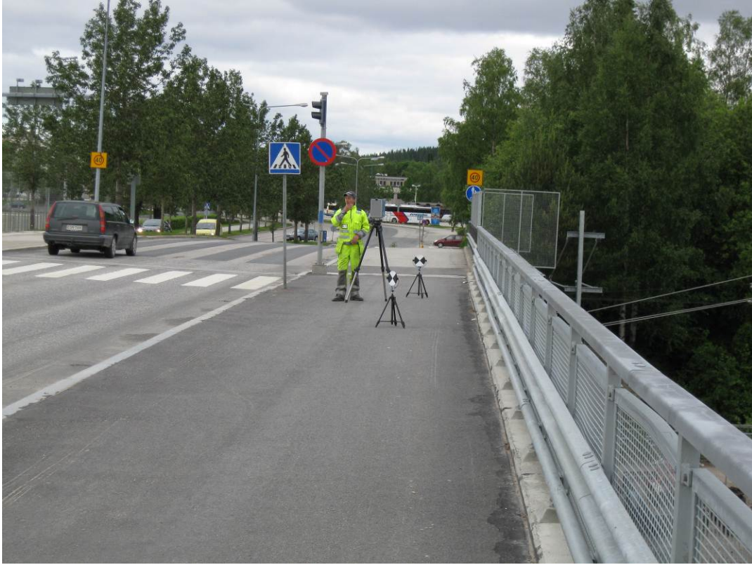
Figure 22: Laser scanning on the bridge deck
