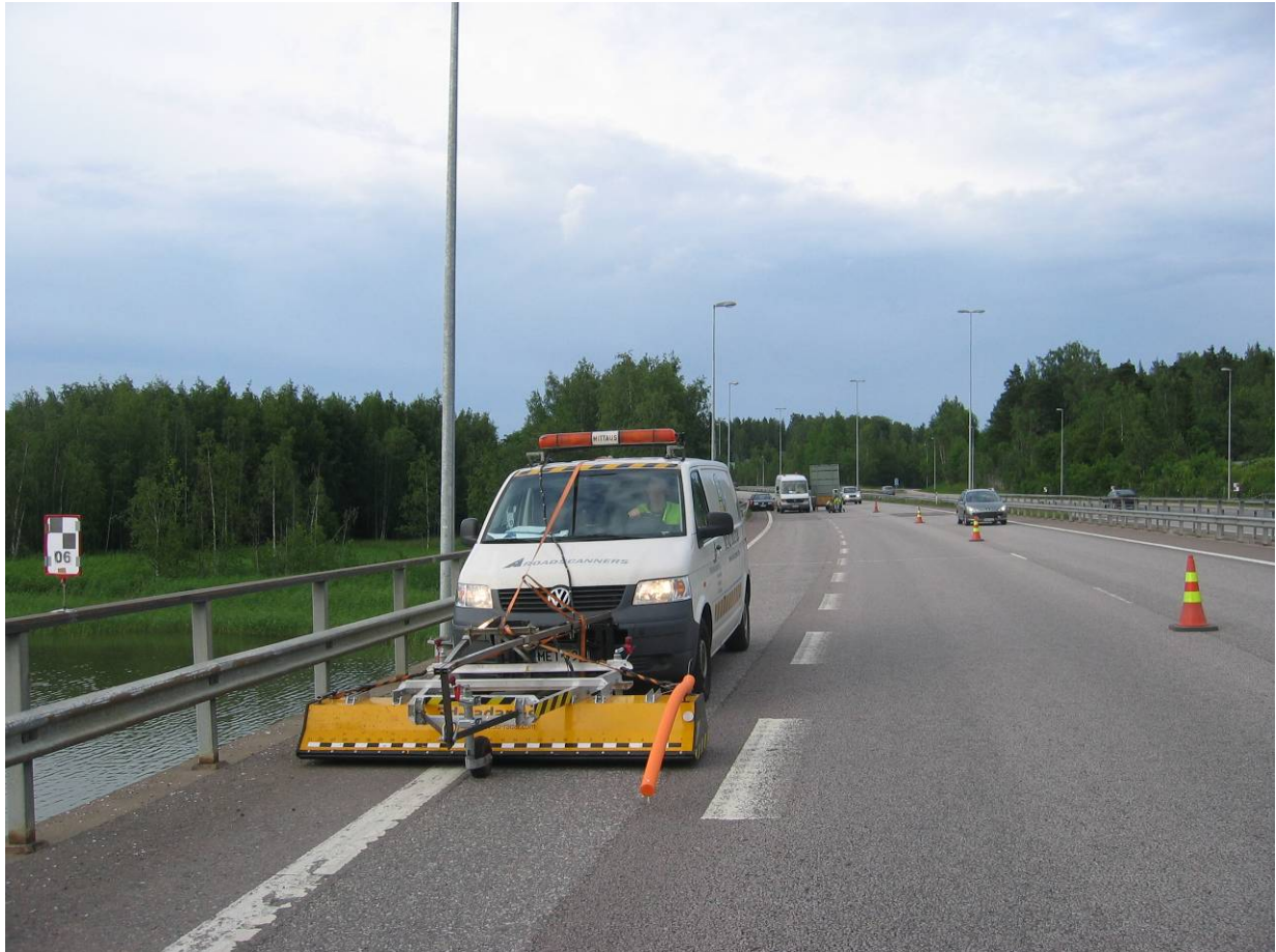
Figure 7: 3D GPR on the Sipoonlahti Bridge, Finland (Courtesy of Roadscanners Oy)
