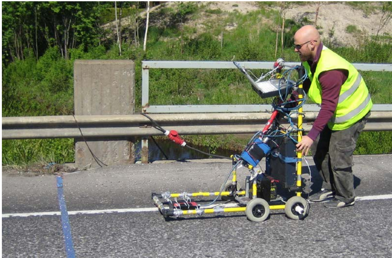
Figure 6: 2D GPR on the Sipoonlahti Bridge, Finland (Courtesy of Roadscanners Oy)
