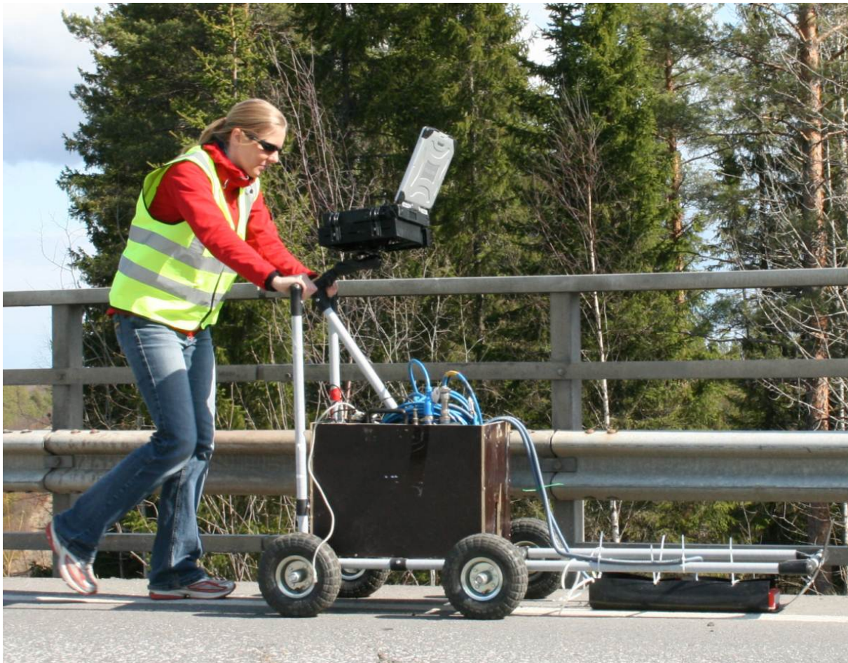
Figure 23: The GPR measurement was made using the GPR system of GSSI (this photo is from a different bridge, Courtesy of Roadscanners Oy)
