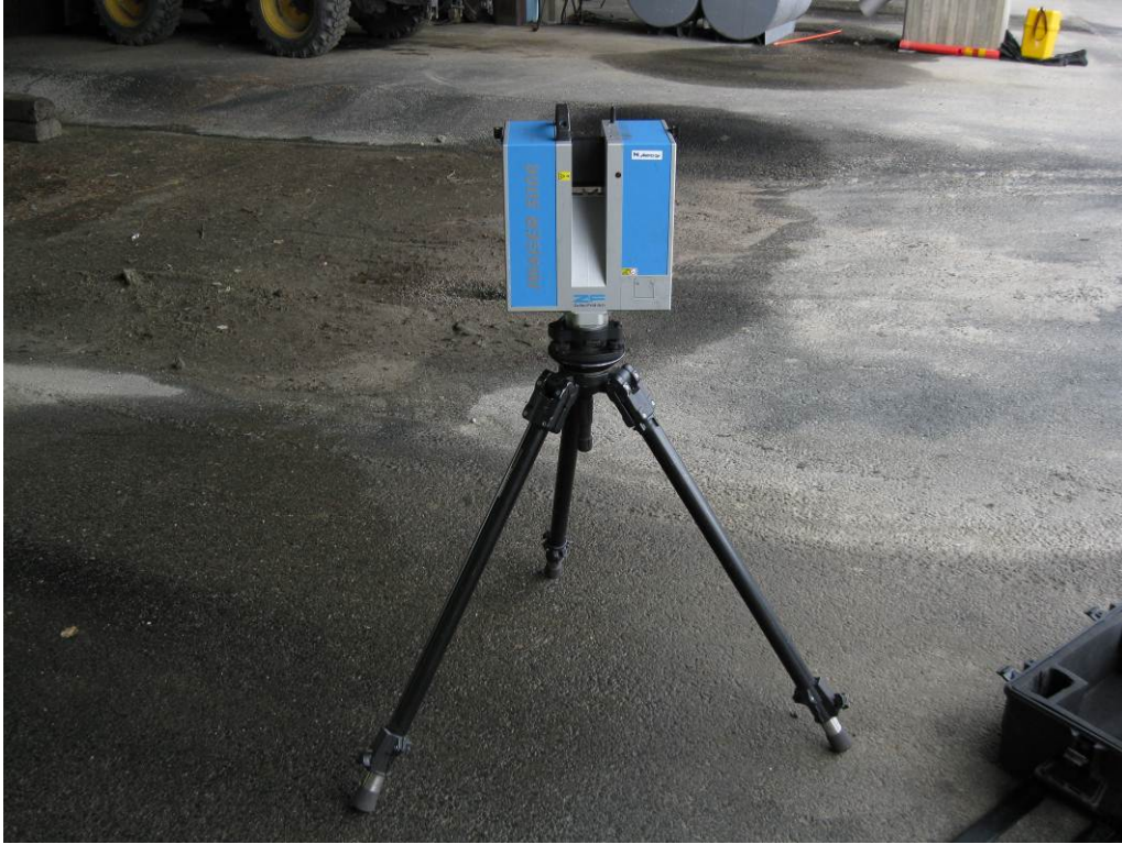
Figure 19: The laser scanning was executed using the Zöller & Fröhlich Imager 5006 system by a measurement consultant (Mitta Oy)
