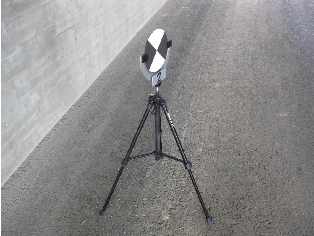
Figure 21: One of the target points of the laser scanning system
