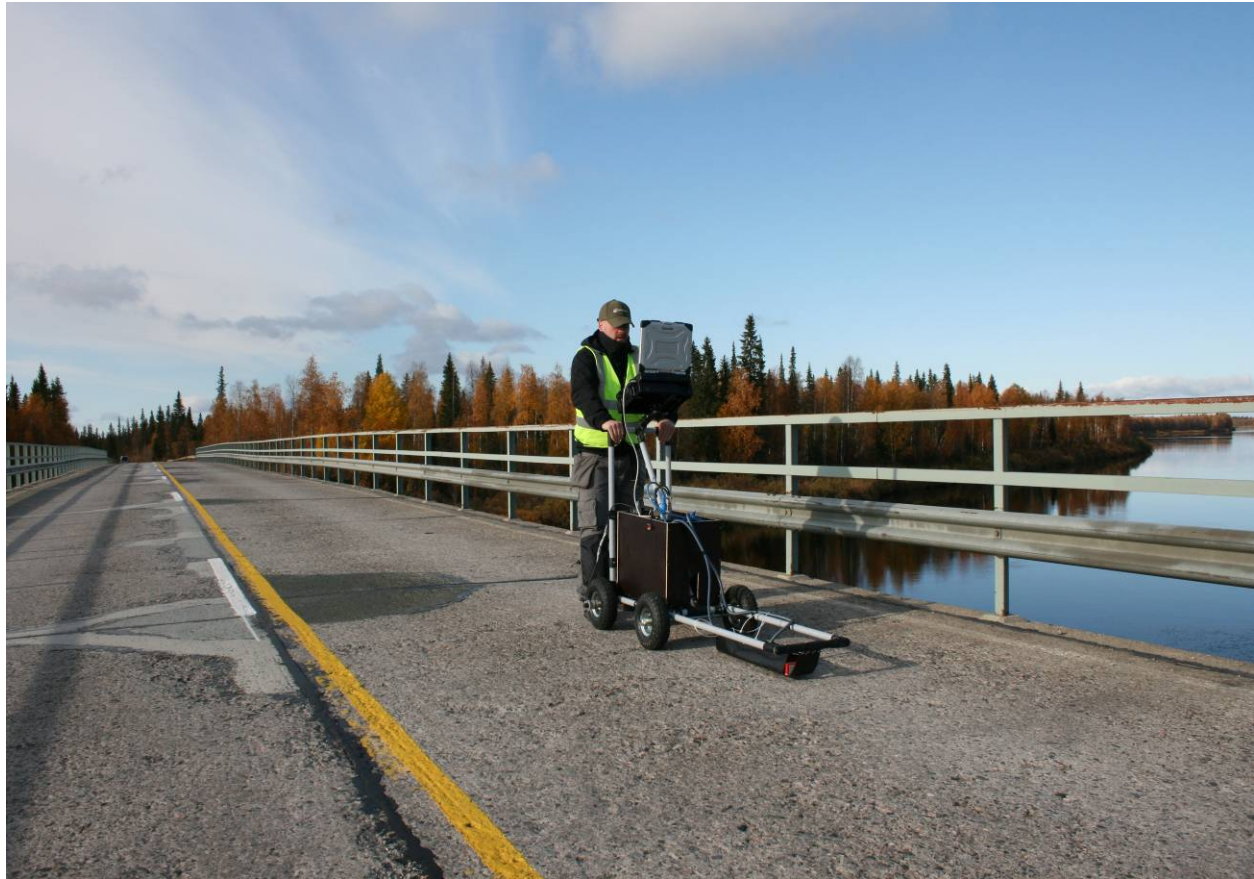
Figure 1: An example of Bridge GPR deck measurement executed in Finland 2008 (courtesy of Roadscanners Oy)
