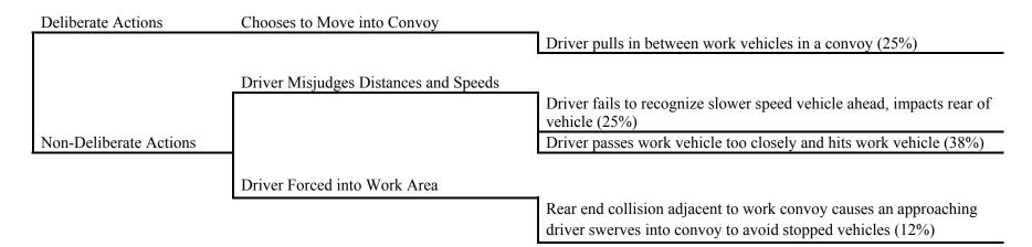
Figure 3. Vehicle Intrusion Crash Sequences: Mobile Operations.
