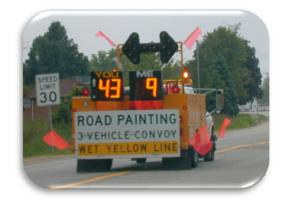
Figure 13. Truck-Mounted DSDs Evaluated in Wisconsin.
