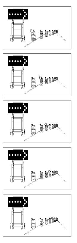
Figure 8. Sequential Warning Light System.
