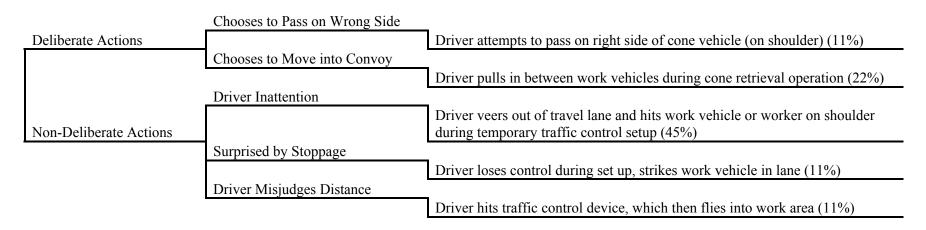
Figure 4. Vehicle Intrusion Crash Sequences: Traffic Control Set-Up and Removal Operations.
