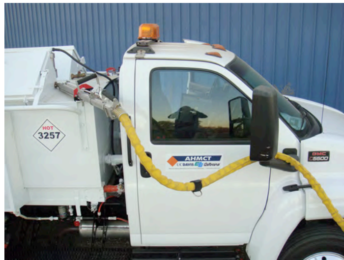
Figure 21. Sealant Hose Recirculation
