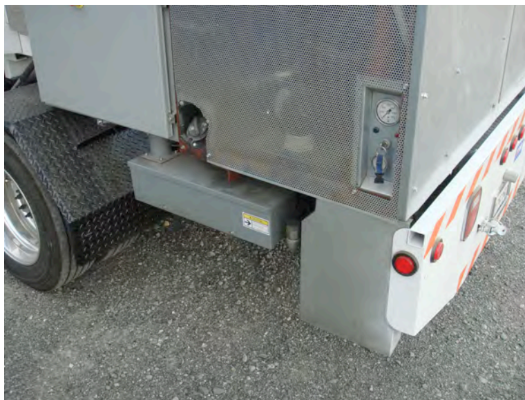
Figure 13. Ignition Switch On Auxiliary Engine
