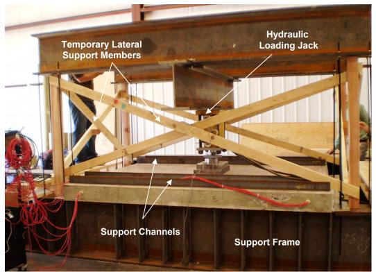
Figure 21: Side view of static load test setup.
