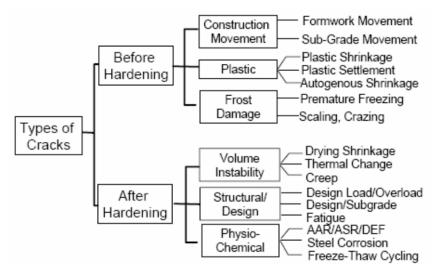
Figure 2: Cracking Mechanisms in Concrete Structures (Transportation Research Circular, 2006)
