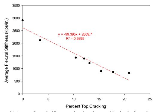
Figure 54: Average flexural stiffness as a function of top cracking for the Control test panels.
