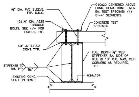
Figure 17: Clamping detail for test specimen.
