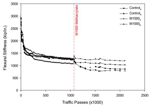
Figure 48: Average flexural stiffness of Panel Set 1.
