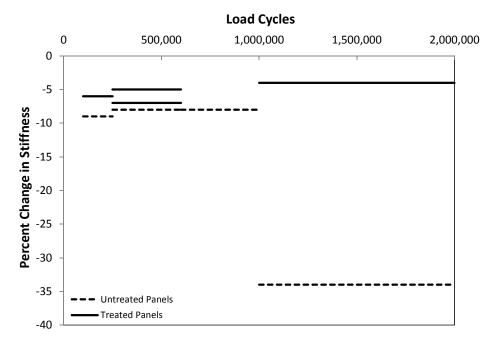
Figure 53: Percent change in stiffness as a function of traffic.
