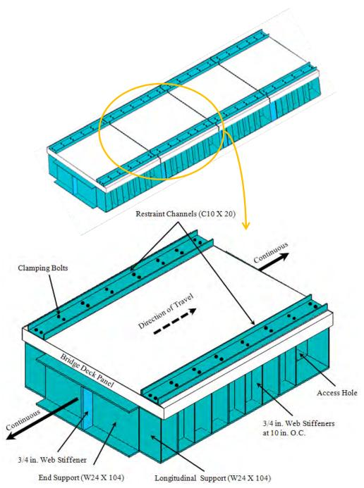
Figure 15: Three-dimensional rendering of support frame.
