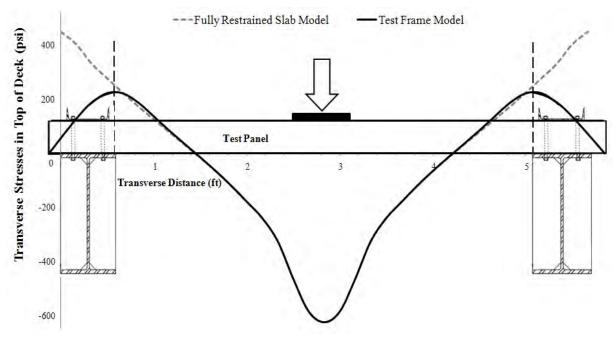
Figure 19: Comparison of transverse stresses in the top of the deck for the fully-restrained slab model and rest frame model.
