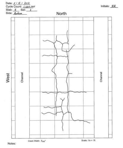
No new crack found in methacrylate overlay Crack widths are withheld due to the effects of shot blasting
