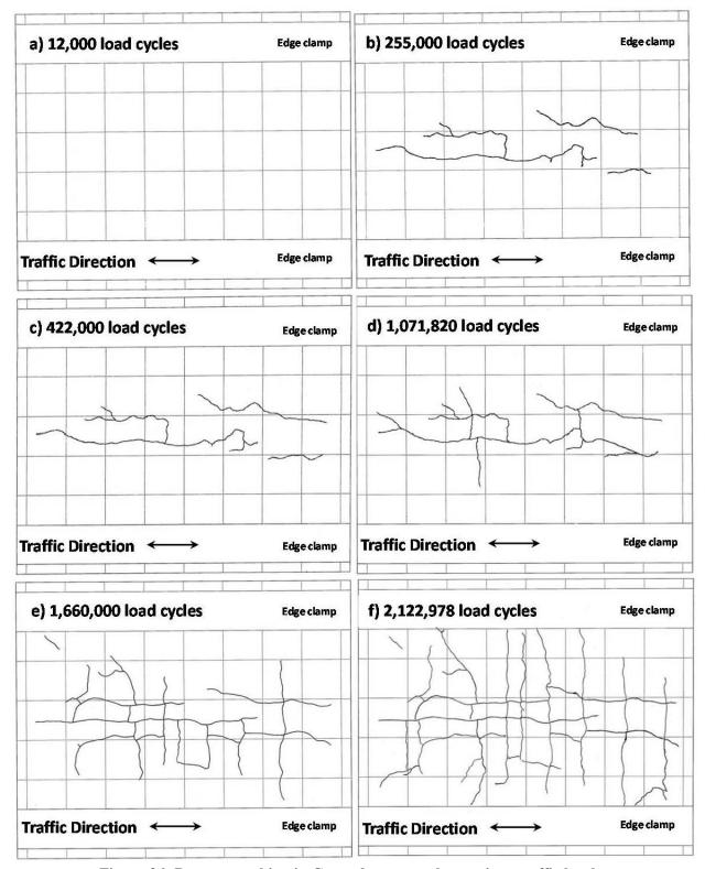
Figure 36: Bottom cracking in Control<sub>a</sub> test panel at various traffic levels.
