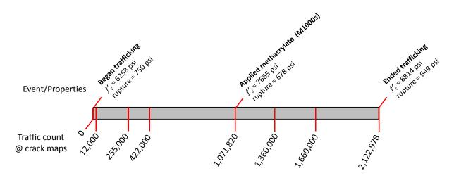
Figure 28: Timeline of events for Control and M1000 test panels (Panel Set 1).
