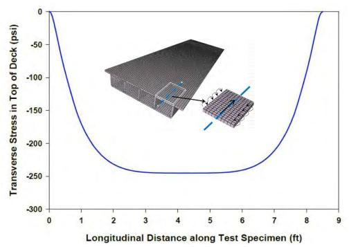
Figure 11: Transverse stresses in the top of the deck under the rolling wheel load as it moves along the specimen.
