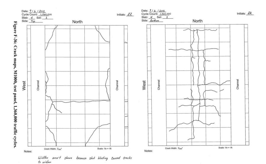
Figure F-37: Crack maps, M1000<sub>b</sub> test panel, 1,660,000 traffic cycles.
