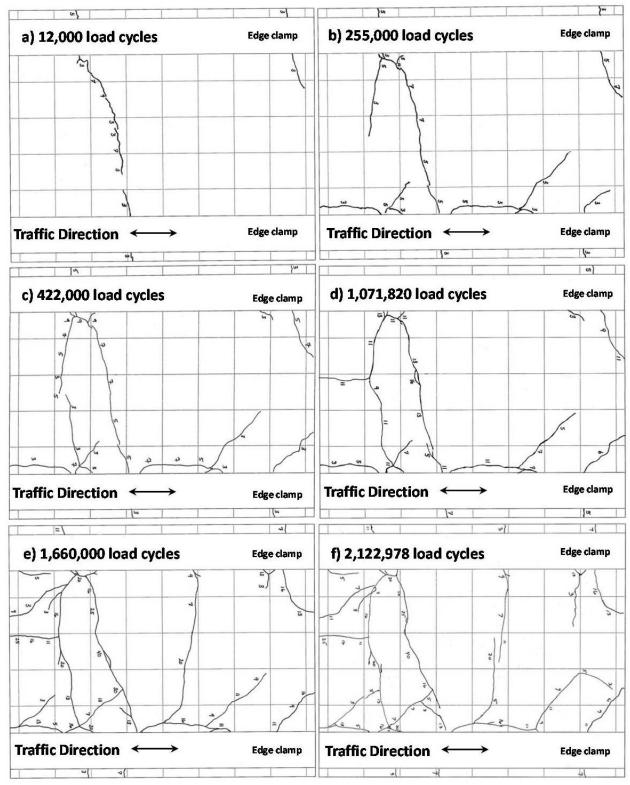
Figure 35: Top cracking in Control<sub>a</sub> test panel at various traffic levels.
