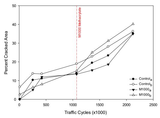
Figure 44: Percent bottom cracking in Panel Set 1.
