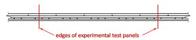
Figure 7: Transverse steel layout in the bridge deck (Section 3 from Figure 6).
