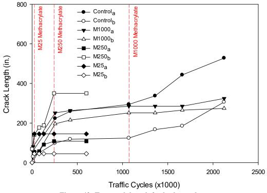
Figure 43: Top crack length for both panel sets.
