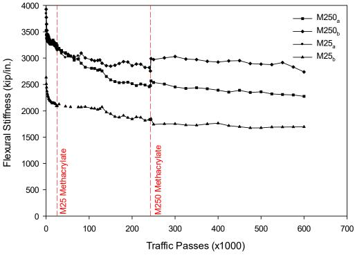
Figure 50: Flexural stiffness of Panel Set 2 based on quarter-point displacements.
