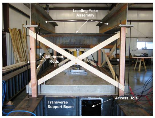
Figure 20: End view of static load test setup.
