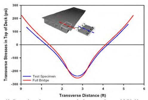
Figure 10: Comparison of transverse stresses in the test specimen and full bridge models.
