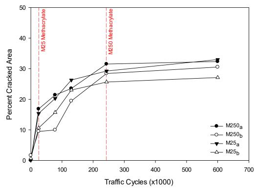
Figure 45: Percent bottom cracking in Panel Set 2.
