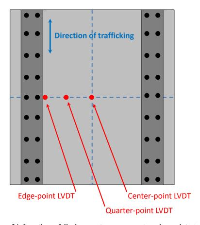
Figure 24: Locations of displacement measurements under each test panel.
