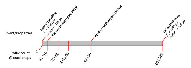
Figure 29: Timeline of events for M250 and M25 test panels (Panel Set 2).
