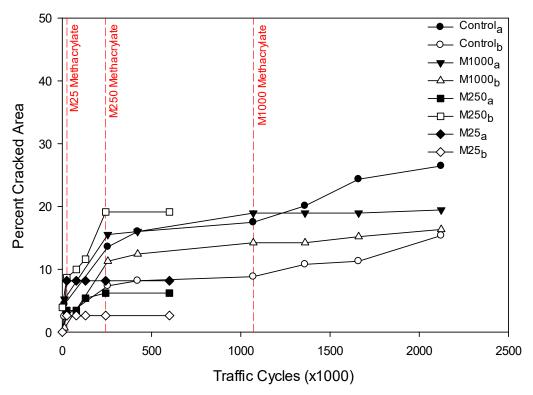
Figure 42: Percent top cracking for both panel sets.
