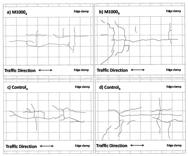
Figure 41: Bottom cracking in M1000 and Control test panels at 1,071,820 traffic passes.
