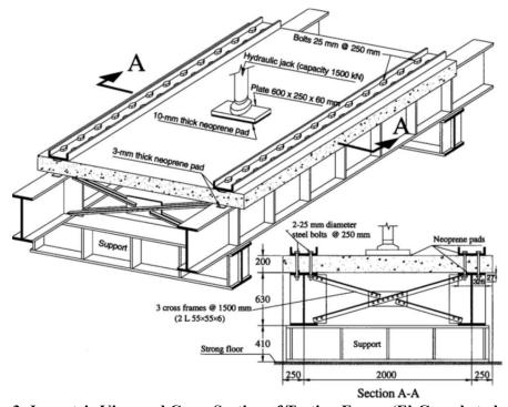
Figure 3: Isometric View and Cross Section of Testing Frame (El-Gamal et al., 2005).
