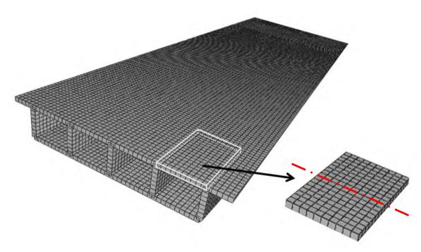
Figure 9: Three-dimensional geometry and VA FEA mesh of the full-scale deck model.
