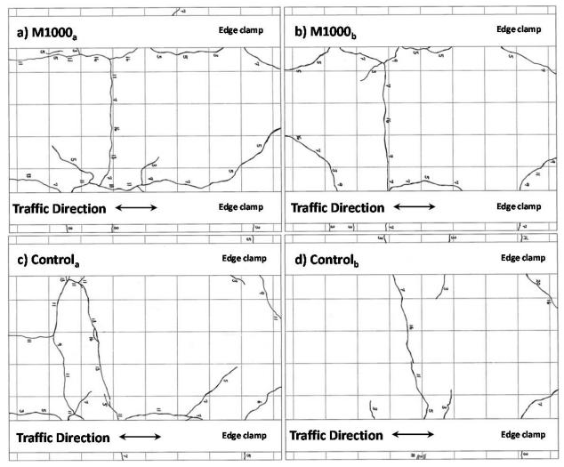
Figure 39: Top cracking in M1000 and Control test panels at 1,071,820 traffic passes.
