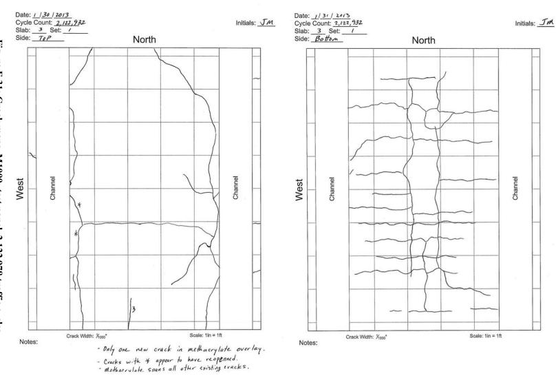
Figure F-31: Crack maps, M1000a test panel, 2,122,978 traffic cycles.
