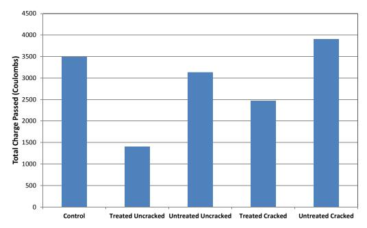
Figure 26: Results from rapid chloride permeability tests on concrete cores.
