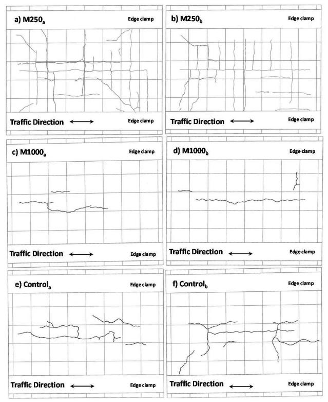
Figure 40: Bottom cracking in M250, M1000 and Control test panels at 250,000 load cycles.
