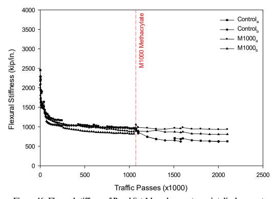
Figure 46: Flexural stiffness of Panel Set 1 based on center-point displacements.
