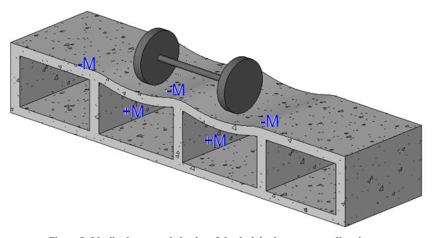
Figure 8: Idealized moment behavior of the deck in the transverse direction.
