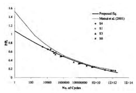
Figure 5: Fatigue life curves for full-scale concrete bridge decks (El-Ragaby et al., 2007).
