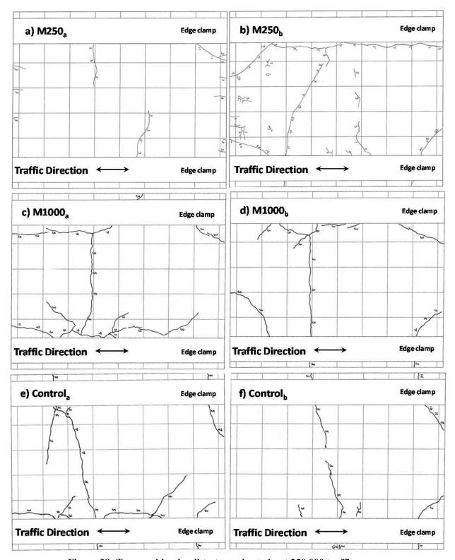
Figure 38: Top cracking in all test panels at about 250,000 traffic passes.
