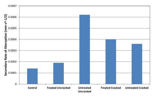
Figure 27: Results from rate of absorption tests on concrete cores.
