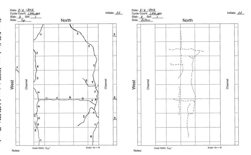
Figure F-28: Crack maps, M1000a test panel, 1,071,820 traffic cycles.
