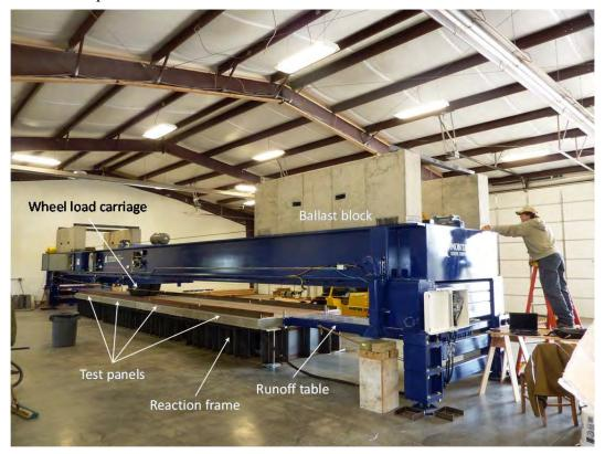
Figure 14: Automated bridge deck tester.
