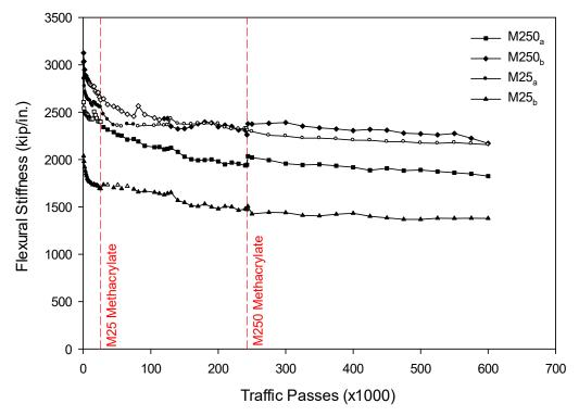
Figure 51: Average flexural stiffness of Panel Set 2.
