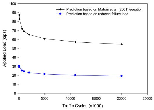
Figure 22: Predicted fatigue life of test panels as a function of applied load.
