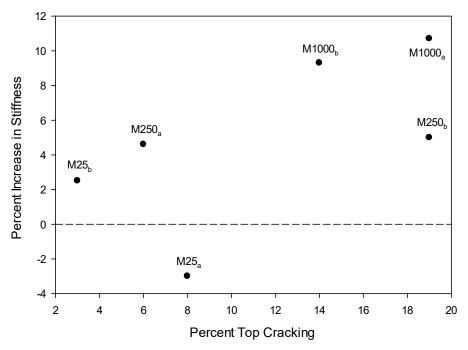
Figure 52: Percent cracking versus percent increase in stiffness.
