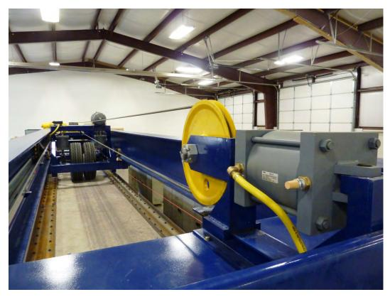
Figure 23: Drive cable and carriage assembly.
