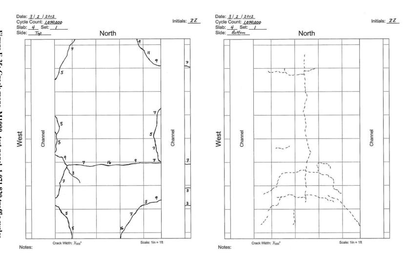
Figure F-35: Crack maps, M1000b test panel, 1,071,820 traffic cycles.
