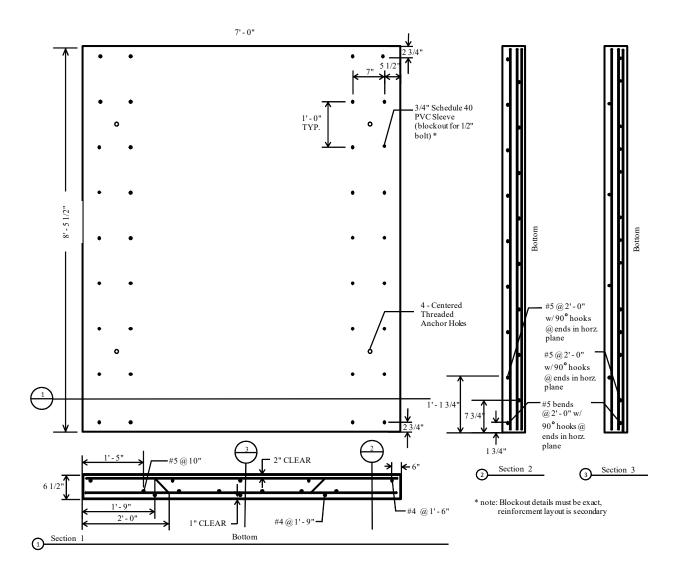
Figure 6: Dimensions and reinforcement details of test specimens.
