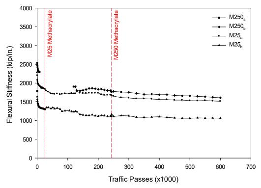
Figure 49: Flexural stiffness of Panel Set 2 based on center-point displacements.
