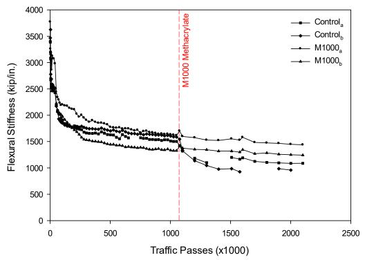
Figure 47: Flexural stiffness of Panel Set 1 based on quarter-point displacements.
