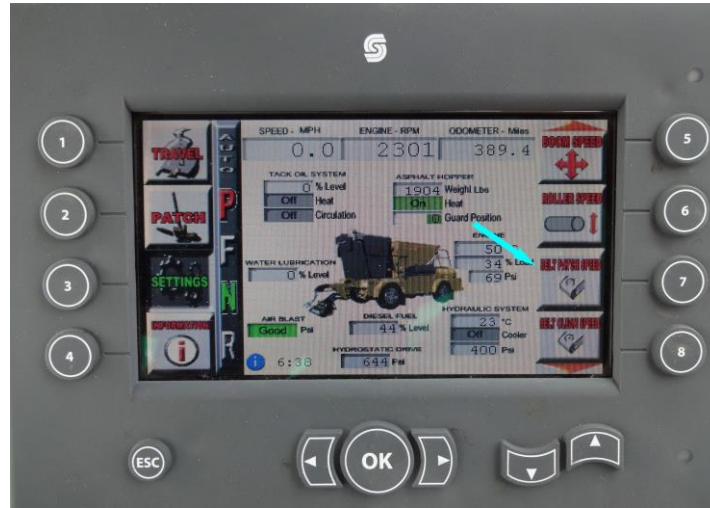
Figure 26. Asphalt Delivery Rate Setting
