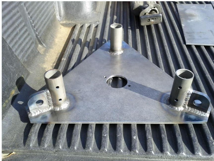
Figure C.2: The assembled tower top plate
