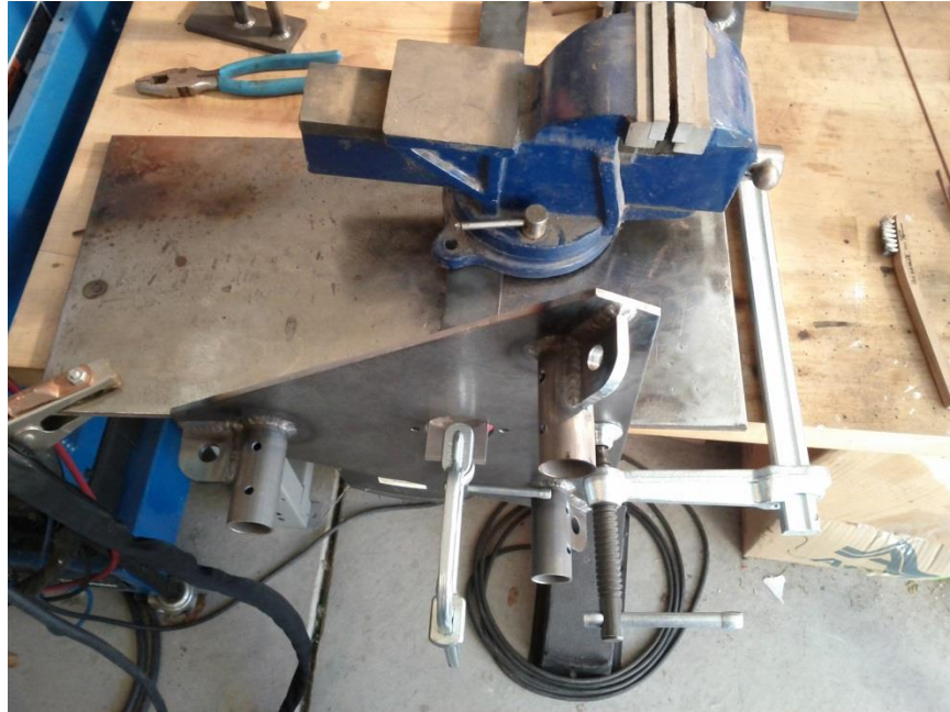
Figure C.1: TIG (tungsten inert gas) welding the tower top plate fabrication
