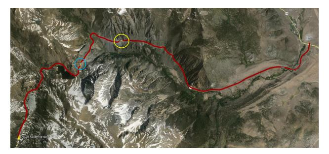
Figure 5.2: Google Earth screen capture with the vehicle path (in red) overlaid on SR 120. The yellow and blue circled areas are locations with very limited GPS availability.
