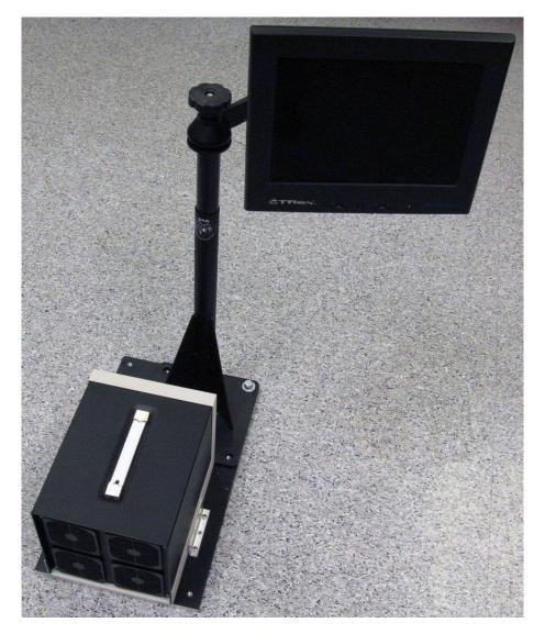
Figure 3.3: Liquid Crystal Display (LCD) and system box containing computer and GPS receivers
