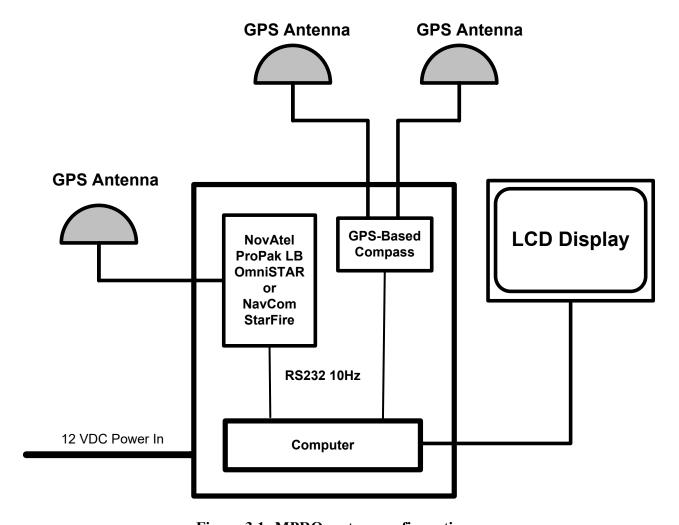
Figure 3.1: MPRO system configuration
