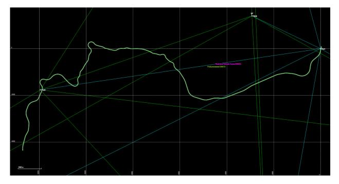
Figure 4.4: Vehicle trajectory resulted from GNSS/IMU post-processing with CORS station P636 base station using POSPac software
