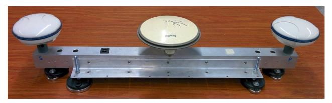
Figure 3.4: GPS antenna bar with magnetic mount
