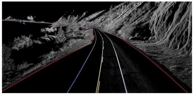
Figure 4.8: Point cloud with extracted feature lines overlaid in Cyclone. The red, blue, and yellow lines denote the edge of pavement, fog line, and centerline, respectively.
