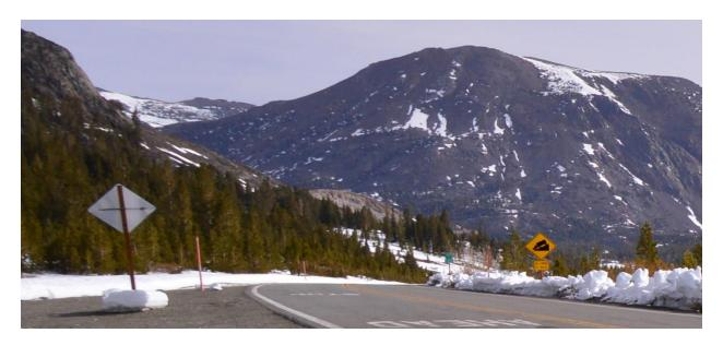
Figure 5.11: Sign and building locations need to be mapped to reduce accidental damage during snow clearing (picture taken 4/21/2014)
