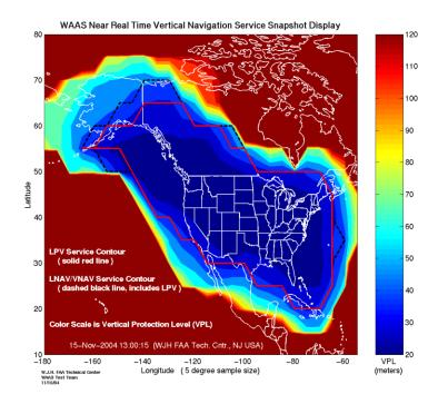
Figure 2.1: WAAS GPS Vertical accuracy map (http://www.nstb.tc.faa.gov/RT VerticalProtectionLevel.htm)
