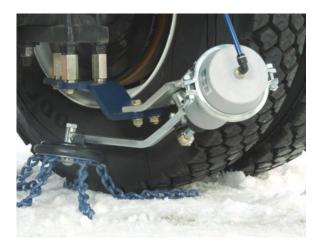
Figure 3. Generalized ATD Installation (Onspot, Similar to Insta-Chain and Roto-Grip)
