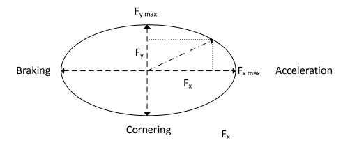
Figure 14. The Tire Friction Ellipse
